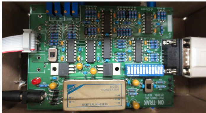
Figure 5.3 OT-301DL amplifier for duolateral PSDs
