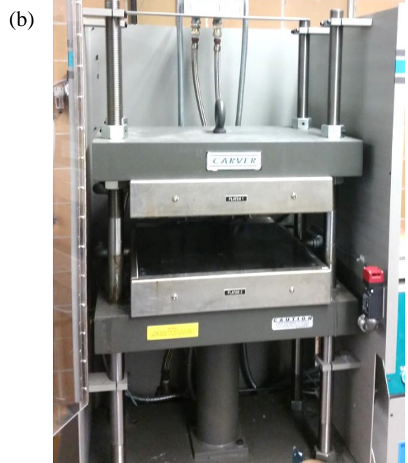
Figure 3-2: a) Hot platen press stacking sequence; b) Carver Inc. self-containing press with heating/cooling platens and programmable controller
