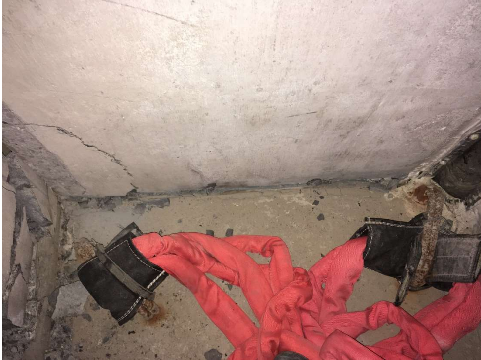
Figure 4-99: Cracking of concrete near the corners on the back of the wall at the end of the collapse test of the CS joint
