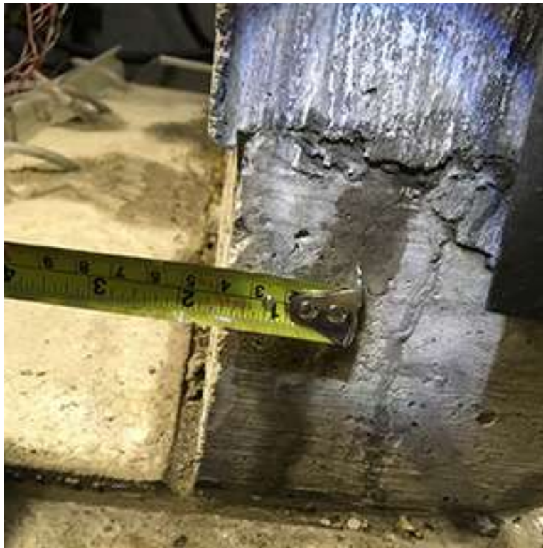
Figure 5-11: Formation of the cracks on the compression side of the upturn part in limit state test of the UF joint
