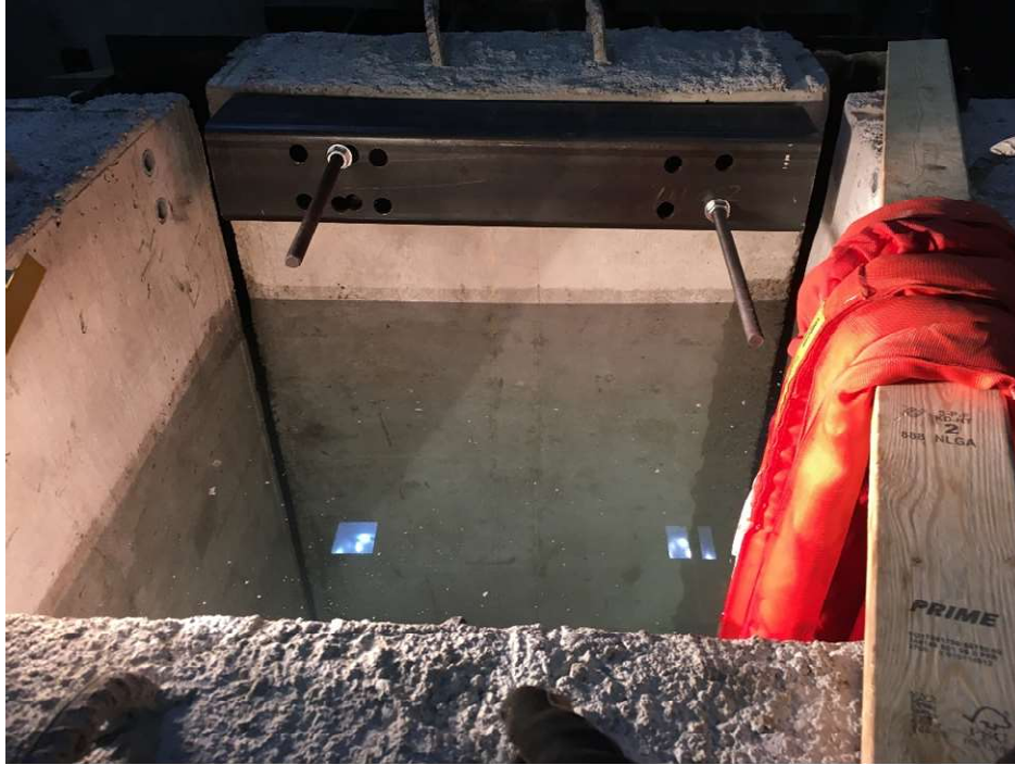
Figure 4-5: HSS beam on the back of the wall
