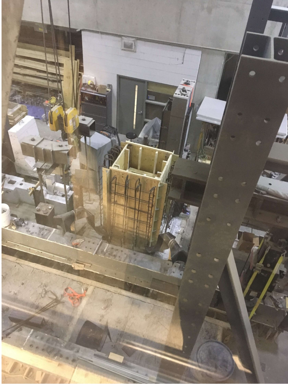
Figure 3-17: The top view of the completed inner formworks and wall reinforcements
