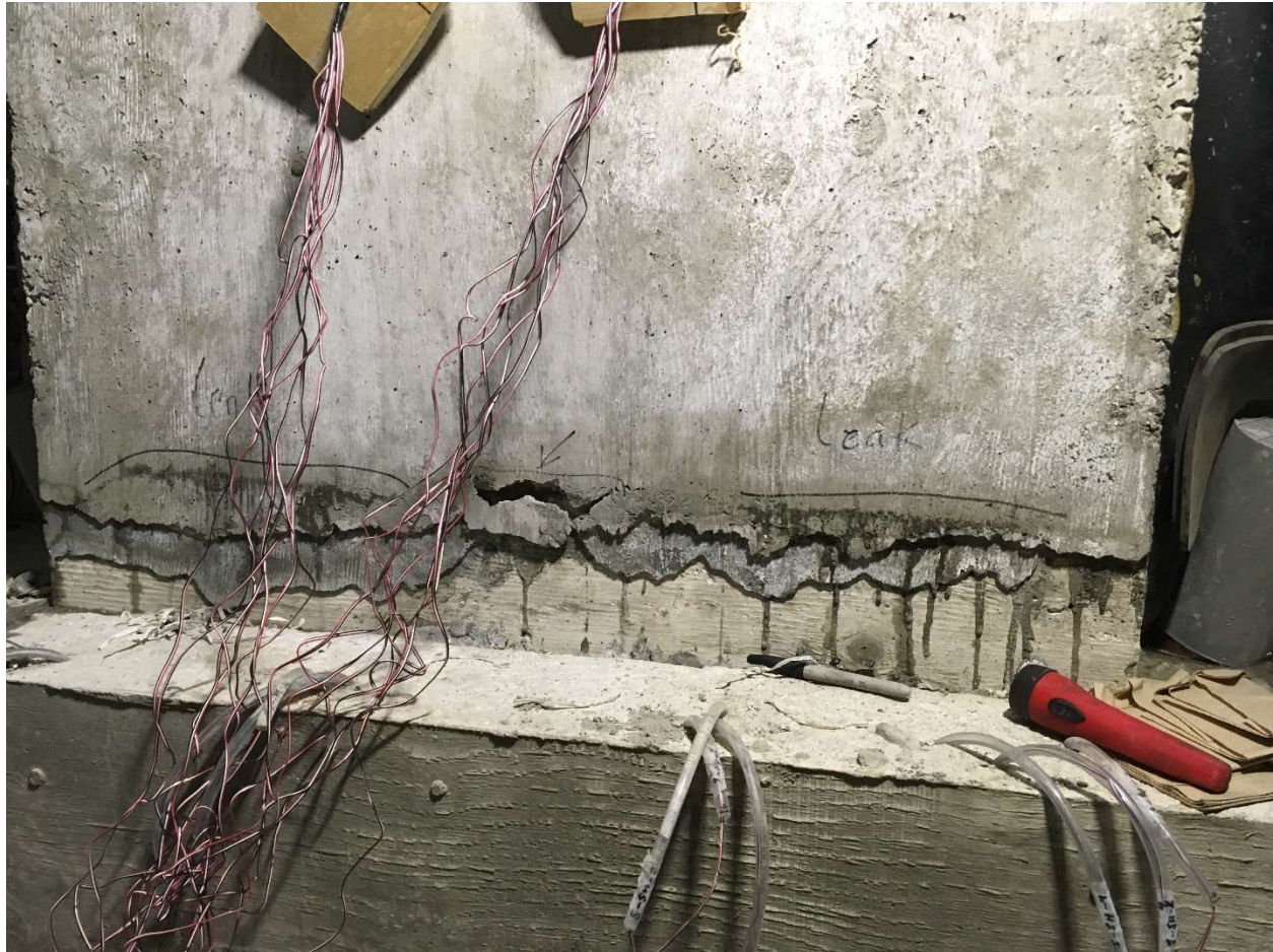
Figure 4-38: Occurrence of leakage at the end of the leakage test of the US joint
