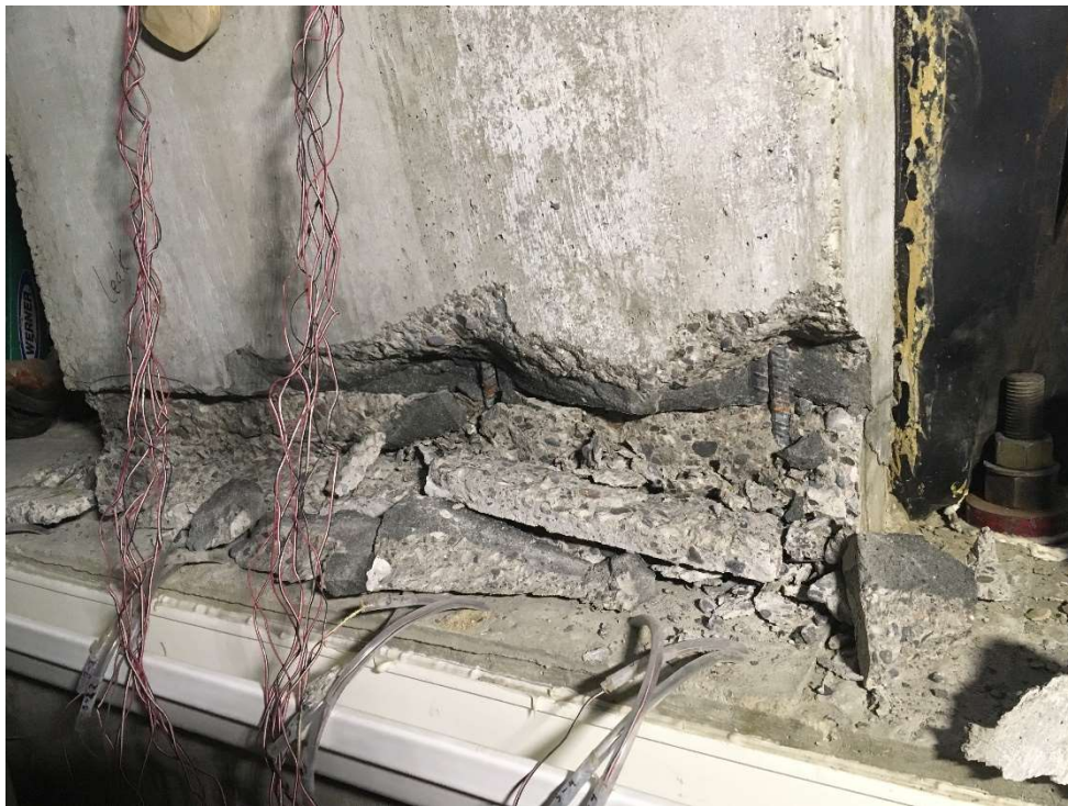
Figure 4-88: Crushing of concrete on the front of the wall at the end of the collapse test of the UF joint
