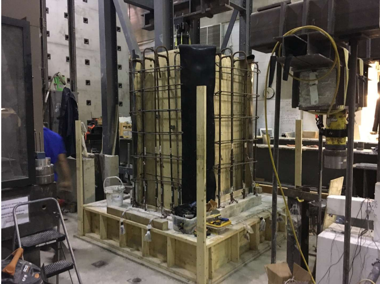
Figure 3-19: A perspective view with the inner formwork completed, reinforcements installed, and the membranes erected and tied to reinforcements
