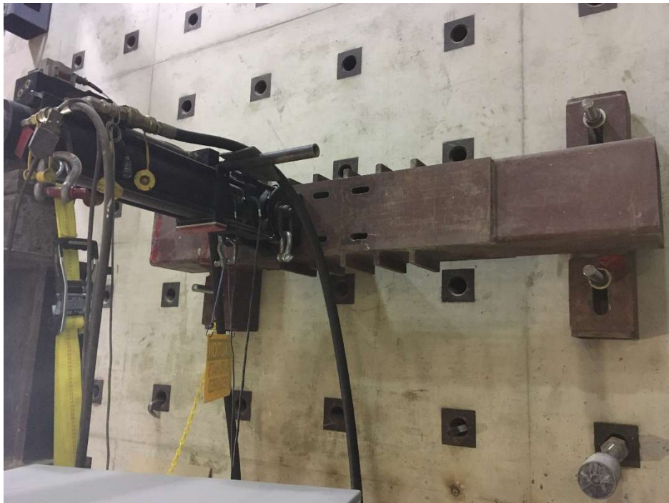
Figure 4-2: Connection of actuator to the supporting bracket
