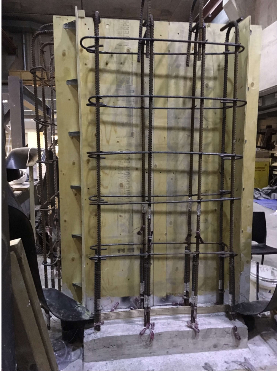
Figure 3-18: The wall reinforcements and the strain gauges for an upturn joint
