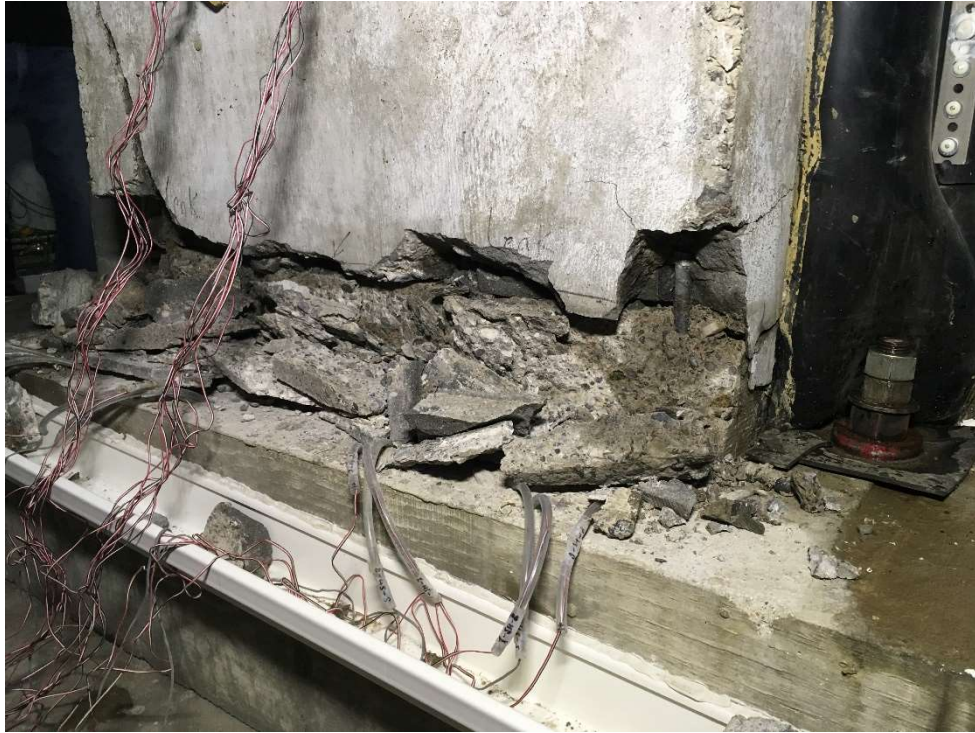
Figure 5-12: Crushing of concrete on the front of the wall in the collapse test of the US joint
