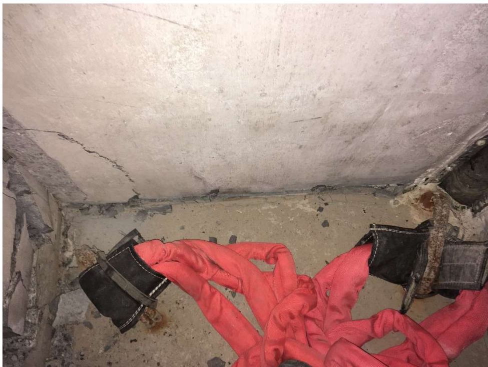
Figure 5-19: Cracking of concrete on the back of the wall in the collapse test of the CF joint
