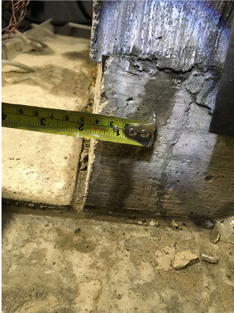
Figure 4-67: Formation of vertical cracks on the compression side of the upturn part
