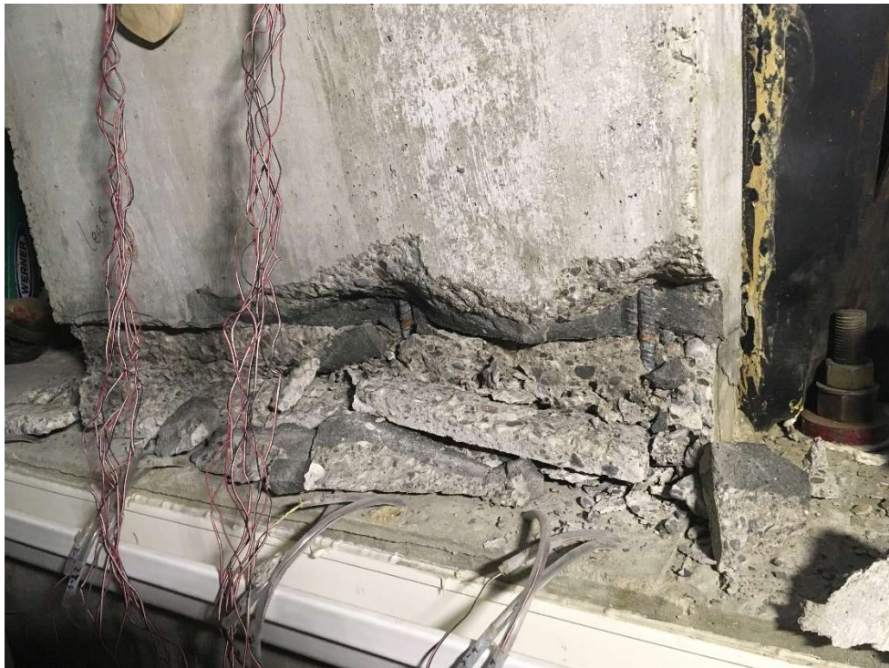
Figure 5-13: Crushing of concrete on the front of the wall in the collapse test of the UF joint
