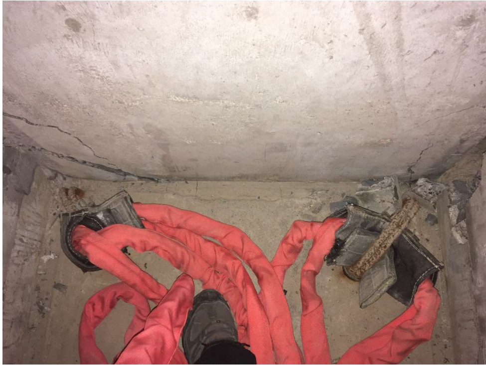
Figure 5-18: Cracking of concrete on the back of the wall in the collapse test of the CF joint
