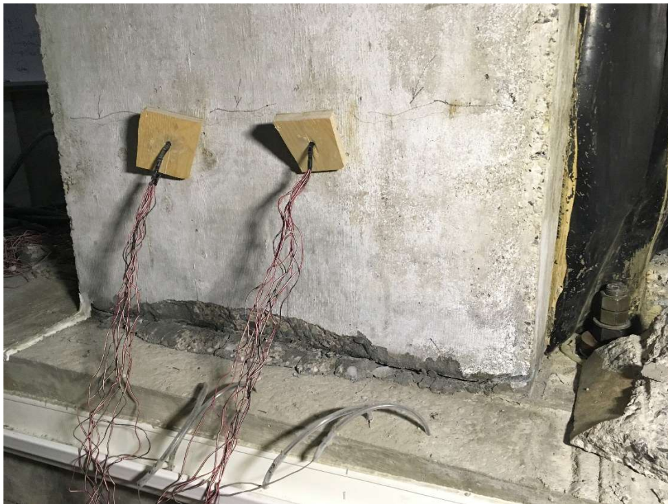
Figure 4-93: Crushing of concrete on the front of the wall at the end of the collapse test of the CF joint
