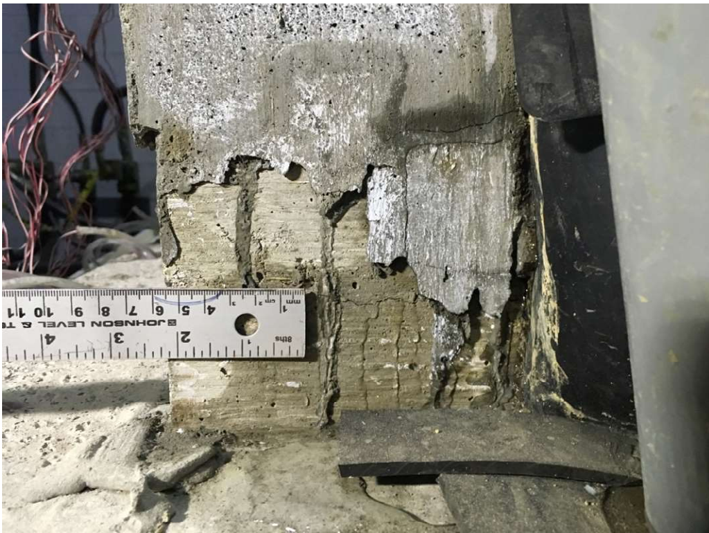
Figure 5-9: Formation of cracks on the tension side of the upturn part in limit state test of the US joint
