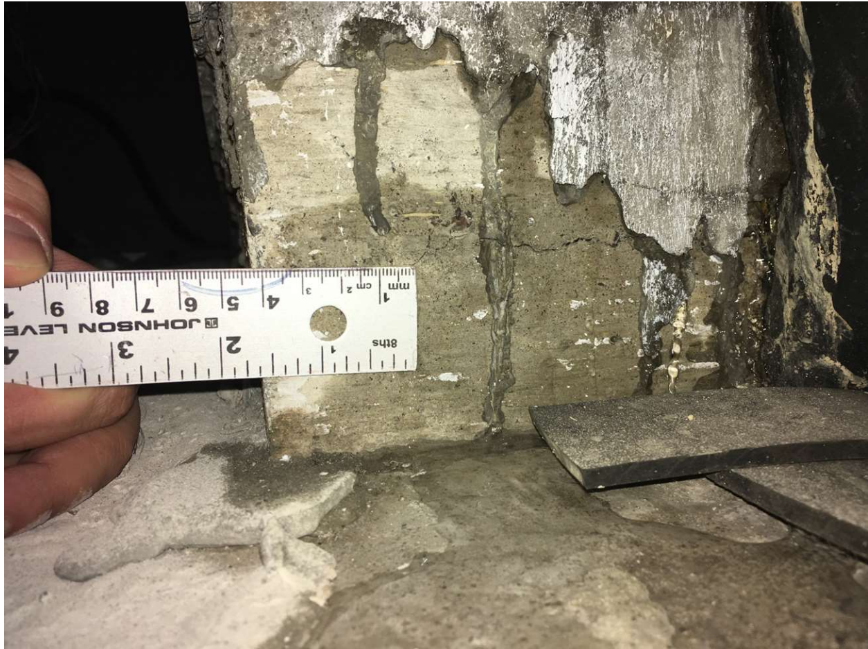
Figure 4-60: Extensive cracking in the upturn part near the end of the test
