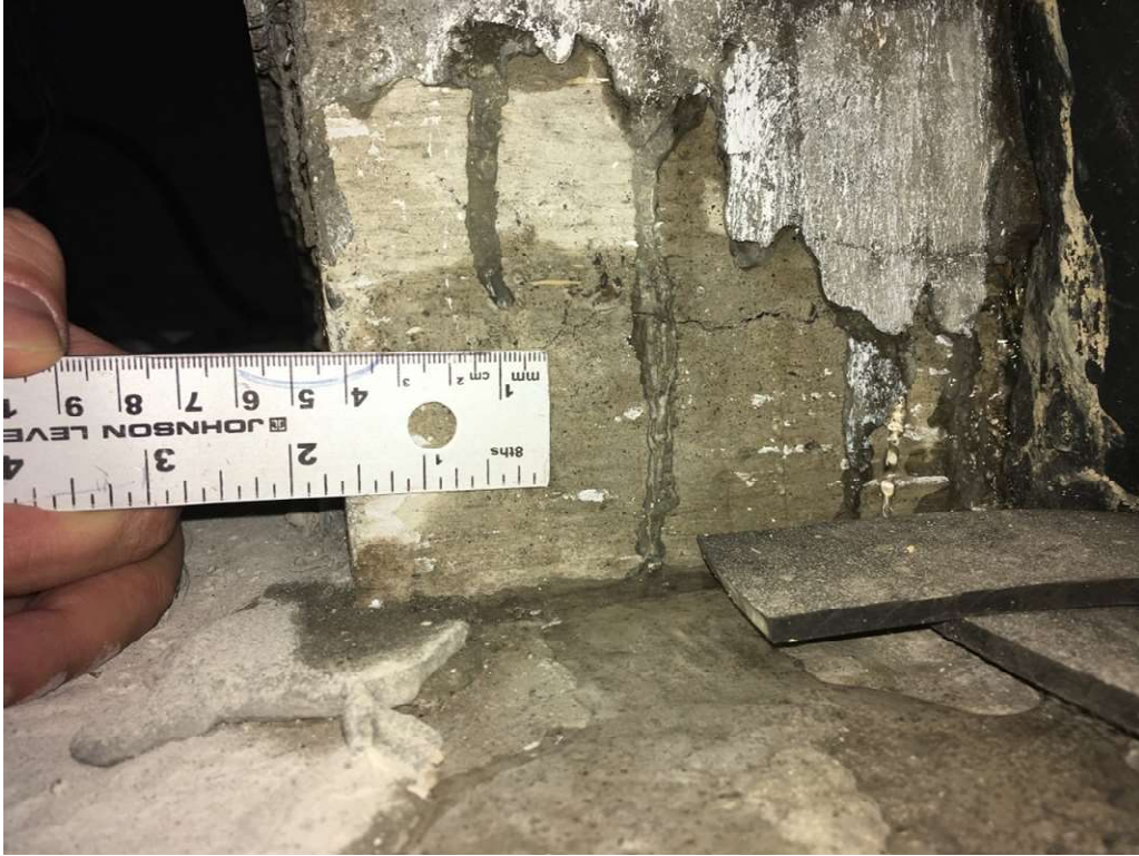
Figure 5-10: Extensive cracking on the upturn part in limit state test of the US joint
