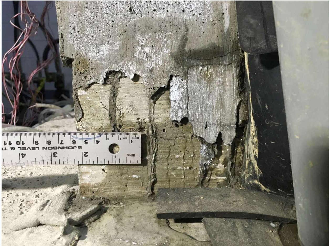
Figure 4-59: Formation of cracks on the tension side of the upturn key
