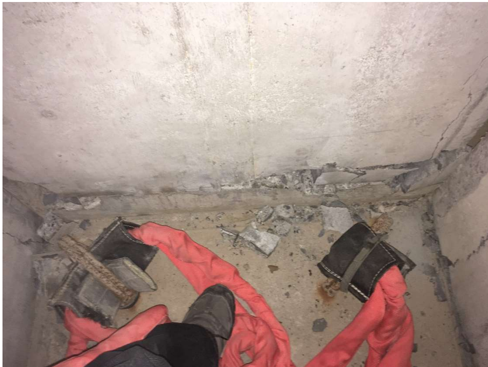
Figure 5-15: Separation of the wall from the upturn part in the collapse test of the UF joint
