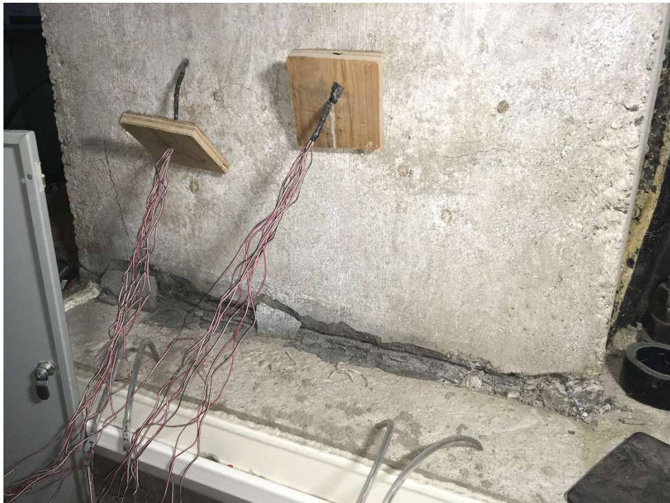
Figure 5-17: Crushing of concrete on the front of the wall in the collapse test of the CS joint
