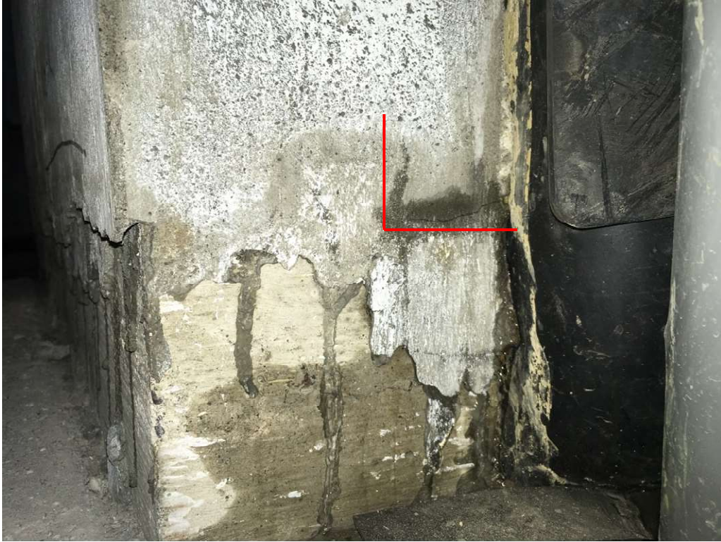
Figure 5-8: Formation of cracks on the outline of the shear key in limit state test of the US joint
