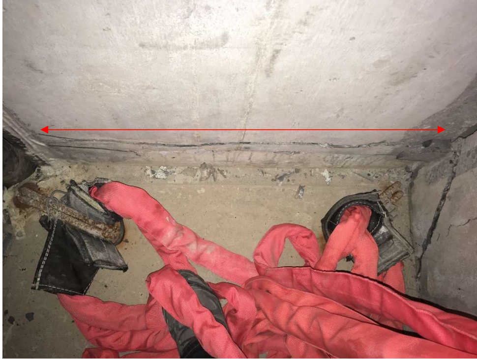
Figure 4-84: Separation of the wall from the upturn part on the back of the wall at the end of the collapse test of the US joint
