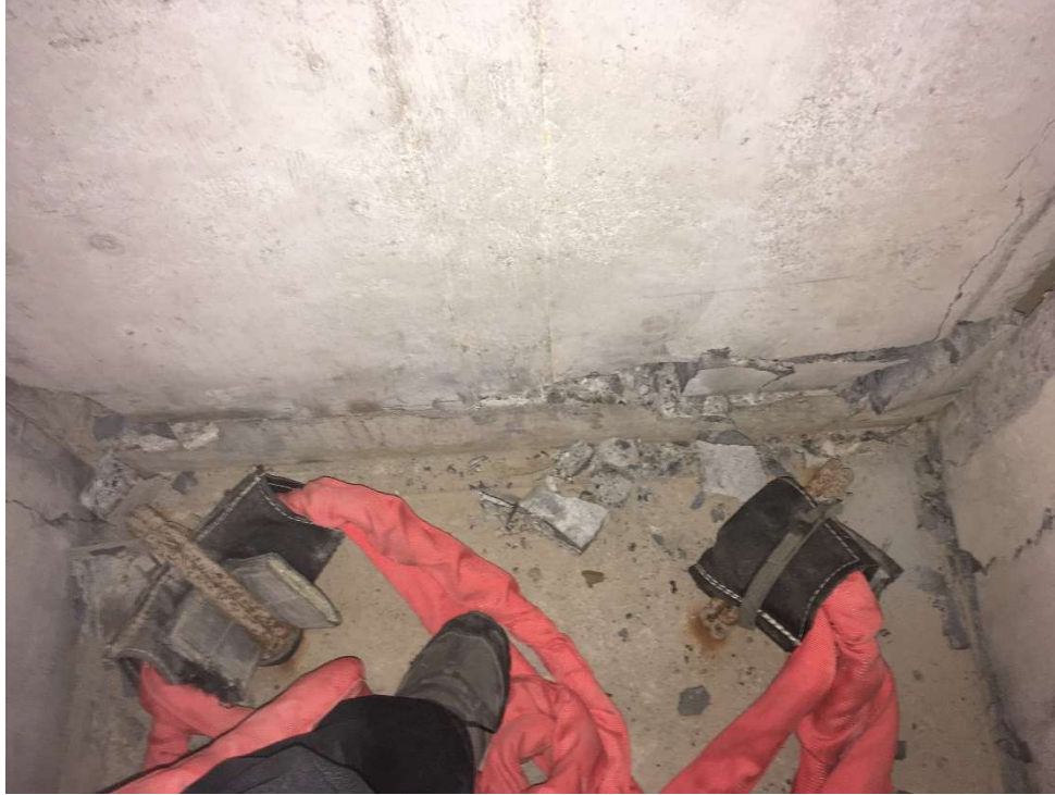
Figure 4-89: Separation of the wall from the upturn part on the back of the wall at the end of the collapse test of the US joint
