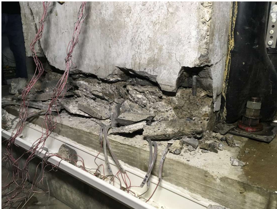
Figure 4-83: Crushing of concrete on the front of the wall at the end of the collapse test of the US joint
