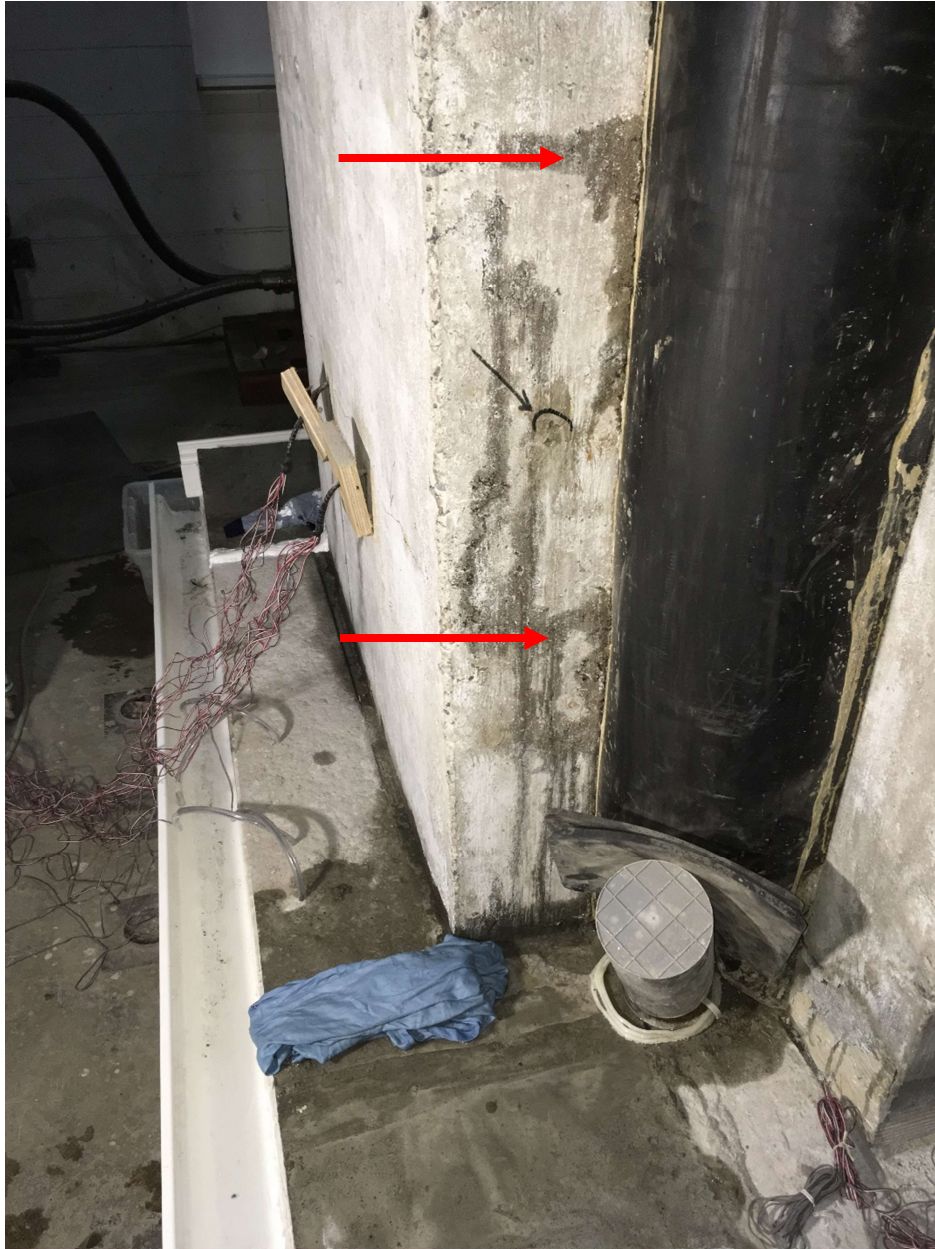
Figure 4-74: Formation of additional cracks along the height of the wall
