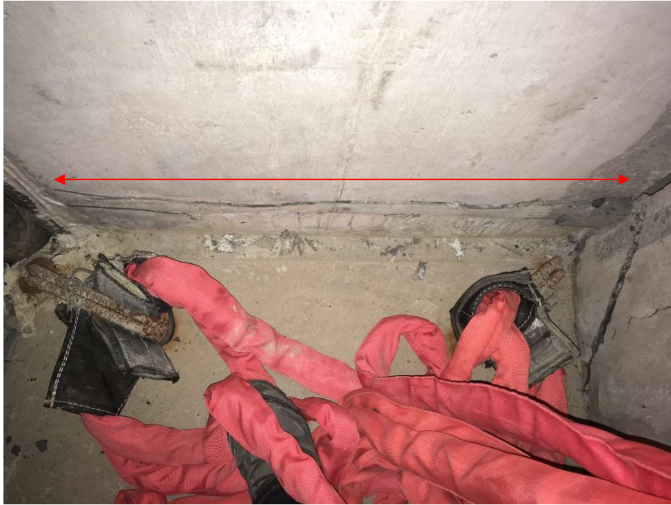
Figure 5-14: Separation of the wall from the upturn part on the back of the wall in the collapse test of the US joint
