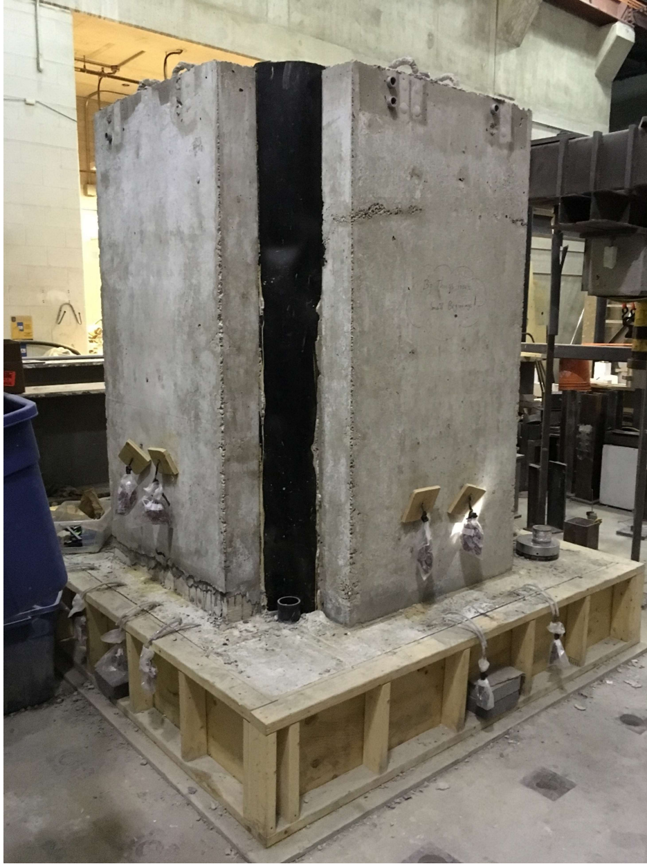
Figure 3-21: The fully constructed concrete tank after the removal of the wall formworks
