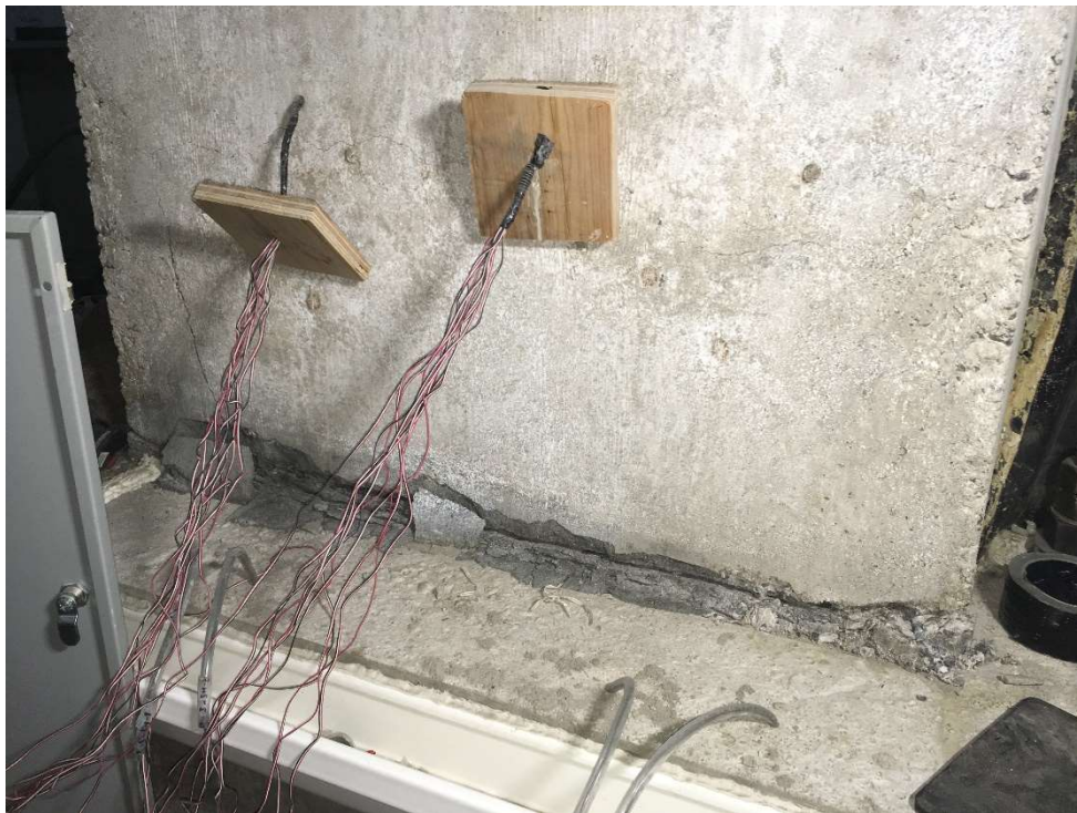
Figure 4-98: Crushing of concrete on the front of the wall at the end of the collapse test of the CS joint
