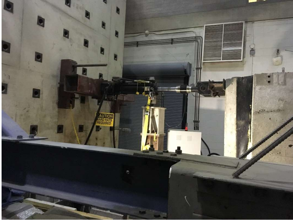
Figure 4-3: Steel pedestals as vertical support for the actuator
