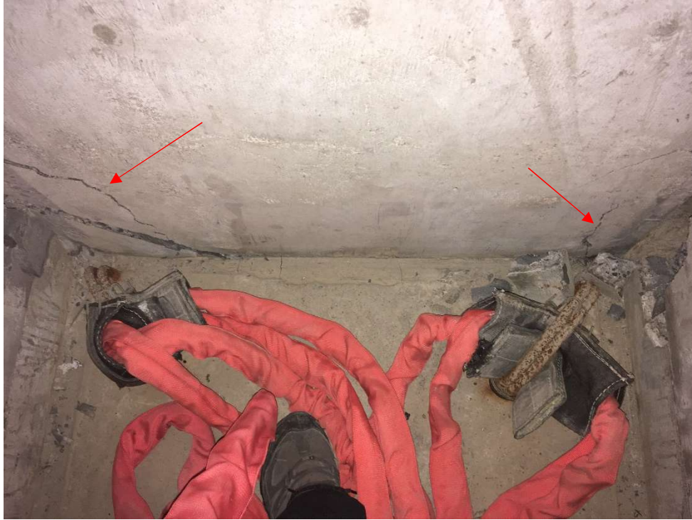
Figure 4-94: Cracking of concrete near the corners on the back of the wall at the end of the collapse test of the CF joint
