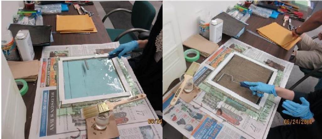
Figure 15: Peel ply and flax fibre wet lay-up process
