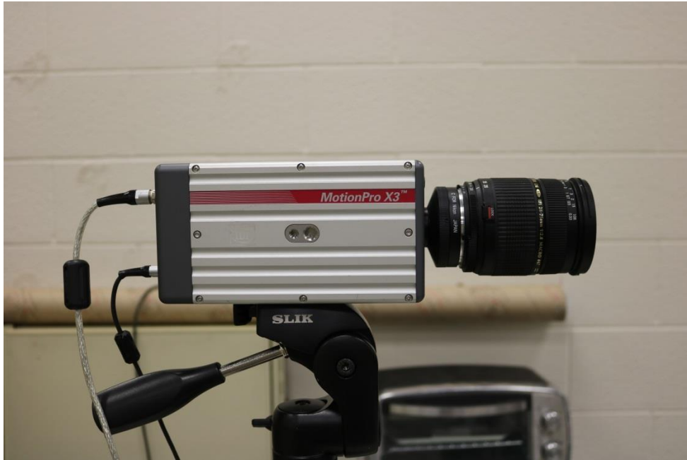
Figure 30. MotionPro X3 High Speed Camera Setup
