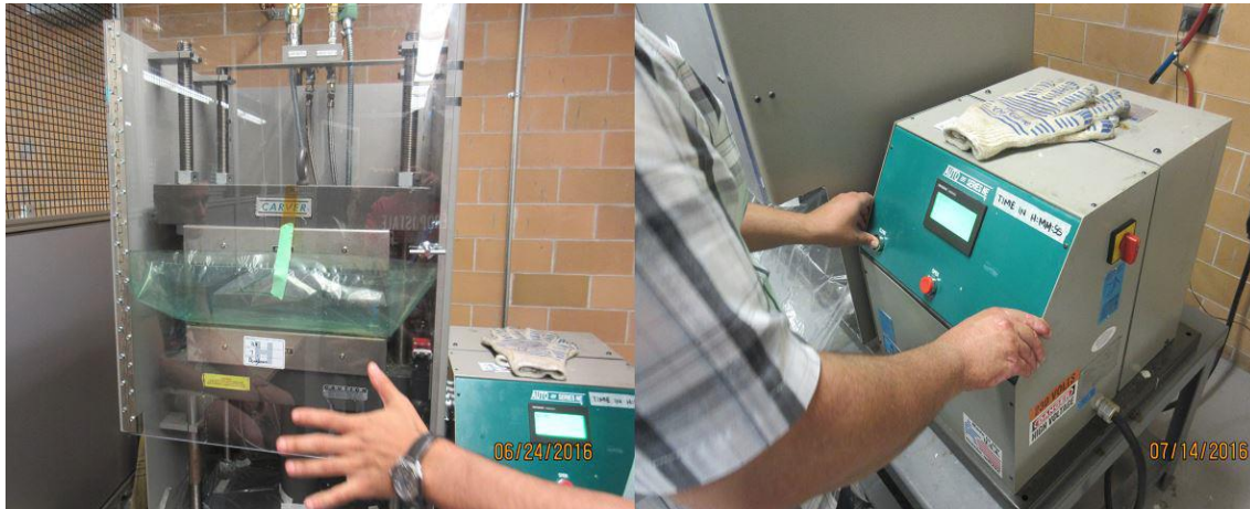
Figure 18: Closing of the protective glass (left) and start of compression (right)
