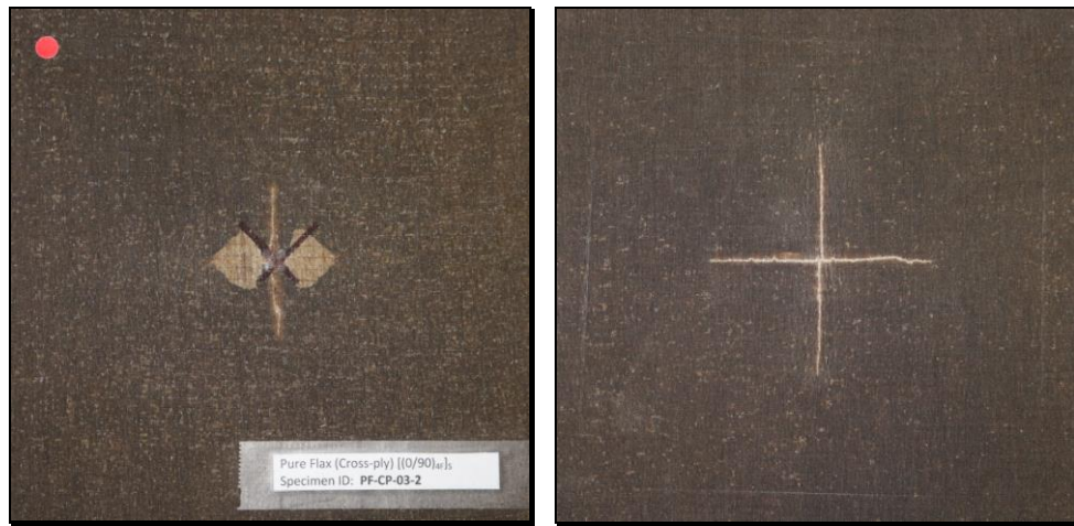
Figure 53: Front face (left); back face damage (right) for [(0/90)_4F]_S at E = 20 \text{ J}
