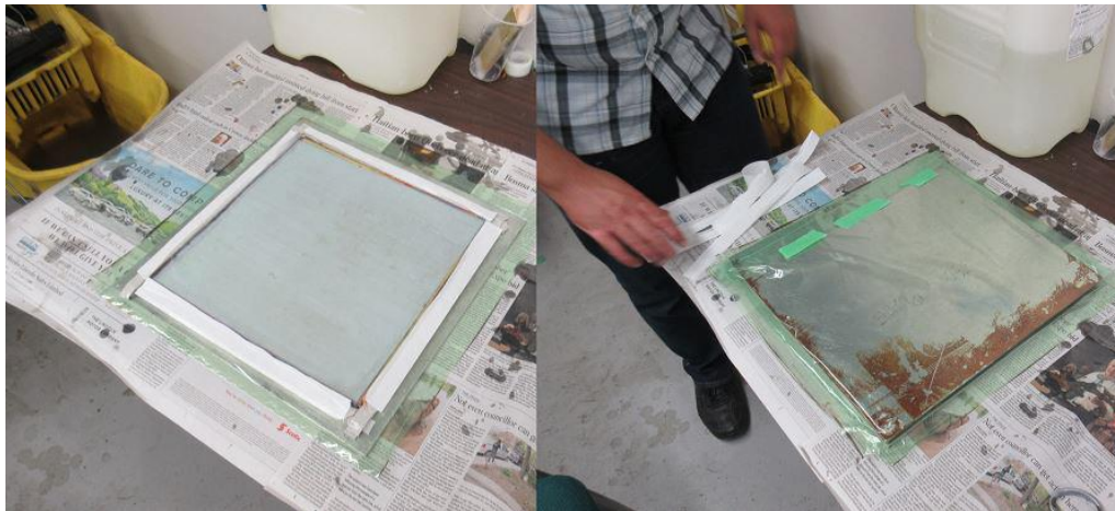
Figure 16: Peel ply application (left) before closing the mould with the top plate (right)
