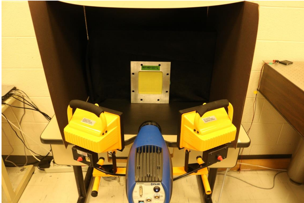
Figure 35. Transient thermographic NDT Setup
