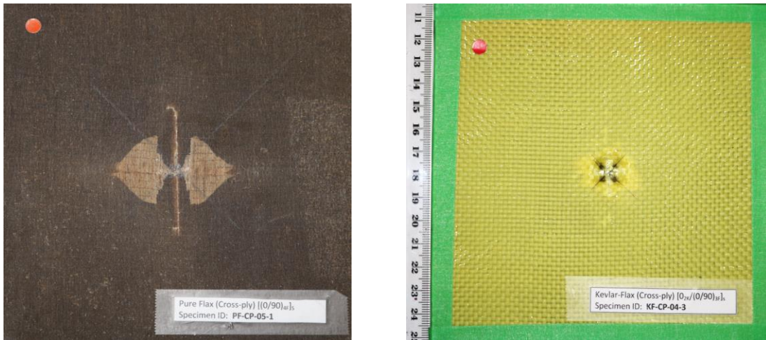
Figure 143: Front face damage to [(0/90)_{4F}]_s and [0_{2K}/(0/90)_{3F}]_s at E = 25 \text{ J}
