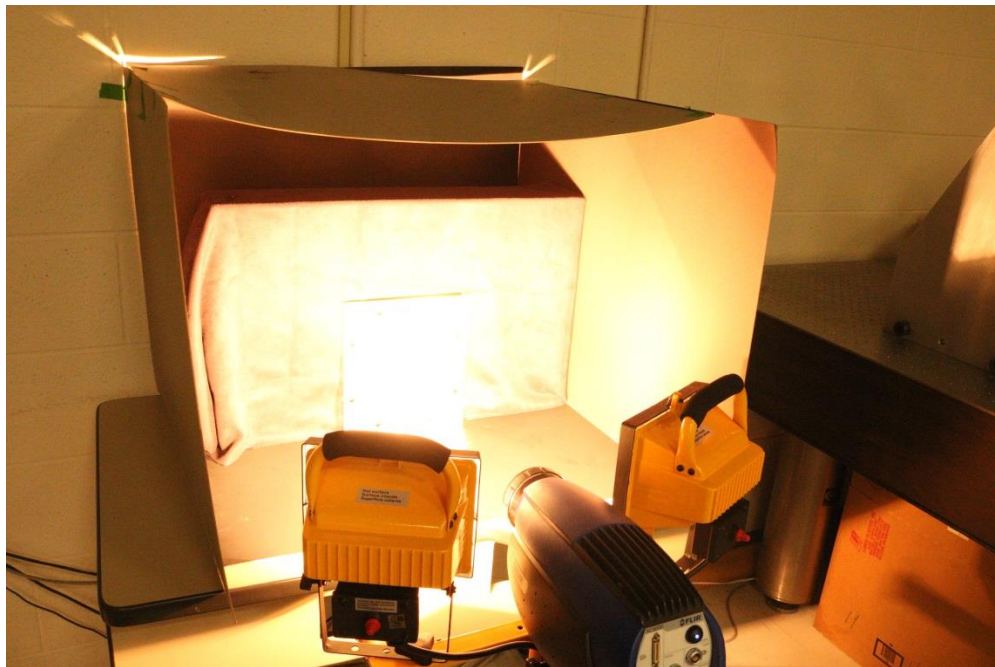
Figure 36. Heating up of the samples during the transient thermographic NDT
