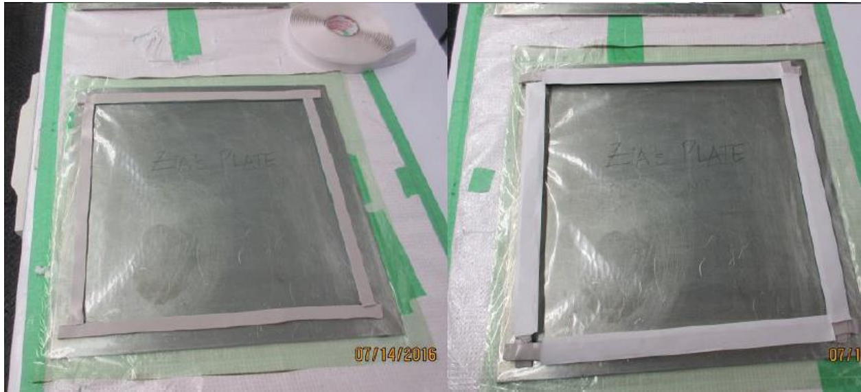
Figure 14: Application of high temperature sealant tape to form the mould cavity
