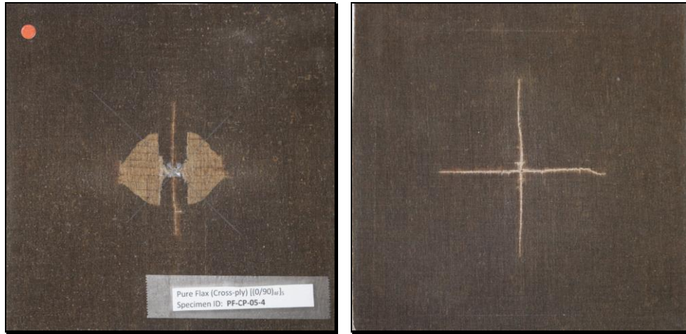
Figure 55: Front face (left); back face damage (right) for [(0/90)_{4F}]_S at E = 27 \text{ J}
