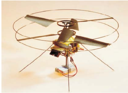
Fig. 2-4 CoaX Coaxial rotor UAV[2]
