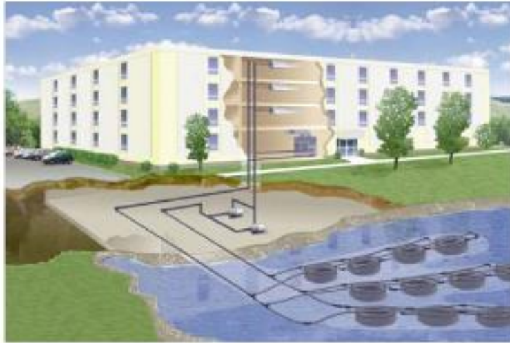
Figure 5 – Pond (Surface Water) GSHP Loop, (reproduced from [12])
