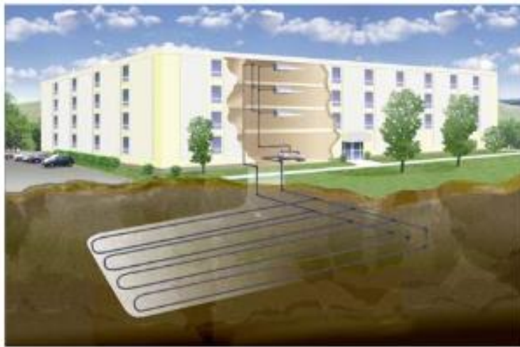
Figure 3 – Horizontal GSHP Loops, (reproduced from [12])
