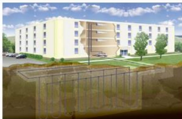
Figure 4 – Vertical GSHP Loops, (reproduced from [12])
