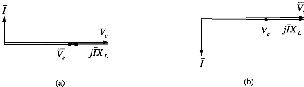
Figure 2-8. Phasor diagram for reactive power control, (a) Leading power factor, (b) Lagging power factor.
