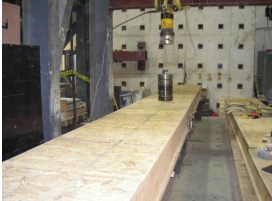
Figure 3.10: View of the wooden joist assembly with 1-kN load placed at the mid-span to measure static deflection
