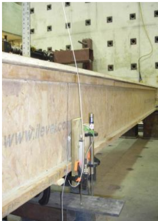
Figure 3.9: View of the LVDT attached to the wooden joist
