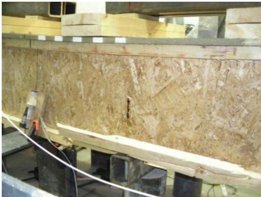
Figure E.12: Close-up view of the bending fracture of the bottom flange and web of the 406x7950 mm wooden joist assembly
