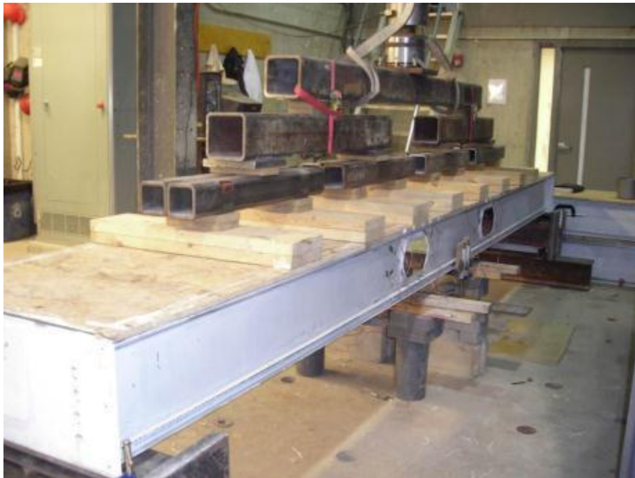
Fig. 3.39: View of the uniformly distributed loading applied to the iSPAN floor joist assembly with web holes
