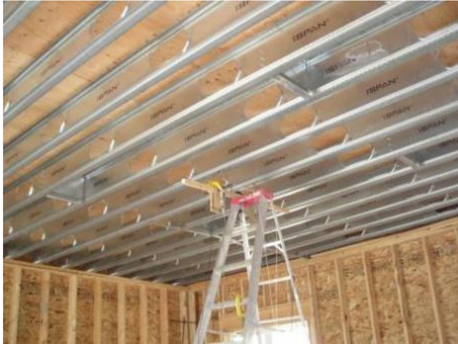
Figure 3.49: View of the LVDTs and accelerometers attached to the bottom flange of iSPAN joist in test site 2
