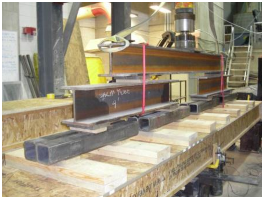
Figure 3.15: View of the uniformly distributed loading applied to the wooden floor joist assembly
