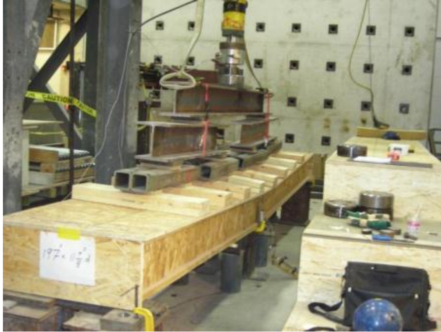
Figure E.5: View of the deformed shape at failure of the 302x5000 mm wooden joist assembly
