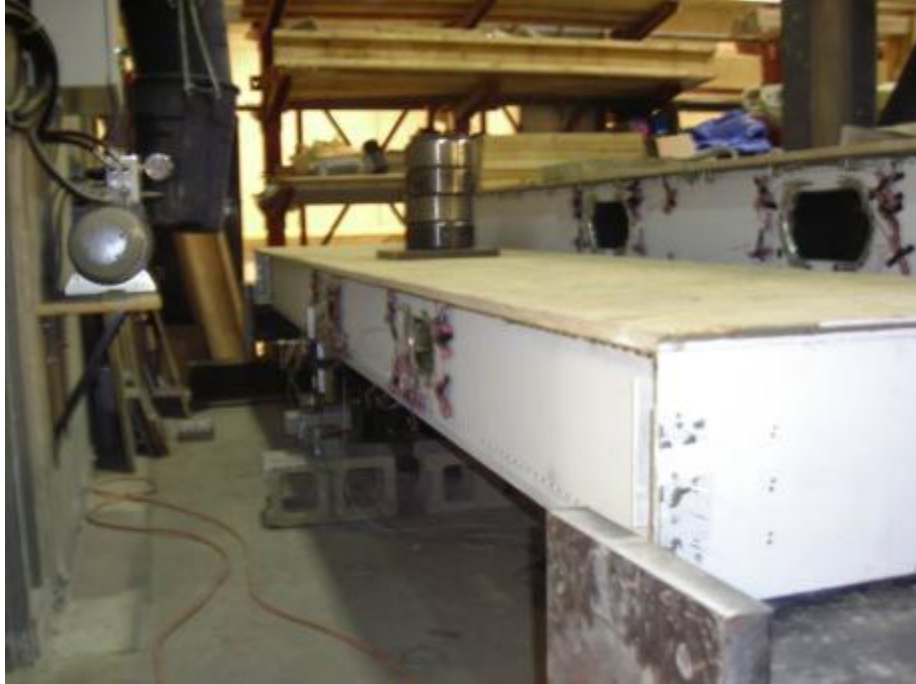
Figure 3.38: View of the iSPAN joist with web holes on which a 1-kN load was placed at mid-span to measure static deflection considering simply-supported framing
