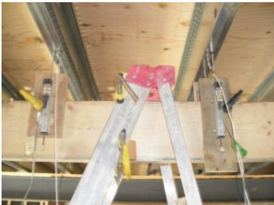
Figure 3.45: Close-up view of the LVDTs and accelerometers attached to the bottom flange of iSPAN joist in test site 1
