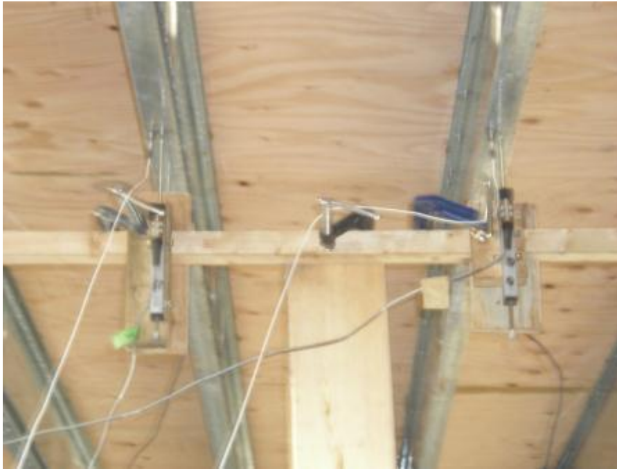
Figure 3.53: View of the LVDTs and accelerometers attached to the bottom flange of iSPAN joist in test site 3
