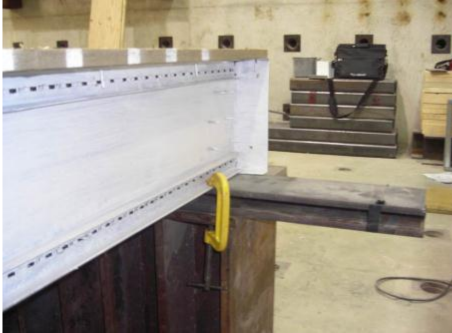
Figure 3.34: View of the clamping system at support to avoid bouncy effect on iSPAN joist assembly with simply-supported framing
