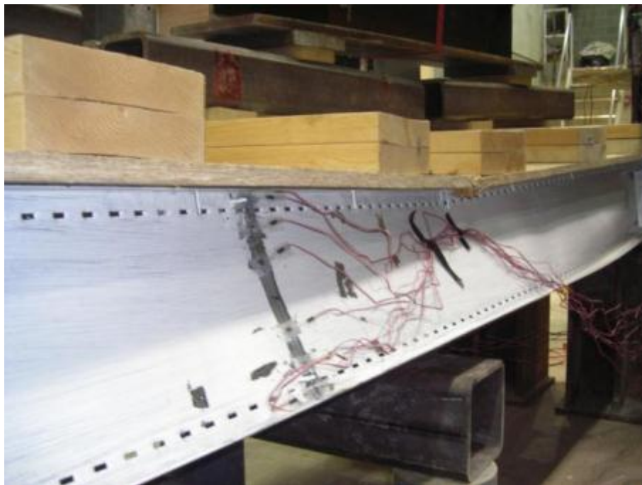
Figure E.14: Close-up view of the lateral torsional buckling failure of the 241x3500 mm iSPAN joist assembly
