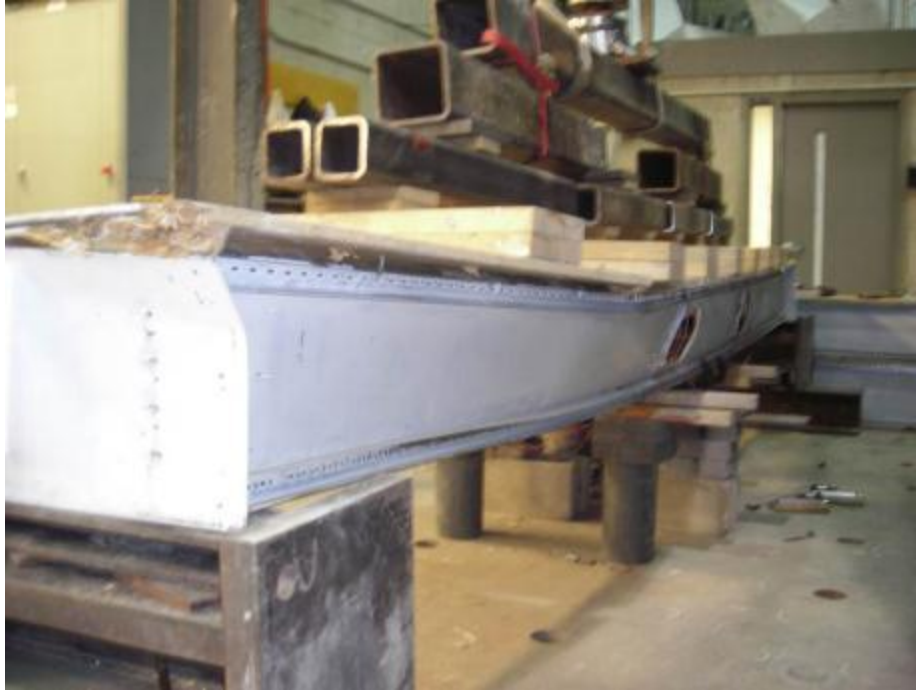
Figure 4.14: View of an iSPAN twin-joist assembly with web hole after failure due to lateral torsional buckling failure
