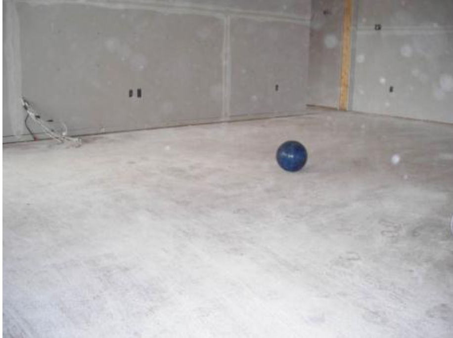
Figure 3.46: View of the bowling ball dropped from a height of 0.3 m over the floor in test site 1
