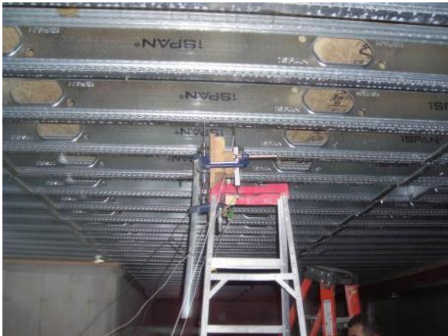
Figure 3.56: View of the LVDTs and accelerometers attached to the bottom flange of iSPAN joist in test site 4
