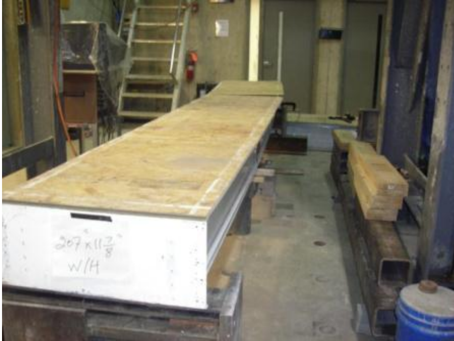
Figure E.32: View of lateral torsional buckling failure of the 302x5250 mm iSPAN joist assembly with web holes
