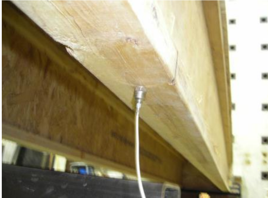
Figure 3.12: View of the accelerometer attached to the bottom flange of the wooden joist
