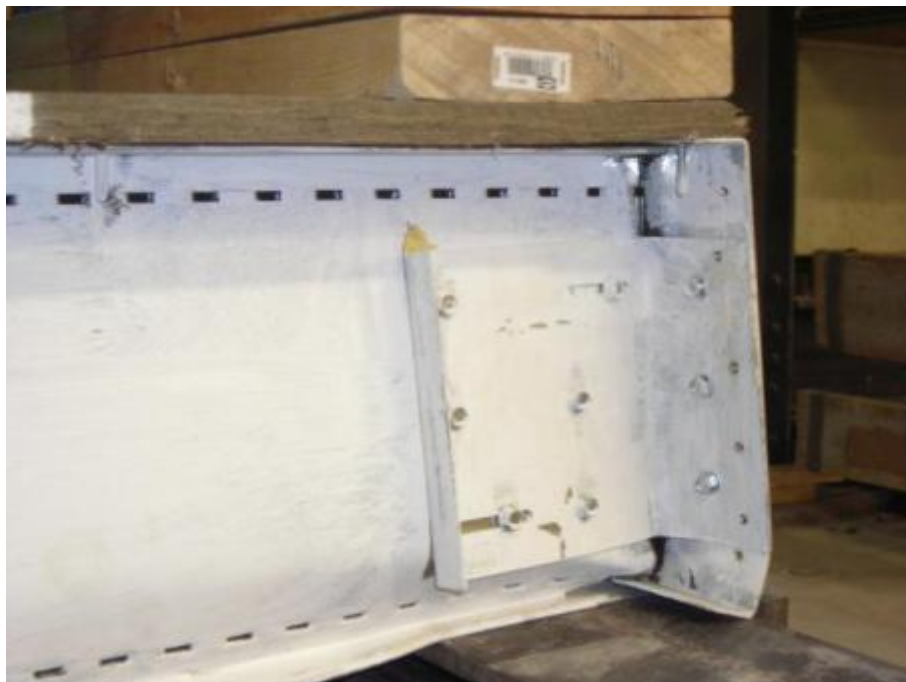
Figure E.27: View of web and rim board crippling at failure at support of the 254x3500 mm iSPAN joist assembly with web holes
