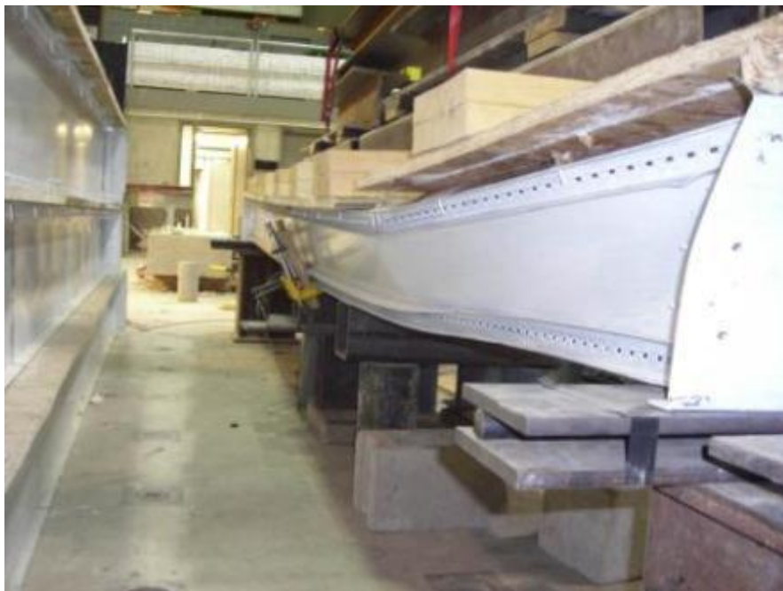
Figure 4.12: View of an iSPAN twin-joist assembly without web holes after failure due to global lateral torsional buckling
