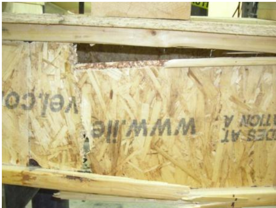
Figure E.10: Close-up view of the bottom flange and web fracture and top flange-web separation at failure of the 356x6100 mm wooden joist assembly
