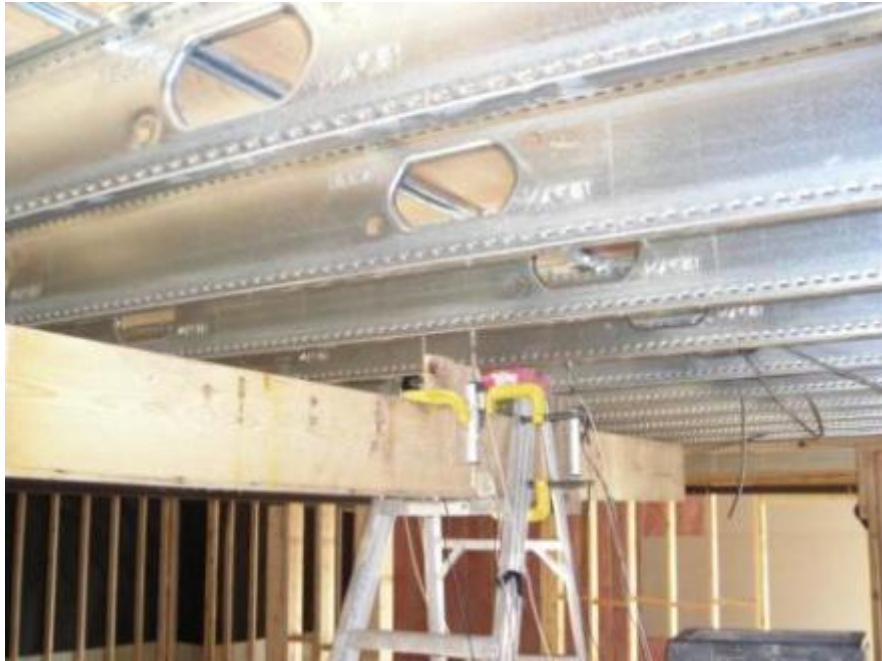
Figure 3.44: View of the LVDTs and accelerometers attached to the bottom flange of iSPAN joist floor in test site 1
