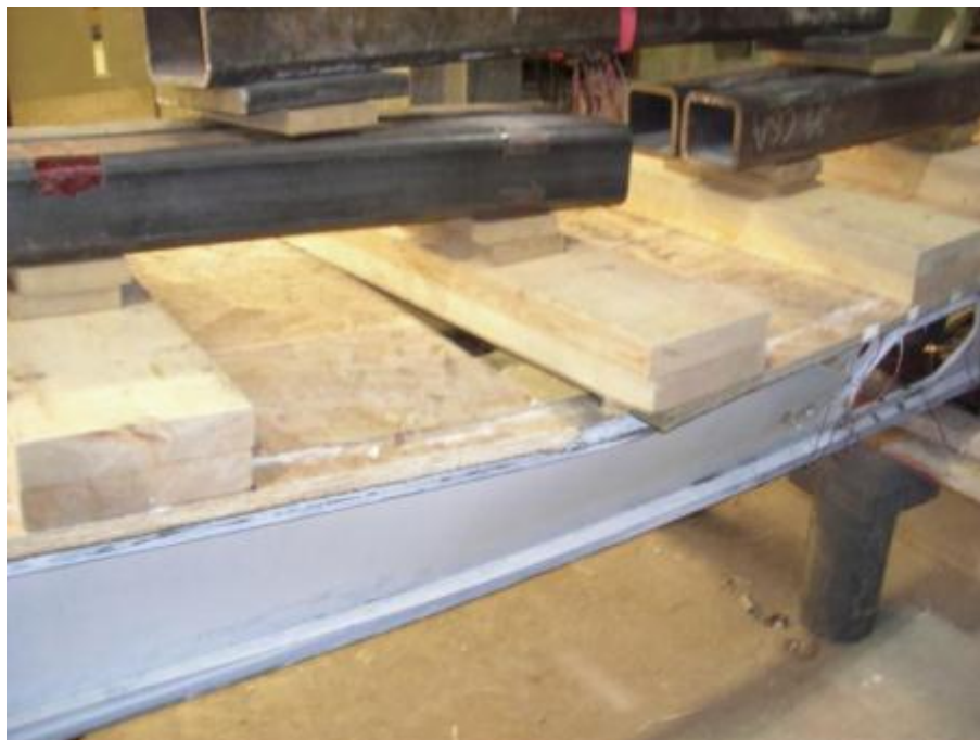
Figure E.31: Close-up view of lateral torsional buckling failure along with OSB separation normal to the joist of 302x5000 mm iSPAN joist assembly
