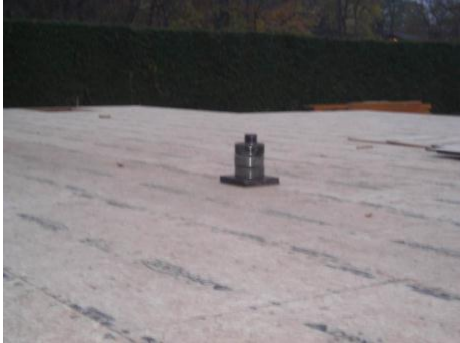
Figure 3.57: View of the 1-kN load placed at mid-span of the joist to measure static deflection in test site 4
