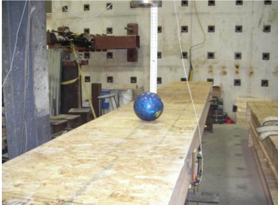
Figure 3.14: View of the bowling ball dropped over the wooden joist assembly from a height of 0.3 m
