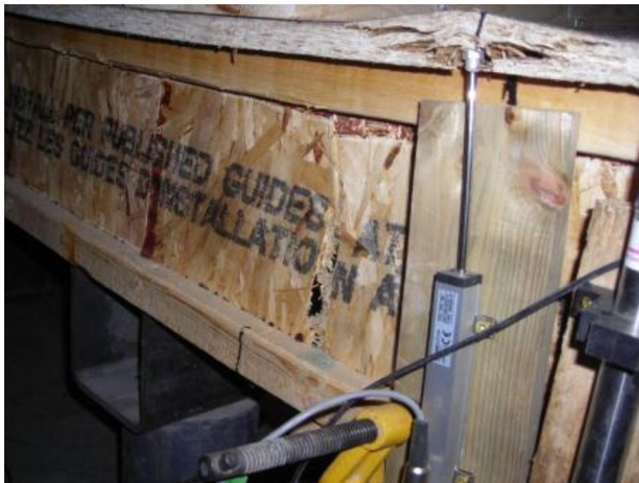
Figure E.2: Close-up view of the bending fracture of the OSB web and top flange-OSB web separation at failure of the 241x3500 mm wooden joist assembly
