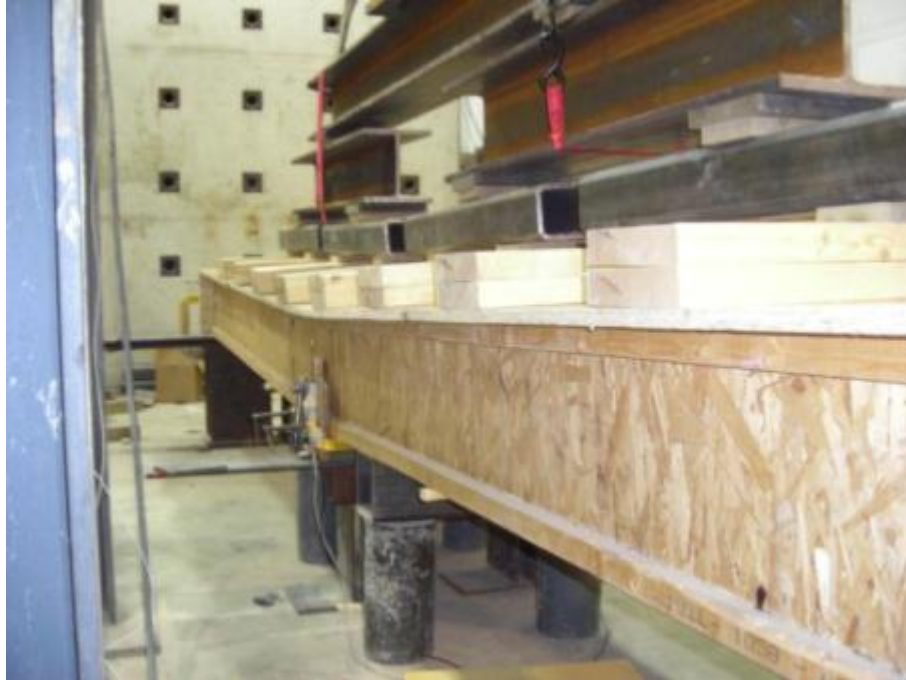
Figure E.7: View of the deformed shape at failure of the 302x5250 mm wooden joist assembly
