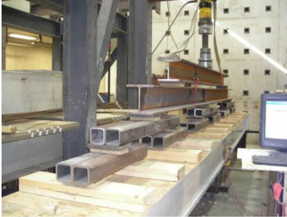
Fig. 3.36: View of the uniformly distributed loading applied to the iSPAN floor joist assembly
