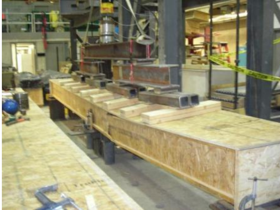
Figure E.9: View of the deformed shape at failure of the 356x6100 mm wooden joist assembly
