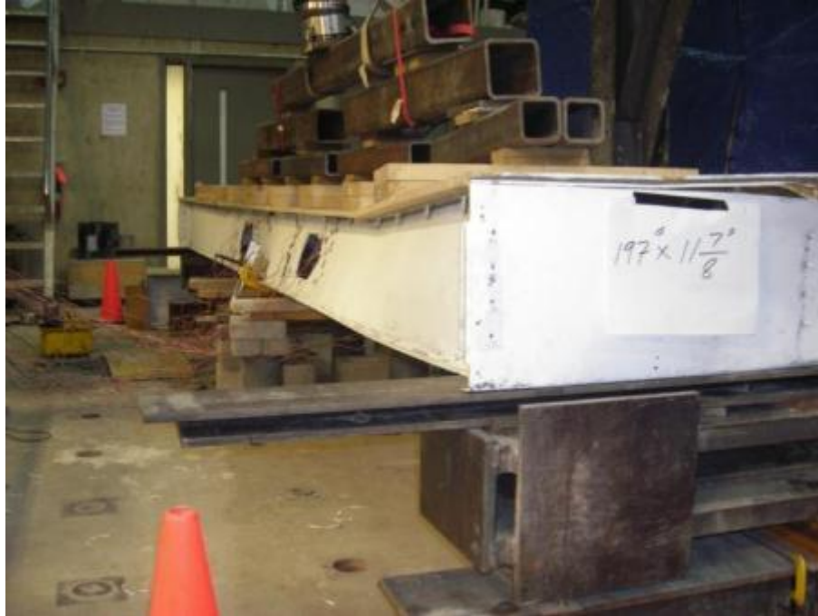
Figure E.30: View of the lateral torsional buckling failure of the 302x5000 mm iSPAN joist assembly with web holes
