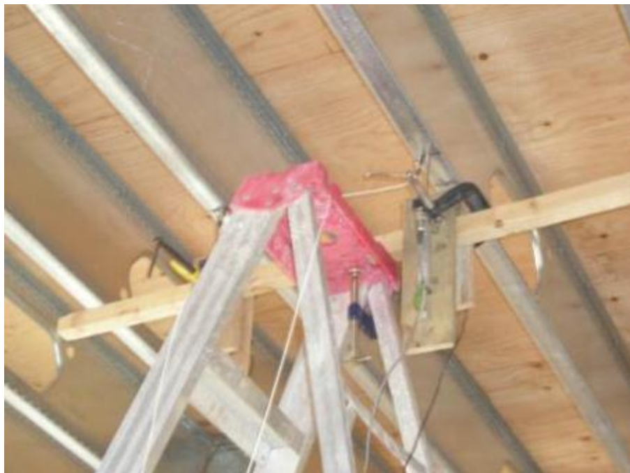
Figure 3.50: Close-up view of the LVDTs and accelerometers attached to the bottom flange of iSPAN joists in test site 2
