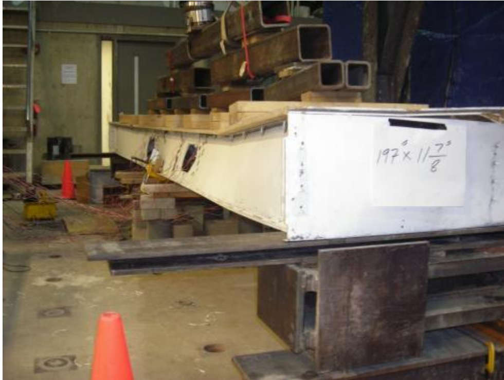
Figure 5.16: View of the experimental lateral torsional buckling shape of the 300x5000 mm iSPAN joist assembly
