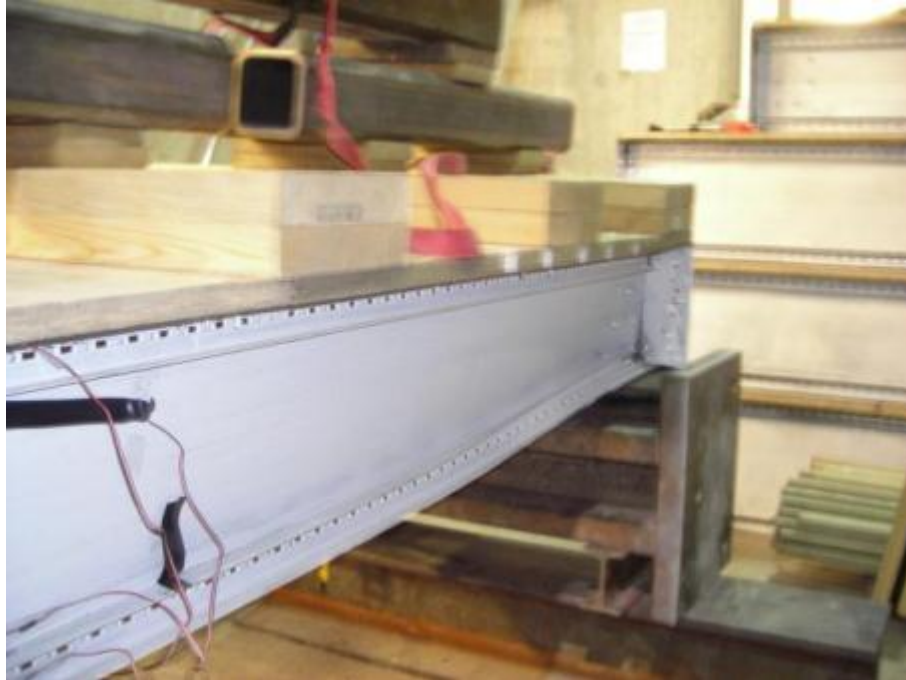
Figure E.26: View of the deformed shape at failure of the 254x3500 mm iSPAN joist assembly at support
