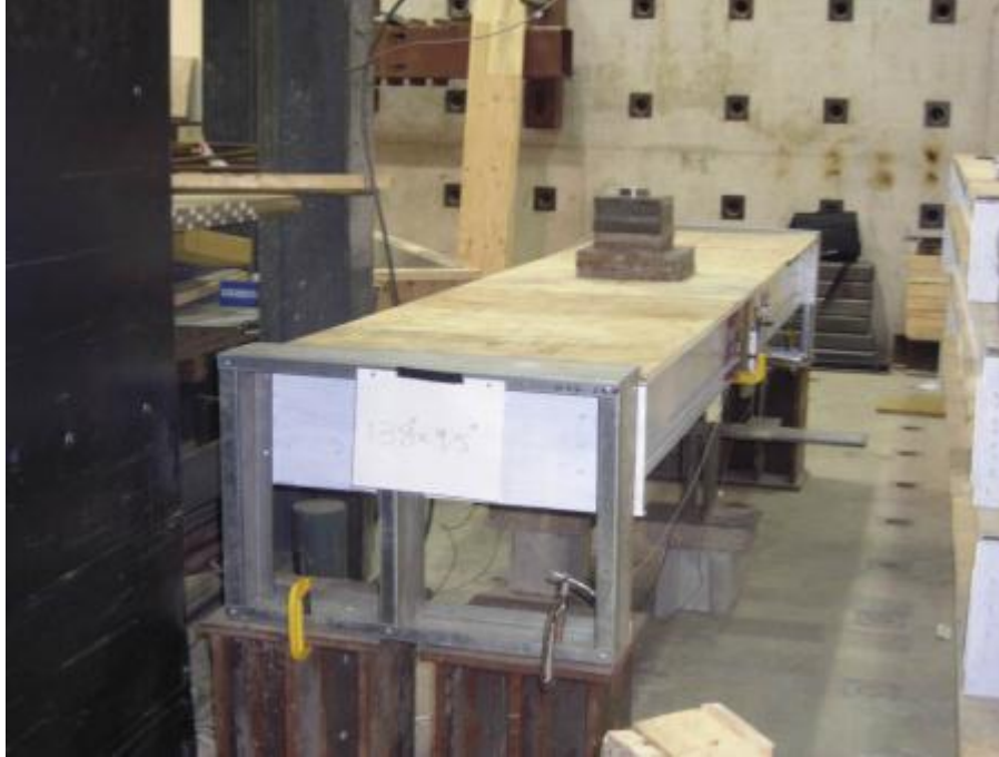
Figure 3.30: View of the iSPAN joist assembly with 1-kN load placed at the mid-span to measure deflection in case of balloon framing
