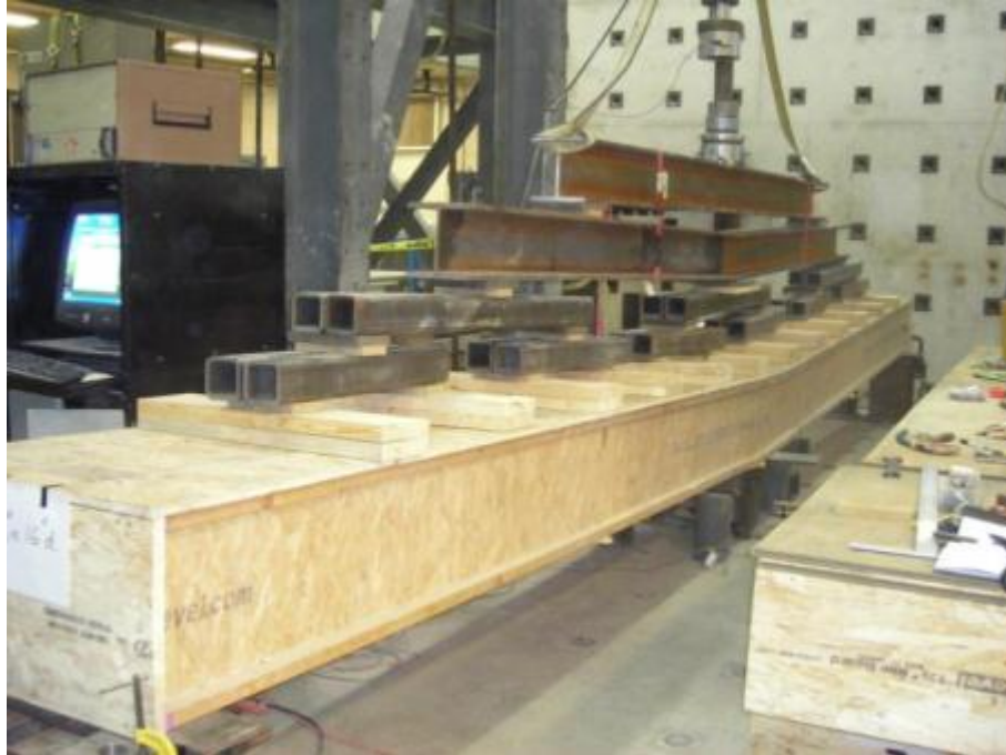
Figure E.11: View of the deformed shape at failure of the 406x7950 mm wooden joist assembly
