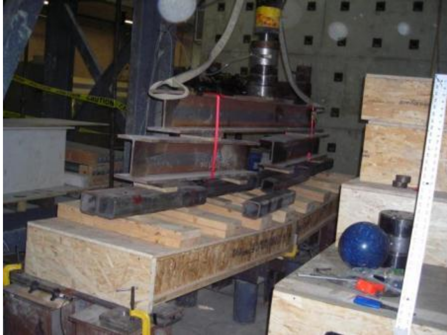
Figure E.1: View of deformed shape at failure of the 241x3500 mm wooden joist assembly
