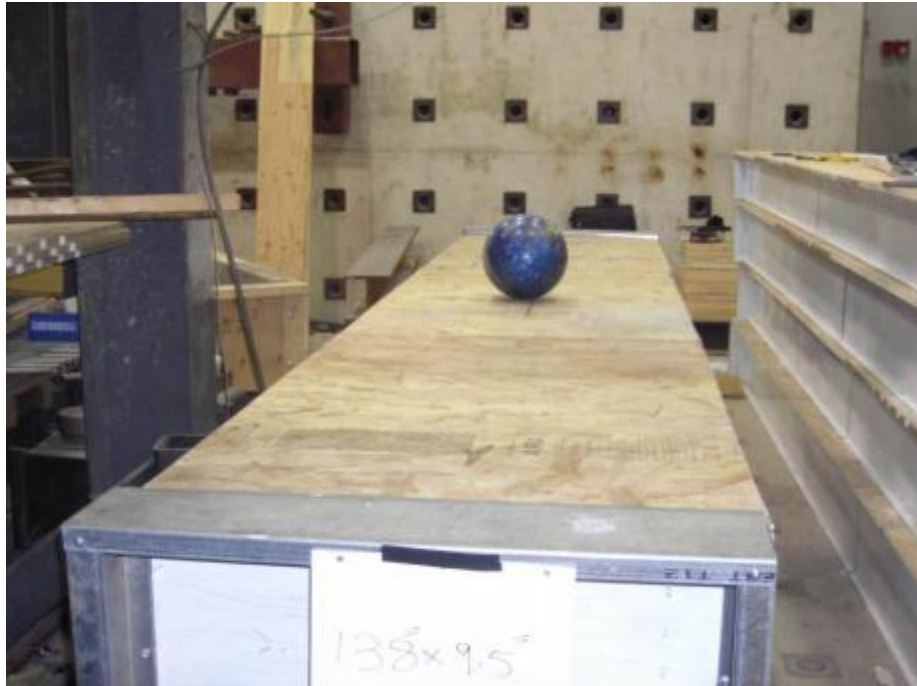
Figure 3.32: View of the bowling ball dropped from a height of 0.3 m over the iSPAN joist assembly with balloon framing
