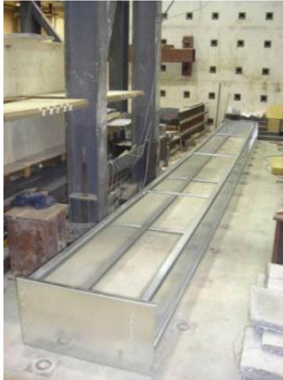
Figure 3.26: View of the bracing attached to the iSPAN joists at the quarter points of the iSPAN joists (note that the joists are upside down in this photo)
