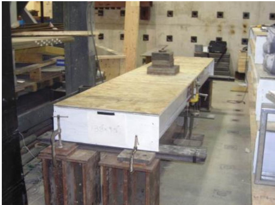
Figure 3.33: View of the iSPAN joist with 1-kN load placed at mid-span to measure static deflection of the assembly with simply-supported framing
