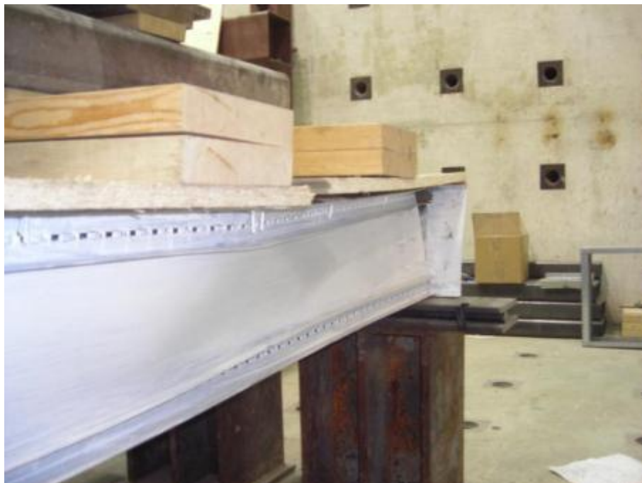
Figure E.16: Close-up View of lateral torsional buckling failure of the 241x4500 mm iSPAN joist assembly along with rim board separation from the joist at the support
