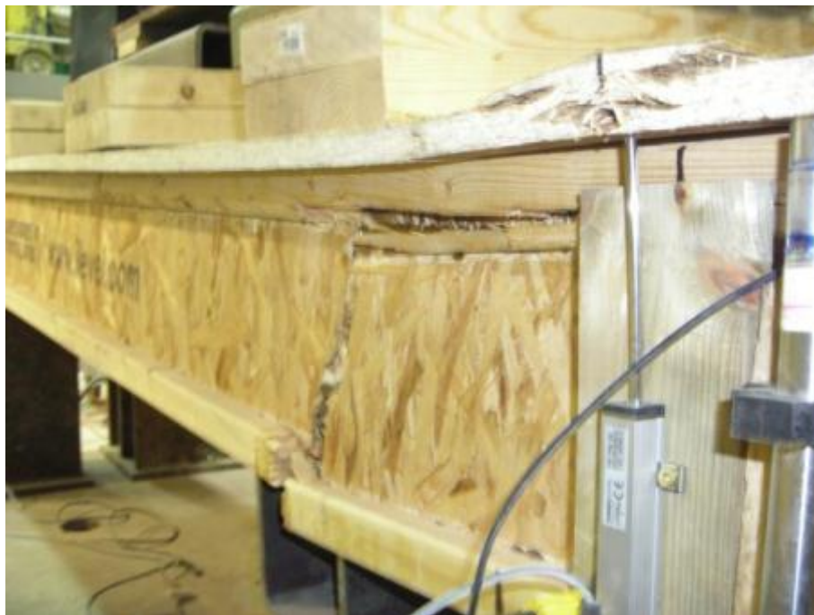
Figure E.4: Close-up view of bending fracture of the joist and top flange-OSB web separation of 241x4500 mm wooden joist assembly
