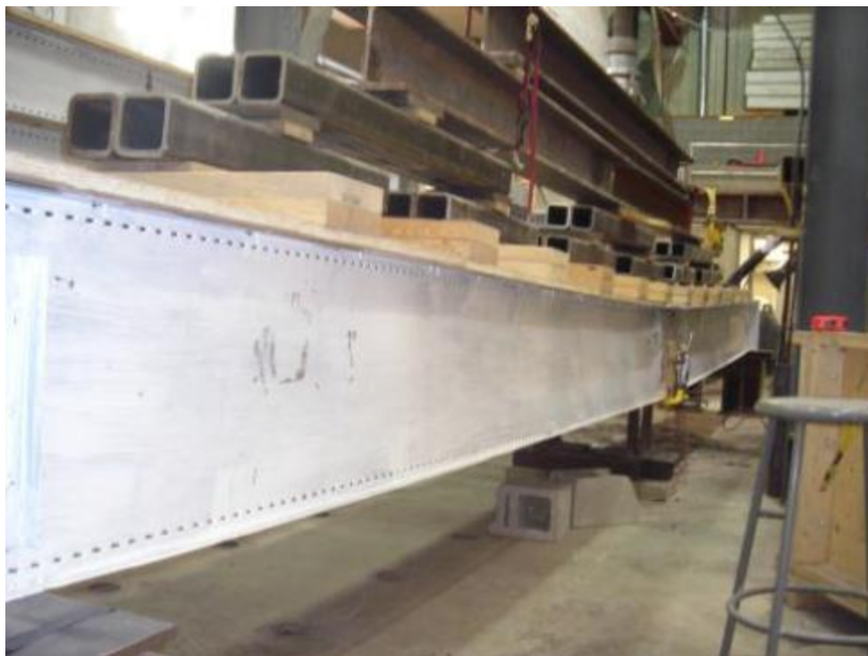
Figure 5.12: View of the experimental deformed shape at failure of the 406x7950 mm iSPAN joist assembly
