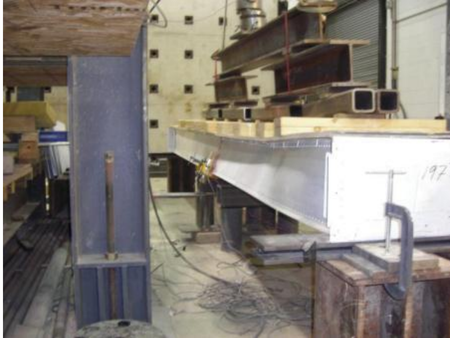
Figure E.17: View of lateral torsional buckling failure of the 302x5000 mm iSPAN joist assembly
