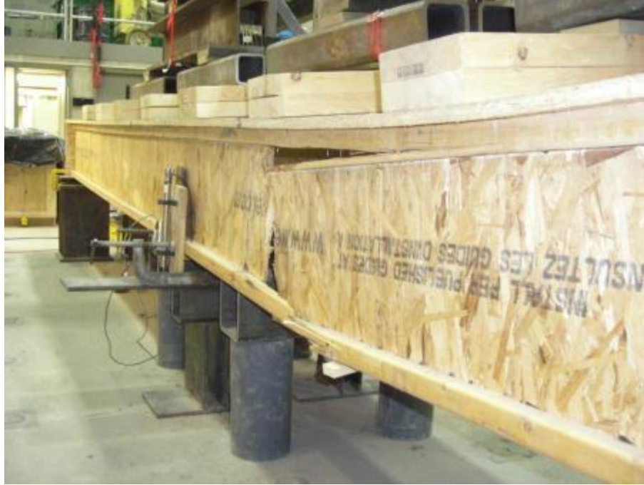
Figure 4.5: Close-up view of a wooden twin-joist assembly showing joist flexural failure and OSB-joist top flange separation
