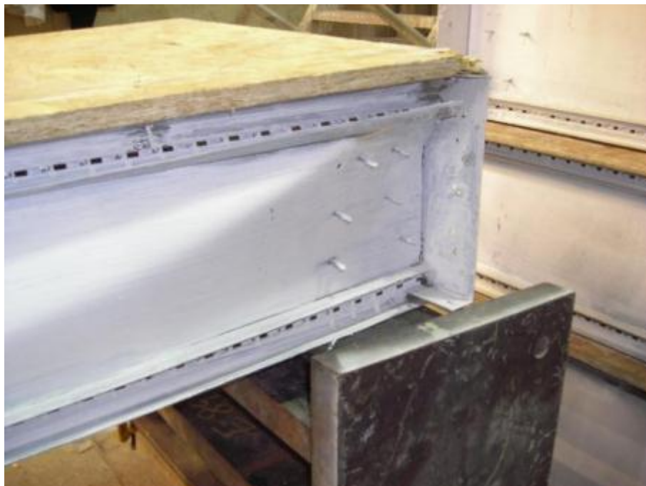
Figure E.29: Close-up view of lateral torsional buckling failure of the 254x4500 mm iSPAN joist assembly with web holes
