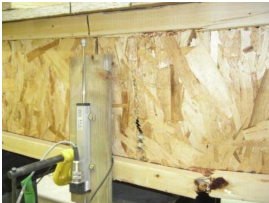
Figure E.6: Close-up view of the bending fracture of bottom flange and web of the 302x5000 mm wooden joist assembly at failure
