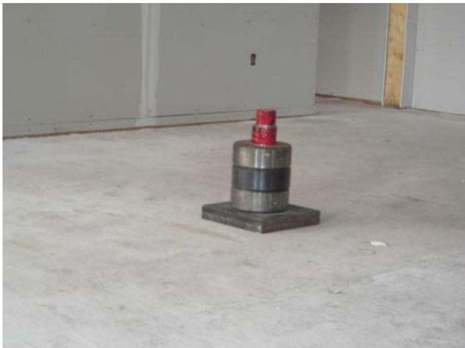
Figure 3.47: View of the 1-kN load placed at mid-span of the joist to measure the static deflection in test site 1
