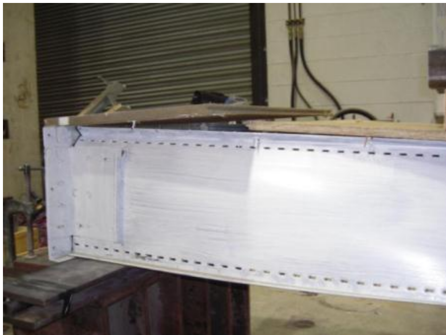
Figure E.20: View of splitting of the OSB sheets and separation of OSB sheet and the top flange at the support region of the 302x5250 mm iSPAN joist assembly
