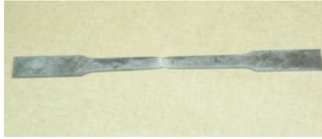
Figure 3.61: View of the failure shape in one of the tested coupons
