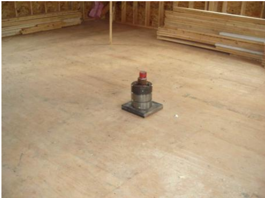
Figure 3.52: View of the 1-kN load placed at mid-span of the joist to measure the static deflection in test site 2
