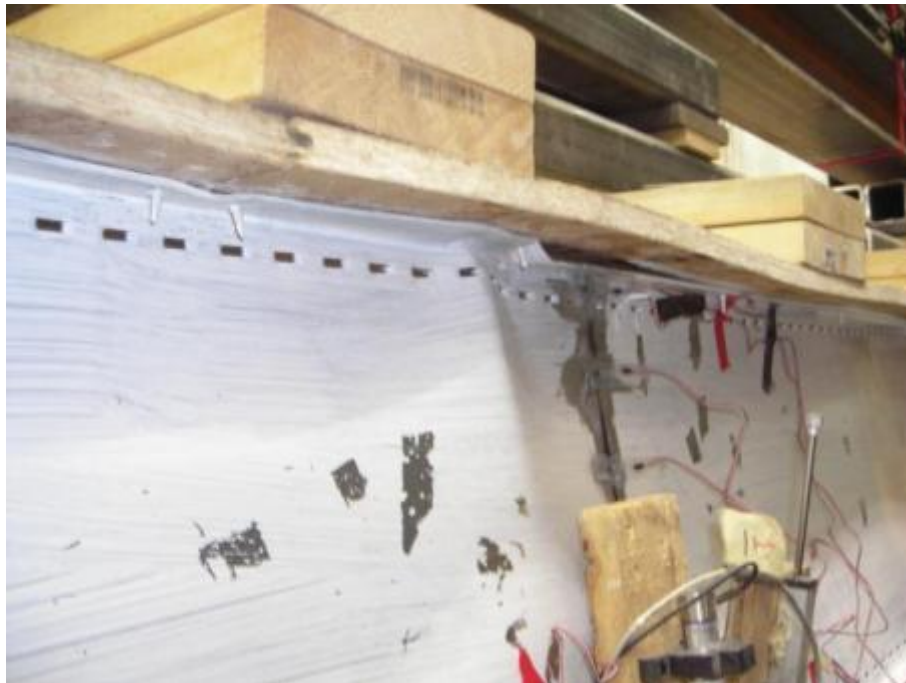
Figure E.24: Close-up view of the local buckling of the top flange along with web local buckling at the mid-span region of the 406x7950 mm iSPAN joist assembly
