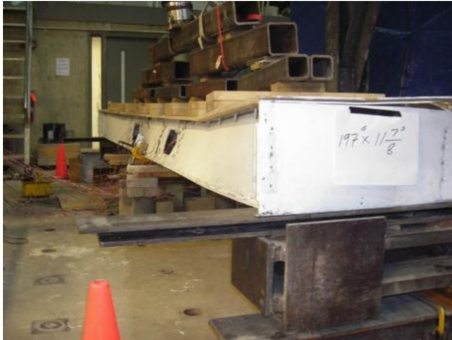
Figure 4.13: View of an iSPAN twin-joist assembly with web hole after failure due to lateral torsional buckling failure
