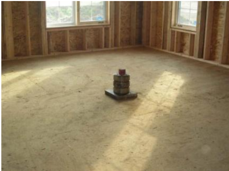
Figure 3.54: View of the 1-kN load placed at mid-span of the joist to measure static deflection in tests site 3
