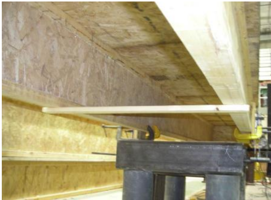
Figure 3.13: View of the transverse strap to brace the wooden joist at quarter point
