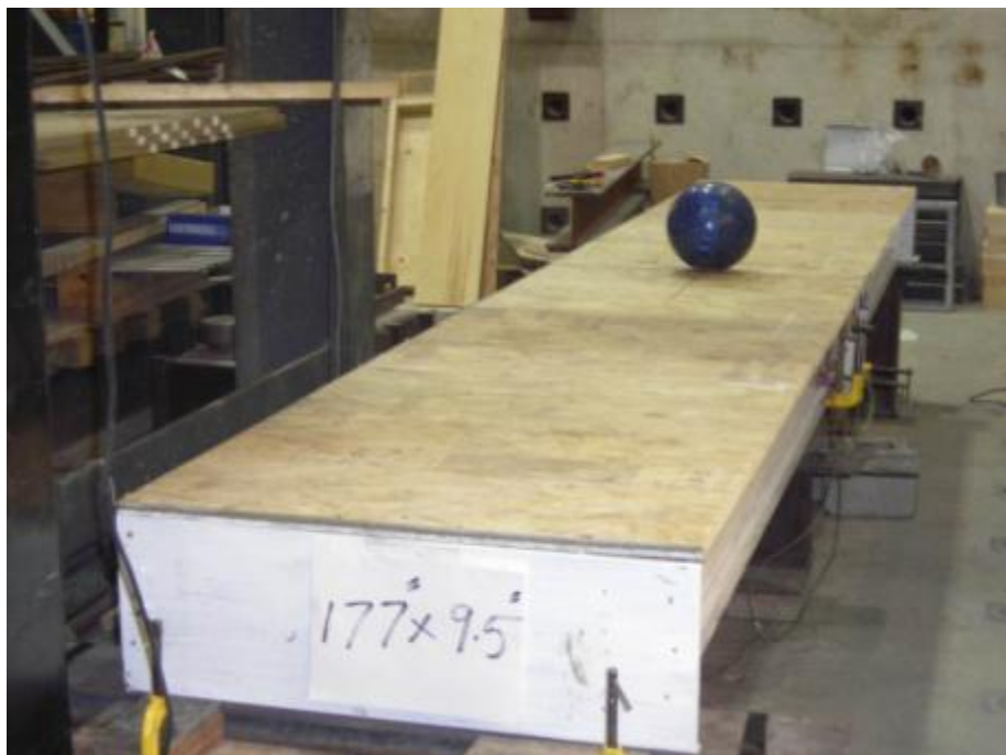
Figure 3.35: View of the bowling ball dropped from a height of 0.3 m over the iSPAN joist assembly with simply-supported framing
