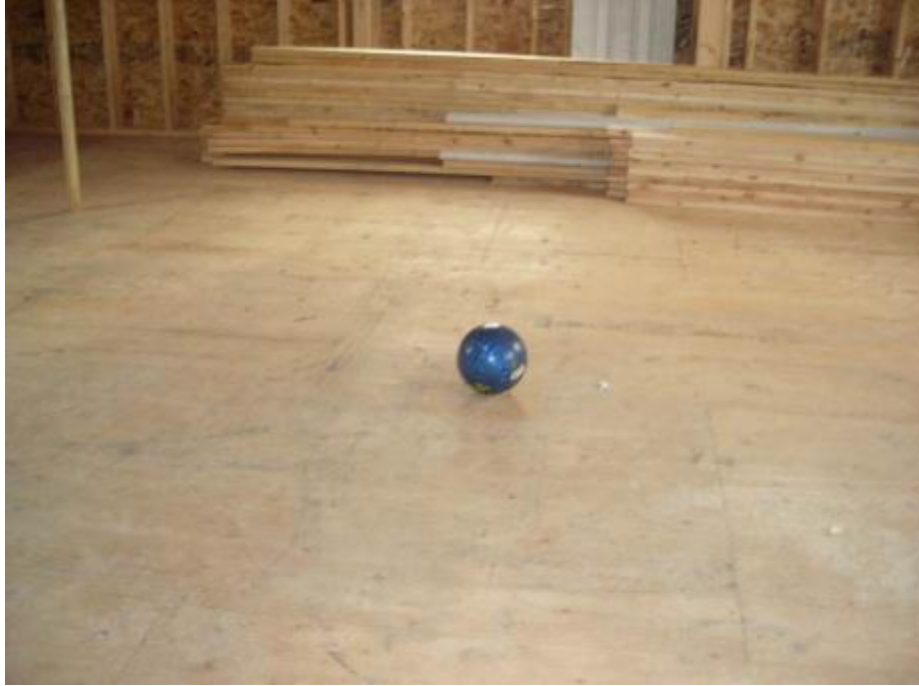
Figure 3.51: View of the bowling ball dropped from a height of 0.3 m over the floor in test site 2
