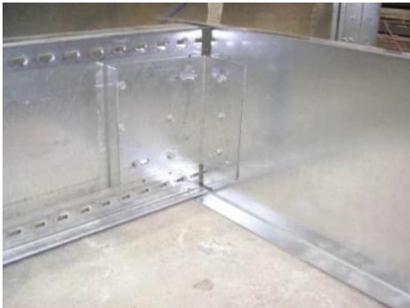
Figure 3.27: View of the clip angle attached to the joist and floor track of the simply-supported framing
