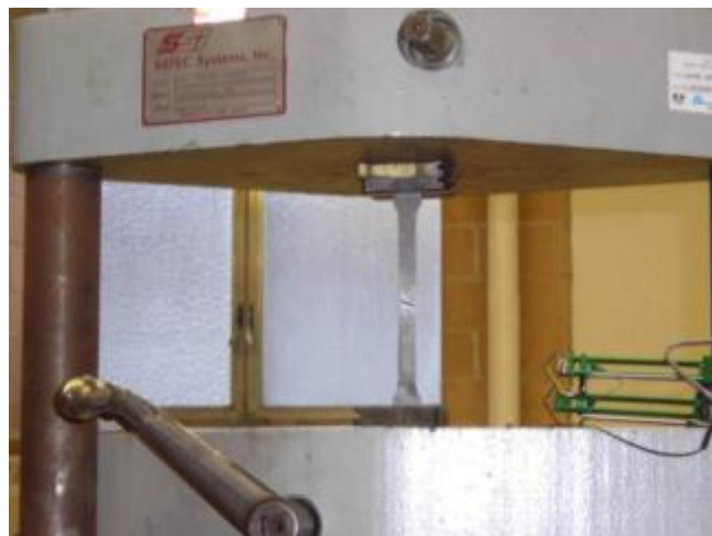
Figure 3.60: View of the coupon sample after failure in the tensile testing machine
