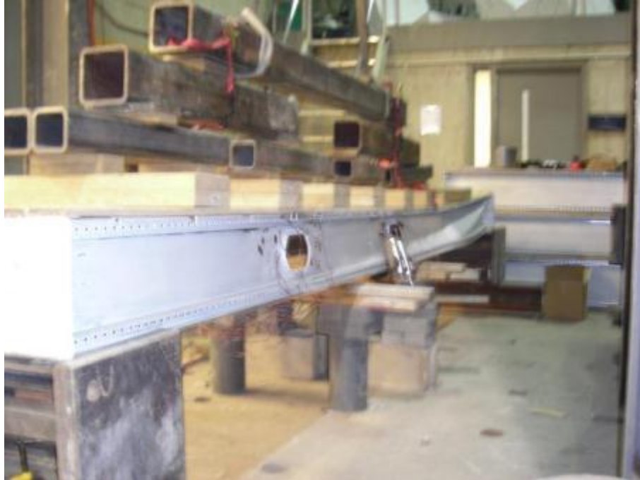
Figure E.28: View of lateral torsional buckling failure of the 254x4500 mm iSPAN joist assembly with web holes
