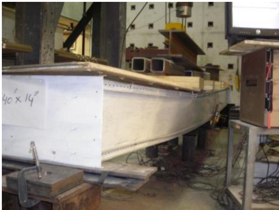
Figure E.22: View of lateral torsional buckling failure at the other side of the 356x6100 mm iSPAN joist assembly
