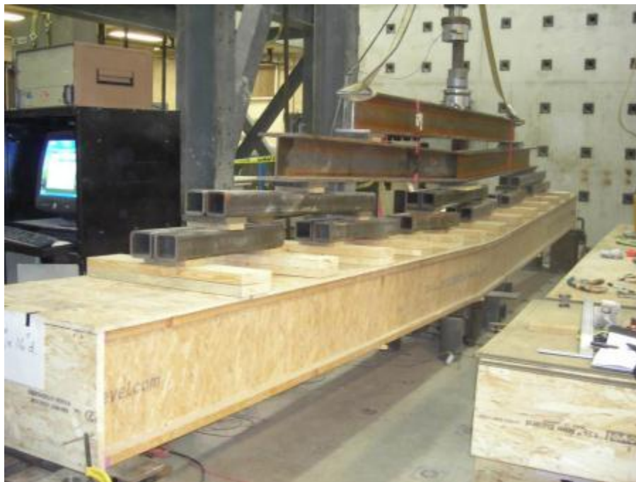
Figure 4.4: View of a wooden twin-joist assembly after pure flexural failure
