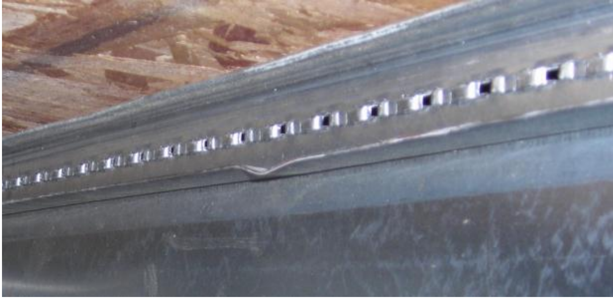
Figure 5.14: View of the experimental local buckling shape in the top flange lip of the 406x7950 iSPAN joist assembly
