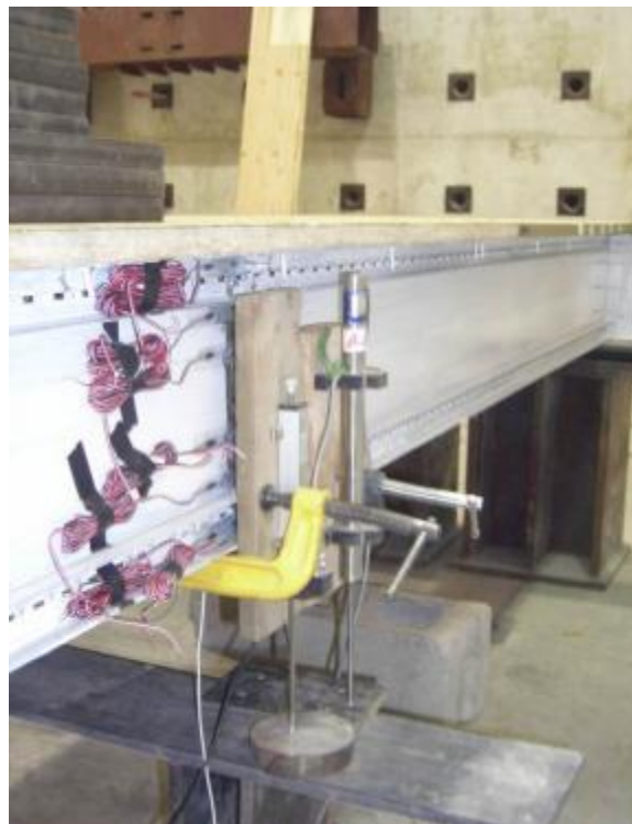
Figure 3.29: View of the LVDT attached to the iSPAN floor joist
