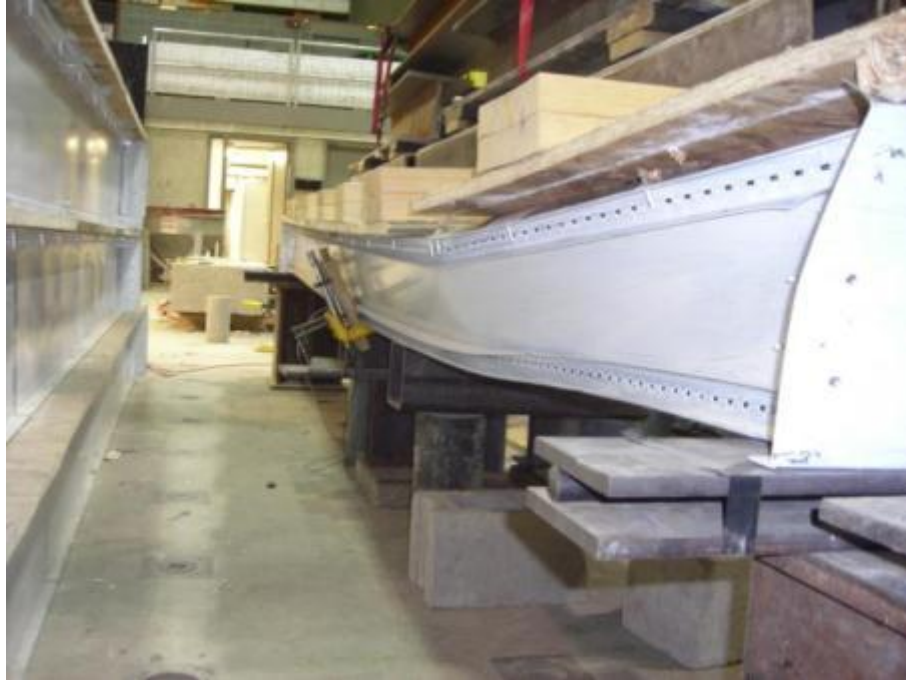
Figure E.15: View of lateral torsional buckling failure of the 241x4500 mm iSPAN joist assembly
