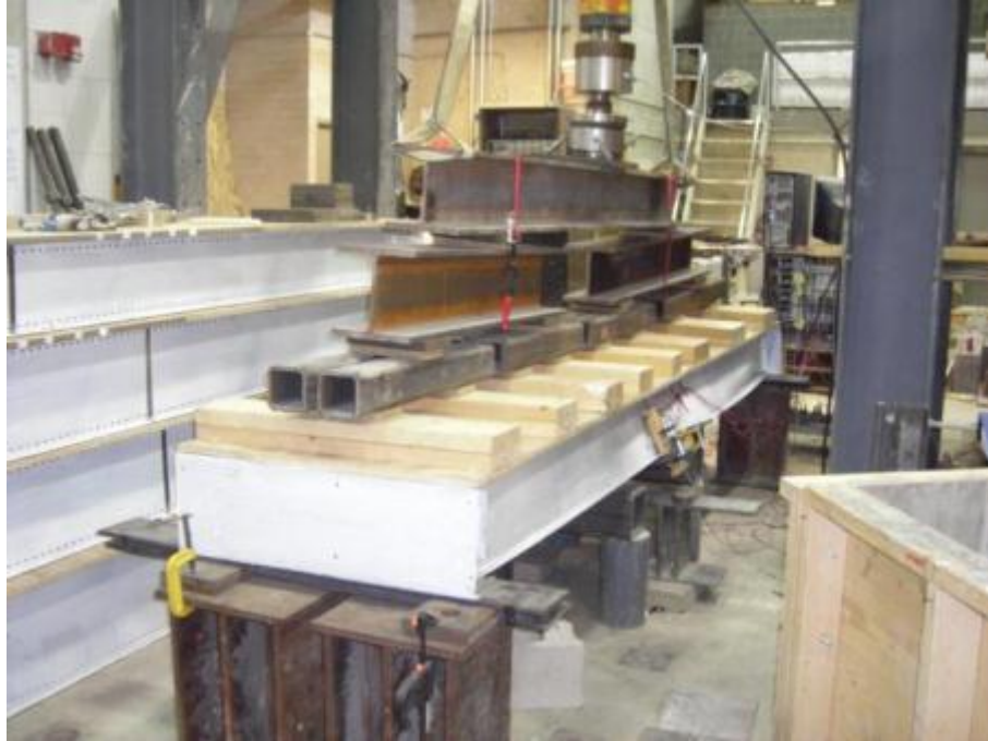
Figure E.13: View of the deformed shape at failure of the 241x3500 mm iSPAN joist assembly
