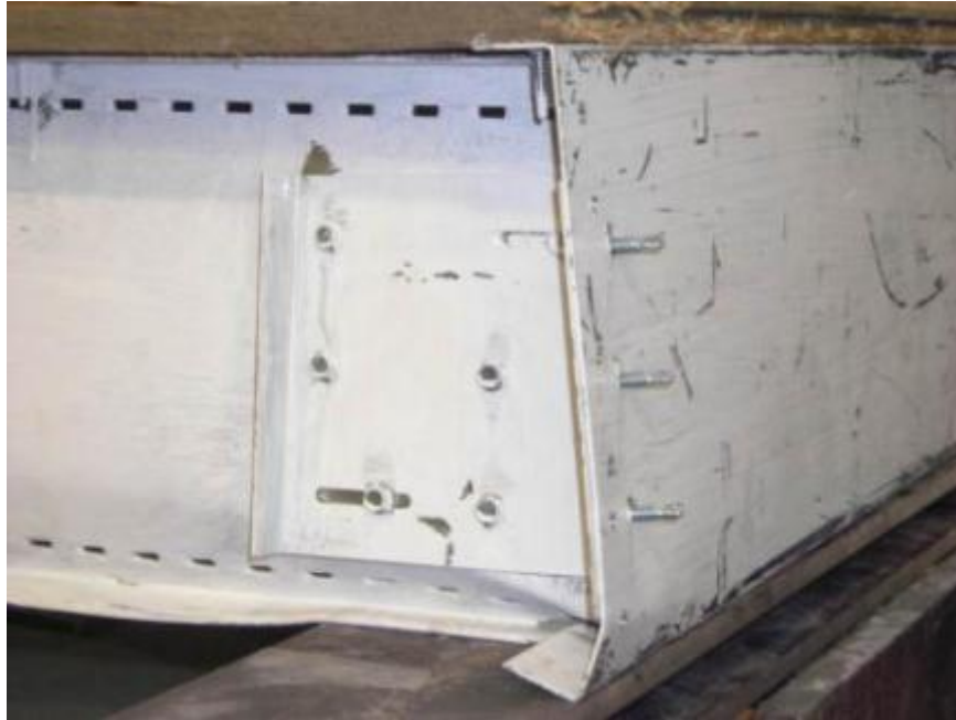
Figure 5.10: View of the experimental deformed shape of the 254x3500 mm iSPAN joist assembly showing web and track crippling at failure
