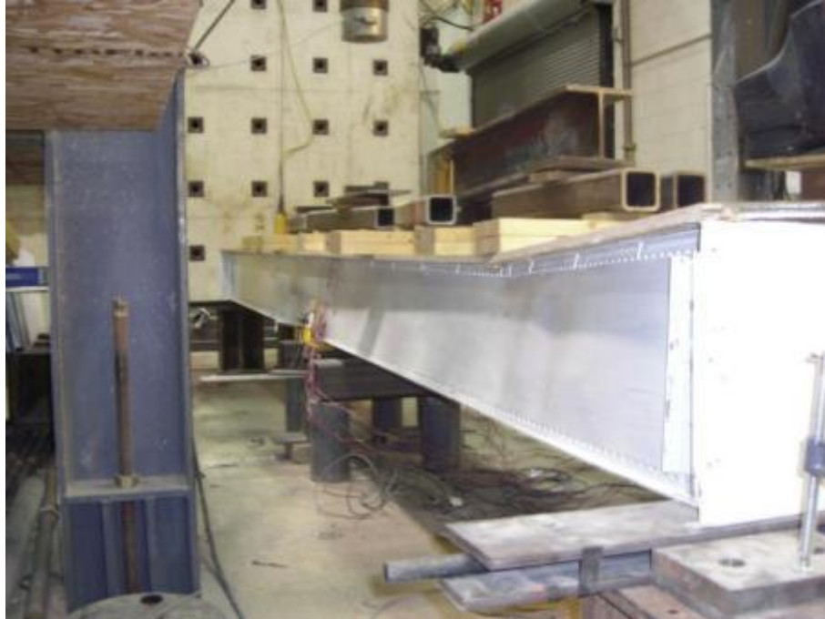
Figure E.21: View of lateral torsional buckling failure of the 356x6100 mm iSPAN joist assembly
