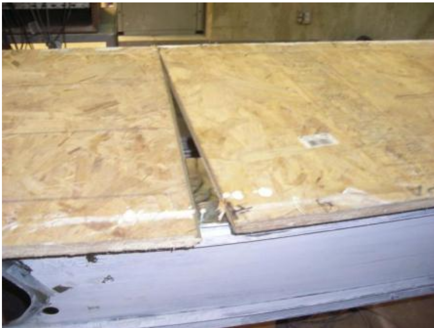
Figure E.33: Close-up view of the lateral torsional buckling failure of the joist and lateral separation of OSB sheets at mid-span region of the 302x5250 mm iSPAN joist assembly with holes
