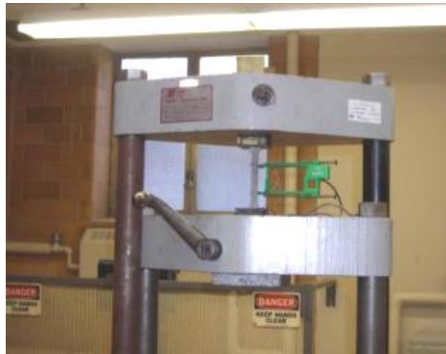
Figure 3.59: View of a typical setup for tensile coupon testing
