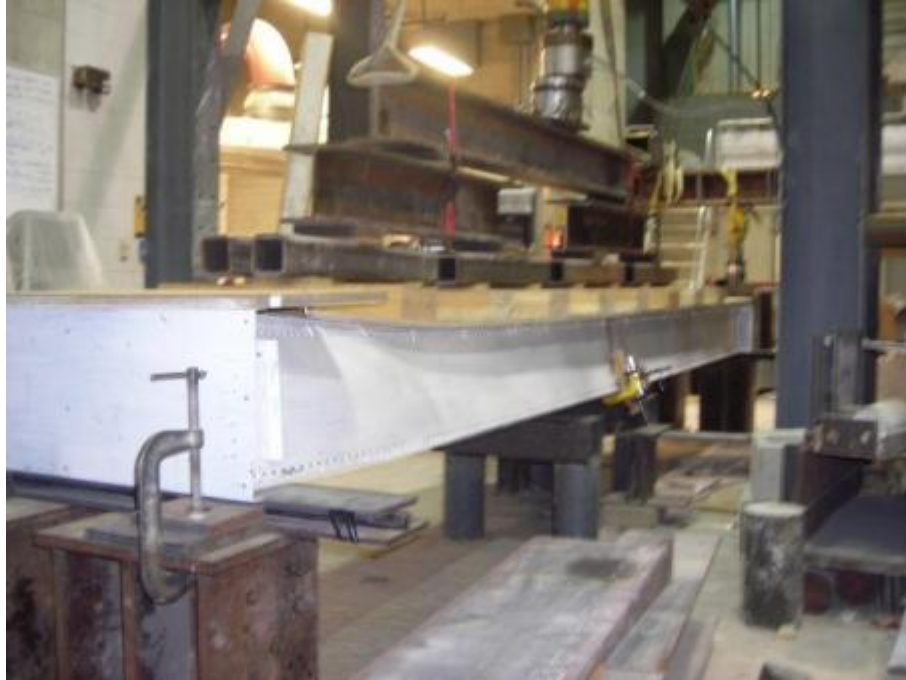
Figure E.19: View of lateral torsional buckling failure of the 302x5250 mm iSPAN joist assembly
