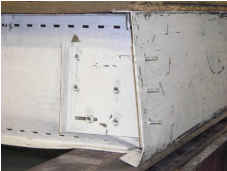
Figure 4.15: View of an iSPAN joist failed due to web crippling at support location
