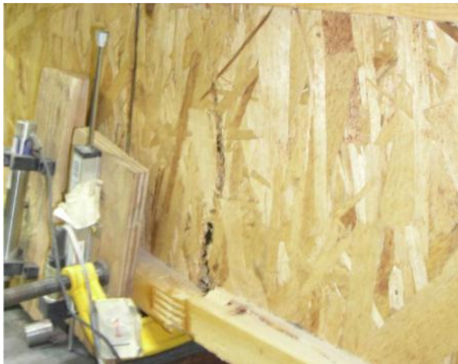
Figure E.8: Close-up view of the bending fracture of the bottom flange of web of the 302x5250 mm wooden joist assembly
