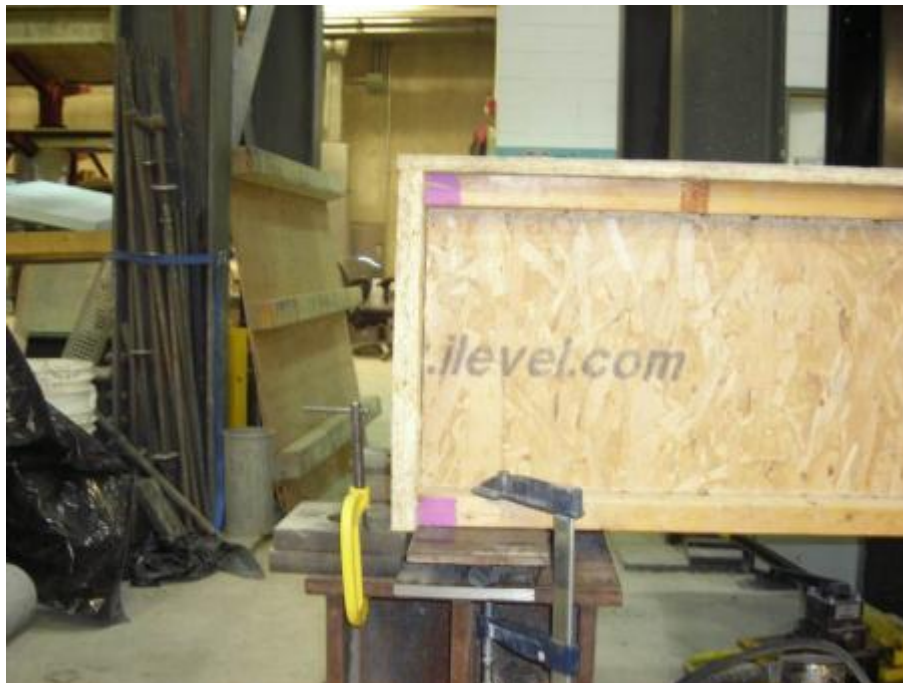
Figure 3.11: View of the clamping system at support of wooden I-joist assembly to avoid bouncy effect
