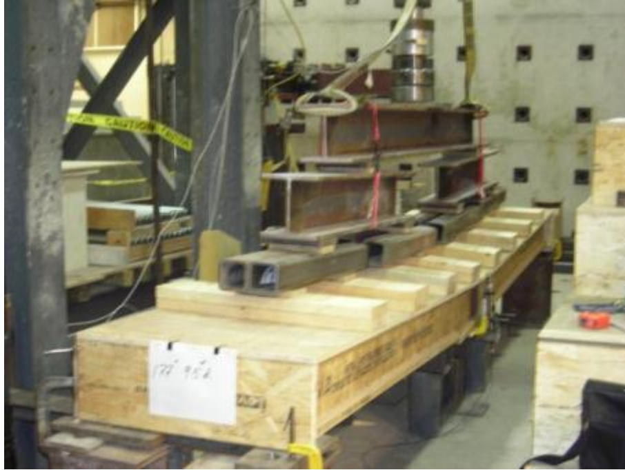
Figure E.3: View of deformed shape at failure of the 241x4500 mm wooden joist assembly
