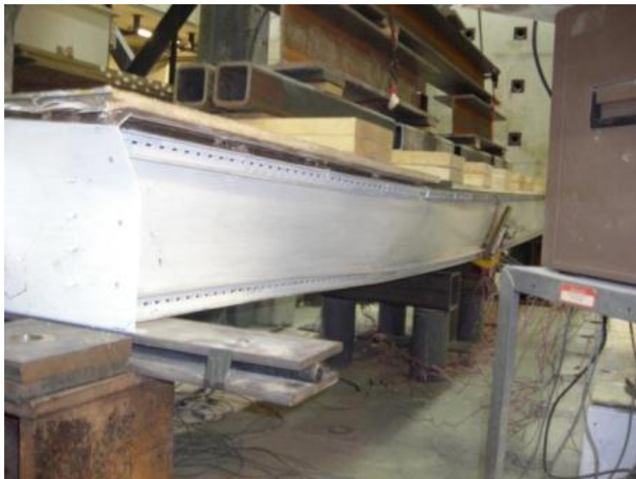
Figure E.18: Close-up view of lateral torsional buckling failure of 302x5000 mm iSPAN joist assembly along with crippling of the rim board over the support
