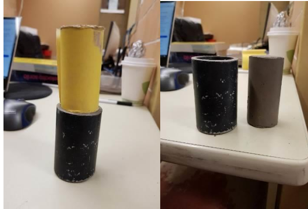
Figure 3-18 DMM triaxial sample extruding
