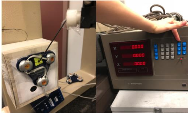
Figure 31 – Setting the origin of CMM measurements
