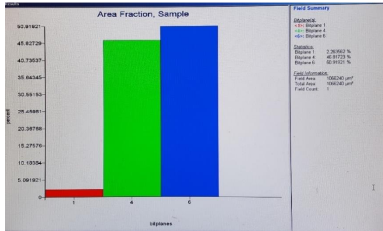
Figure 35: A generic results from Buehler Omnimet software for constituents fraction (Unidirectional laminate, image #14)
