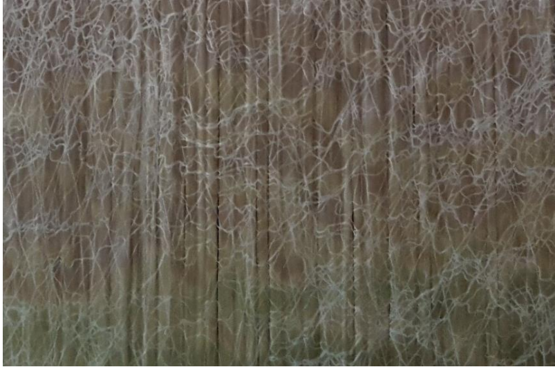
Figure 26: Unidirectional E-Glass ply sample with randomly distributed yarns to hold the UD fibers in place
