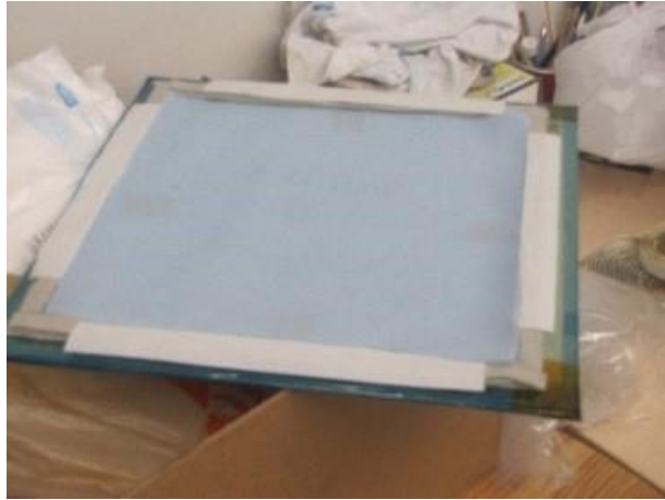
Figure 24: Base plate with peeling membrane
