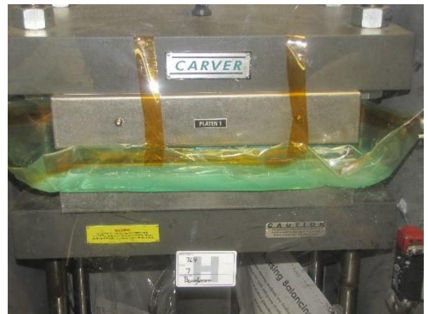
Figure 29: Mold Inside the membrane bag, loaded into the compression molding machine; before and after compression
