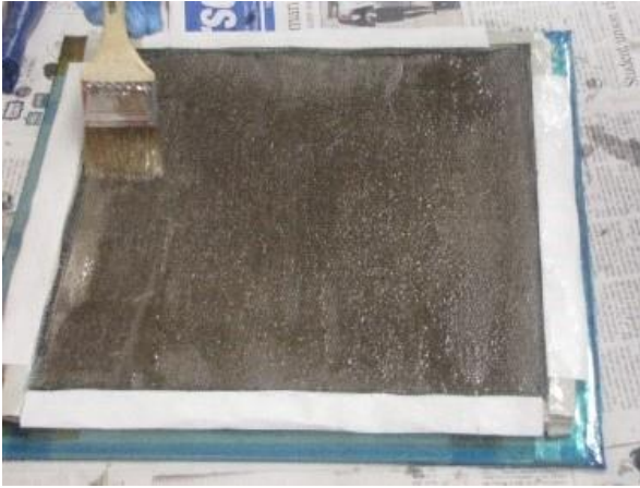
Figure 28: Spreading the matrix using a brush and then raking of resin using rigid roller upon fiber Sheets
