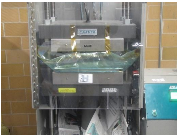
Figure 29: Mold Inside the membrane bag, loaded into the compression molding machine; before and after compression
