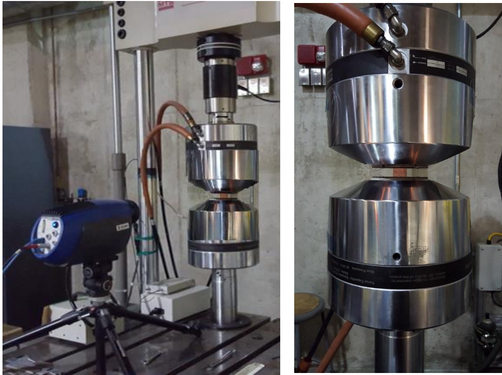
Figure 62: Compression-compression fatigue test set up; IR camera used in this study is shown in left figure.
