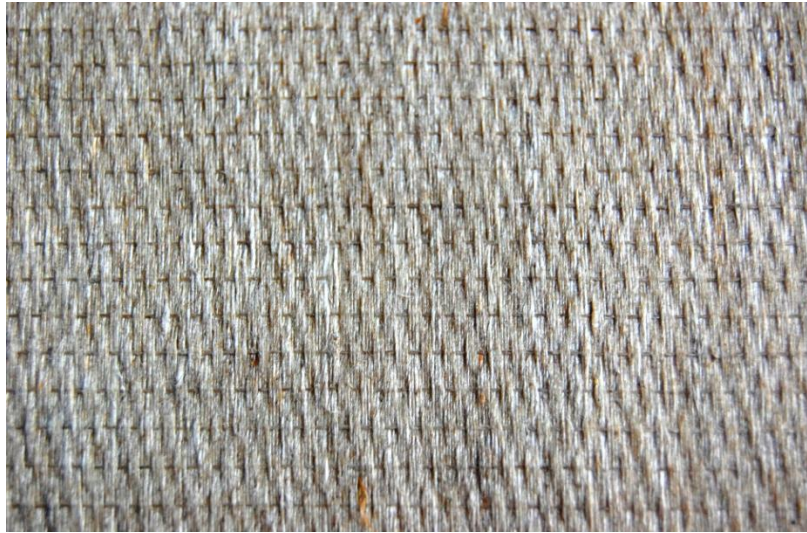
Figure 25: Lineo flax ply sample with yarn strands ratio 0^\circ : 90^\circ equal to 40 : 3
