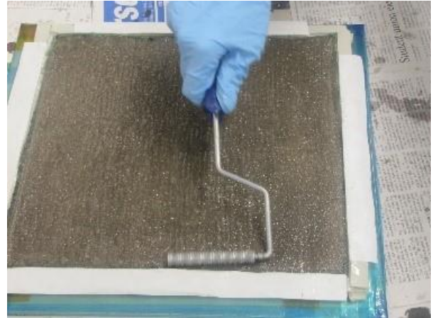
Figure 28: Spreading the matrix using a brush and then raking of resin using rigid roller upon fiber Sheets
