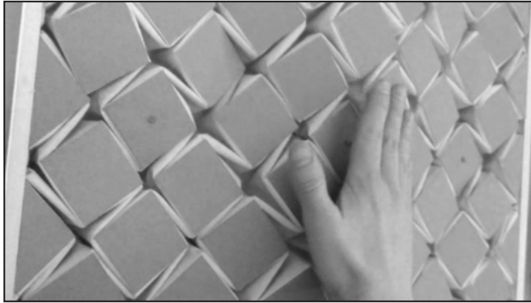
Fig. 41a Responsive surface controlled by light sensors
