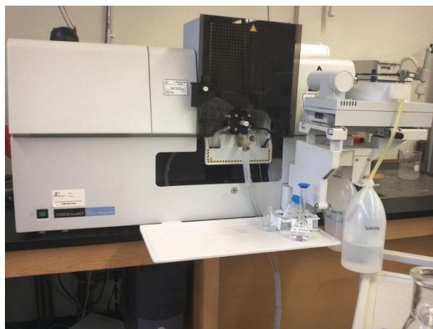
Fig. 2.7 A photograph of the atomic absorption spectrometer that was used to measure the concentration of GNPs in solutions.
