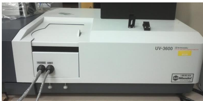
Fig. 2.4 A front view of the UV-NIR spectrophotometer used for the optical absorption measurement.
