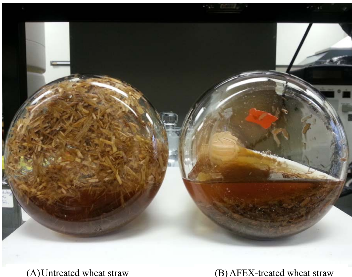
Figure 4-2. Wheat straw after 164 hours of hydrolysis with enzymes NS22086 and NS2218 at 47.5 °C.
