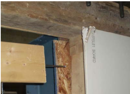
(c) Separation of OSB sheet and gypsum board from stud frame at top end
