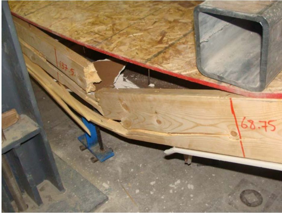
Figure 4.66 - Close-up view of the flexural failure of joist No. 5 in specimen SW-F-3
