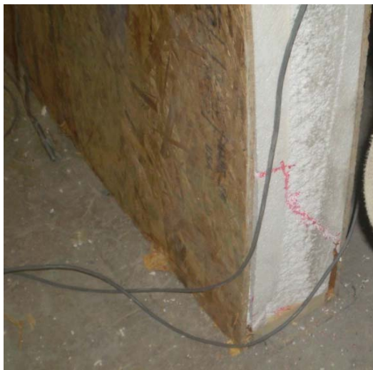
(c) Shear crack in foam at right side
