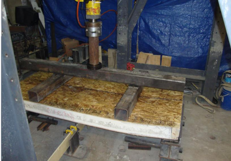
Figure 4.34 - View of the deflected shape of specimen SIP-F-2 after failure
