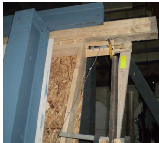
(b) Close-up view of the separation of OSB and drywall from the stud at top of wall
