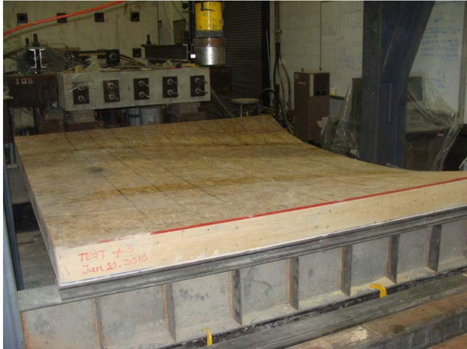
Figure 4.64 - View of the permanent deflected shape of specimen SW-F-3 after removing the loading system
