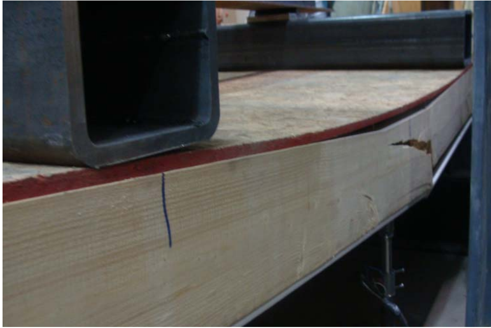
Figure 4.44 - Other view of the deflected shape and flexural failure at mid-span of first joist in specimen SW-F-1
