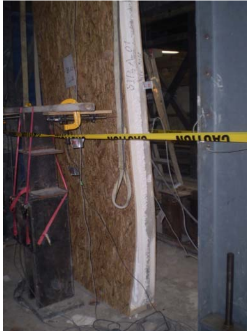
(b) Deformation and failure in specimen SIP-A-1
