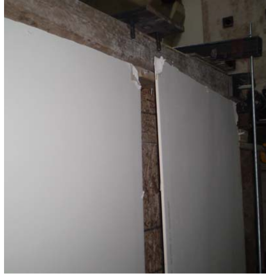
(b) Separation of dry wall from the stud
