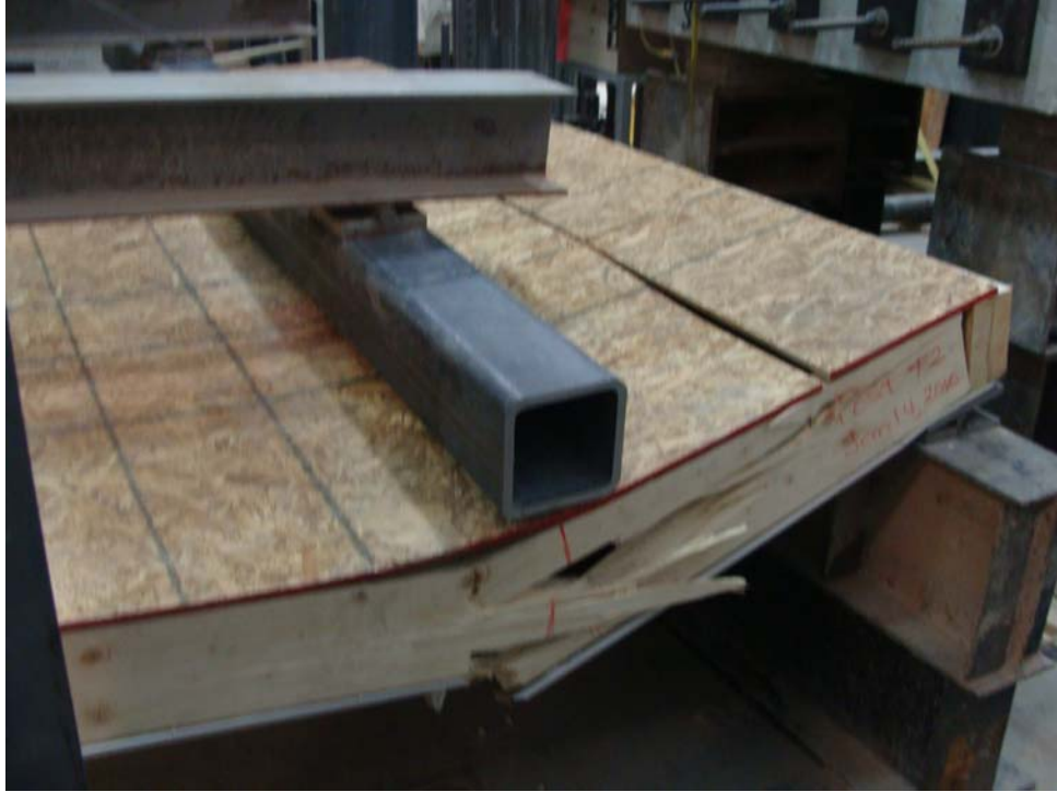
Figure 4.52 - Close-up view of the deflected shape of specimen SW-F-2 after failure
