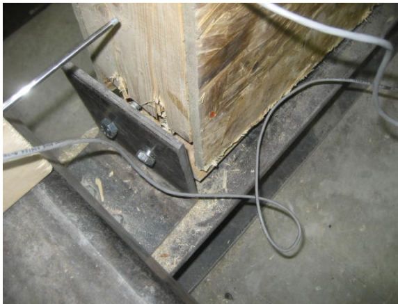
(a) Tearing and cracking of end lumber at the bottom of panel
