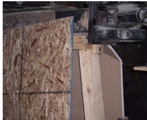
(b) Separation of OSB sheet from stud frame
