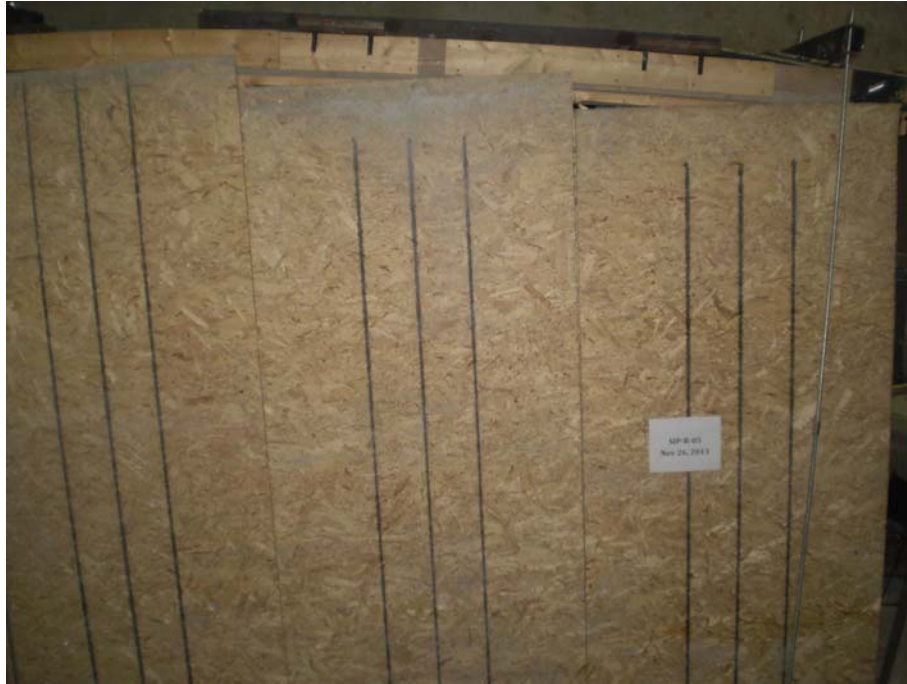
(c) Deformation at failure of specimen SIP-R-4
