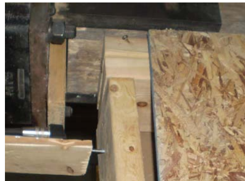
(d) Bending of the nail and OSB crushing in nail connection
