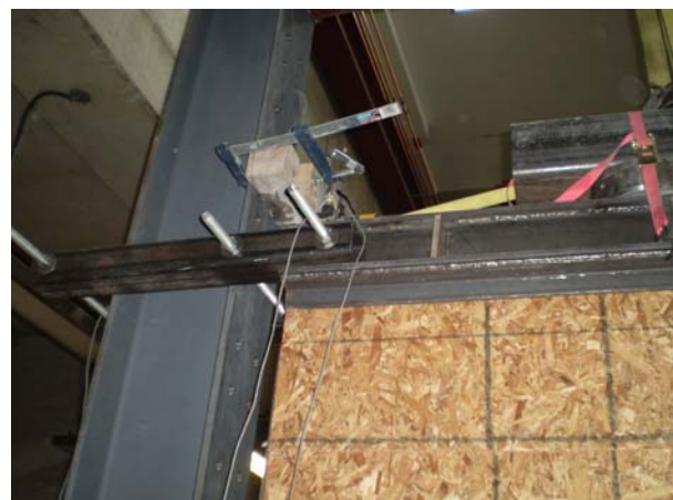
Figure 3.18 – View of POTs locations in panel for stud wall specimen
