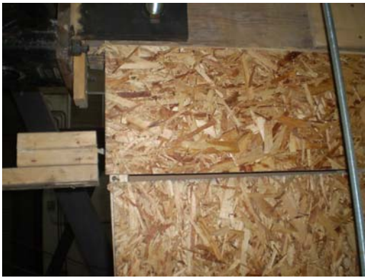
(a) Separation of OSB sheet on joint
