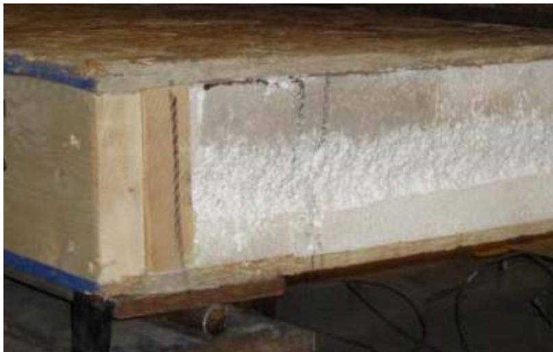
Figure 4.39 - Close-up views of specimen SIP-F-3 showing horizontal shear failure at the top foam-OSB interface
