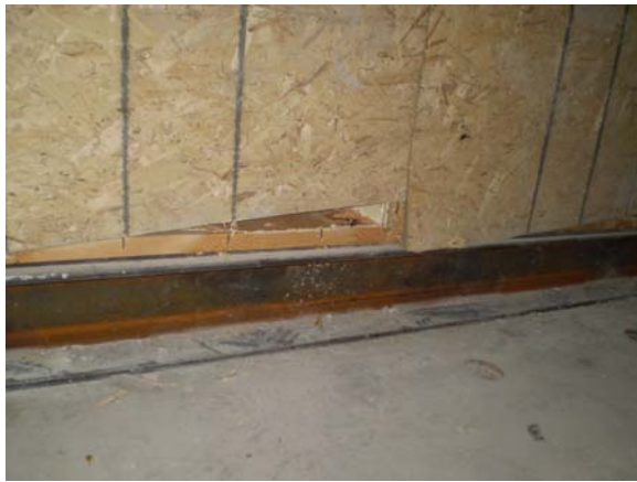
(b) Bending of nail and crushing of OSB sheet at nail location
