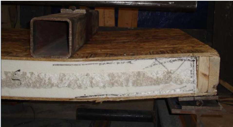
Figure 4.35 - Close-up views of the failure mode of specimen SIP-F-2
