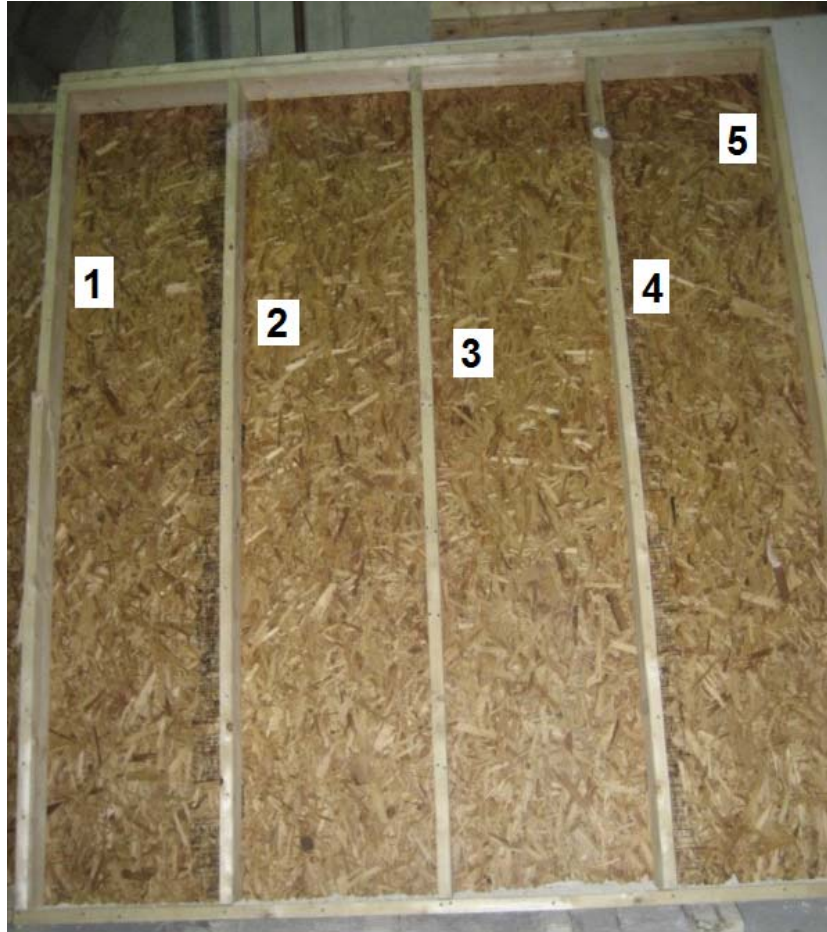
Figure 4.46 - View of the joists after removing the drywall of specimen SW-F-1
