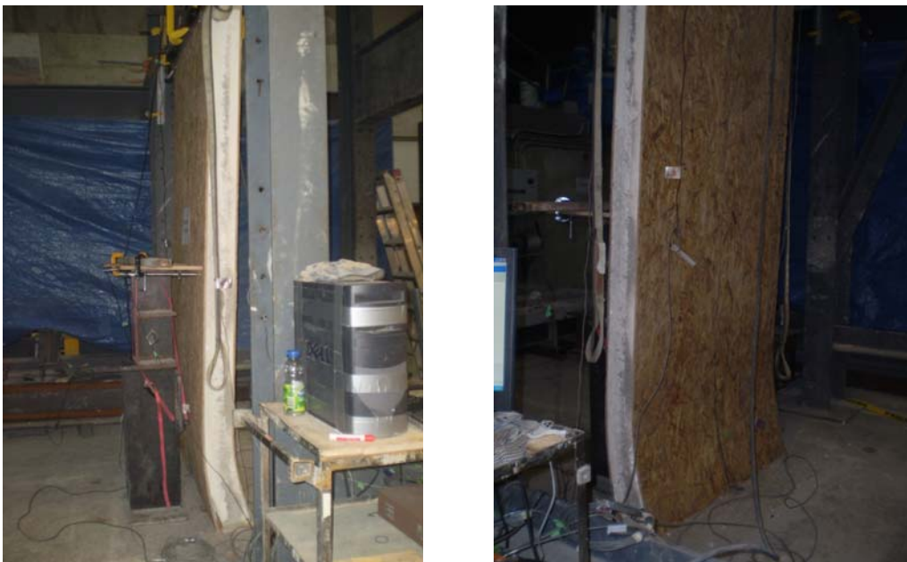
Figure 4.12 - Views of the deformed shape of the wall SIP-A-3 after failure
