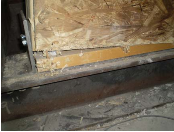
(a) Uplift at the bottom and panel crushing
