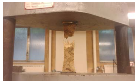
(b) Failure after tension test
