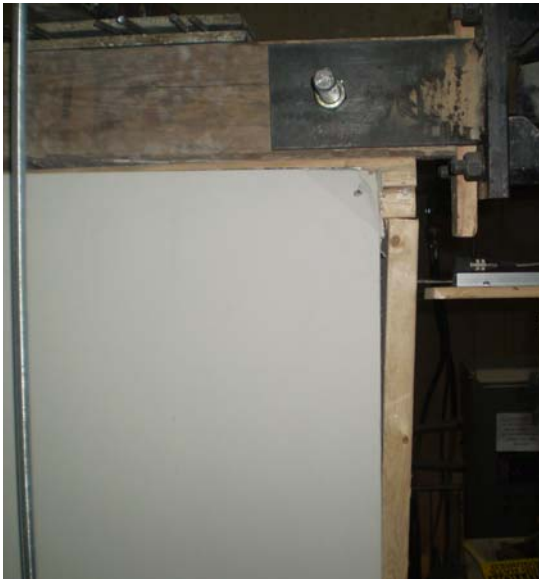
(c) Shear deformation of the wall at the drywall side
