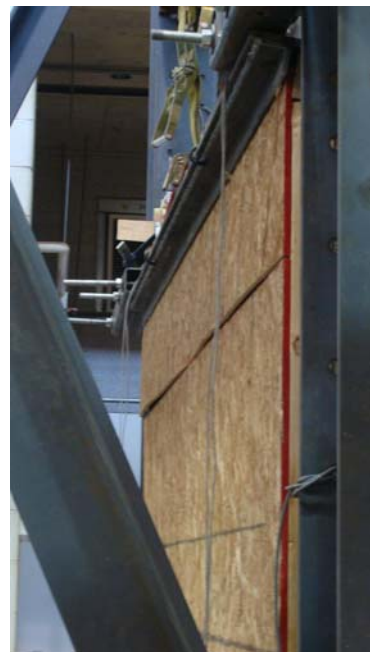
(b) View of OSB sheet joint opening in left right side of the wall
