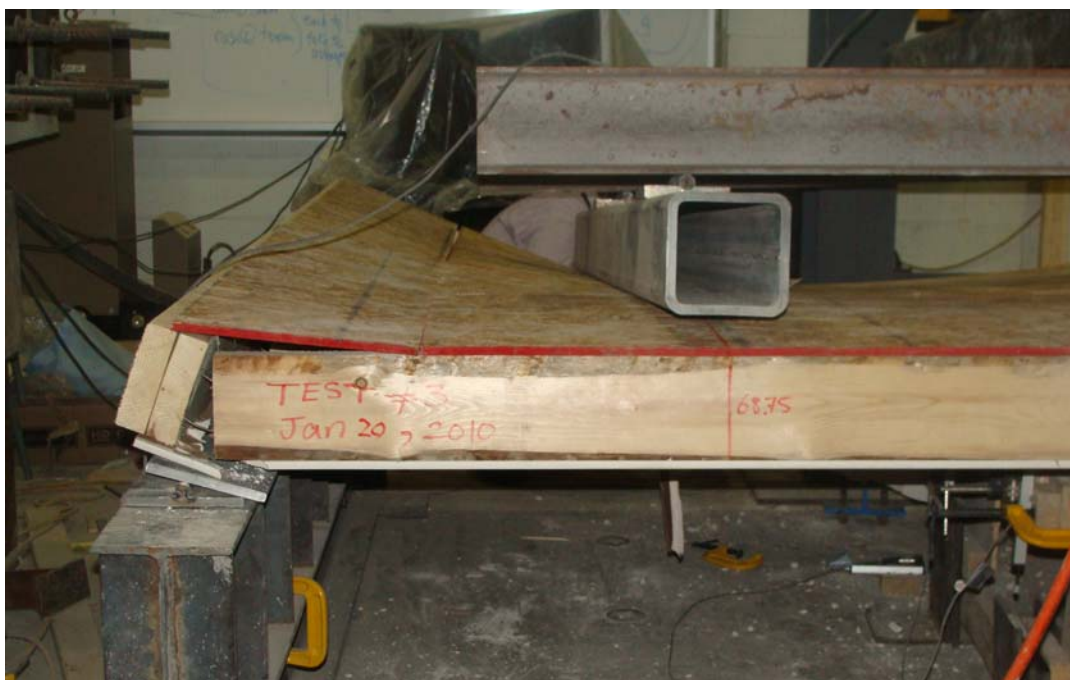
Figure 4.70 - Close-up view of the bearing rotation as well as end stud and OSB sheet separation from joist No. 1 of specimen SW-F-3 after failure
