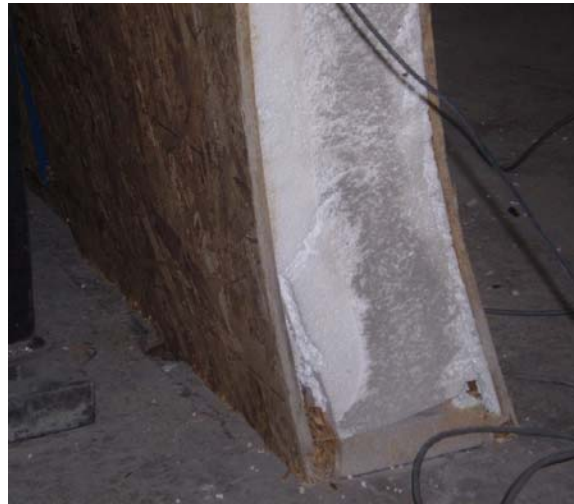
(b) Foam-OSB debonding and shear crack in foam
