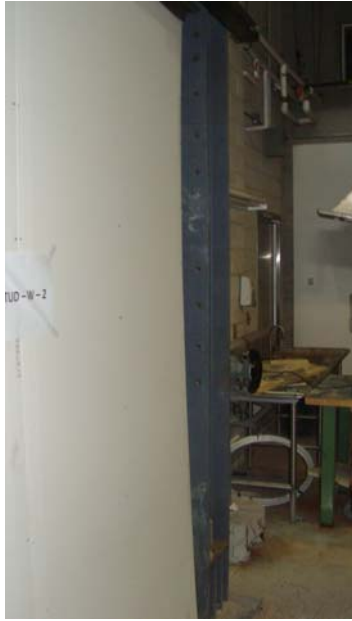
(a) Lateral deflected shape of the drywall side of the wall
