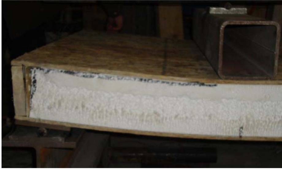
Figure 4.31 - Close-up view of specimen SIP-F-1 showing horizontal shear failure at the top foam-OSB interface
