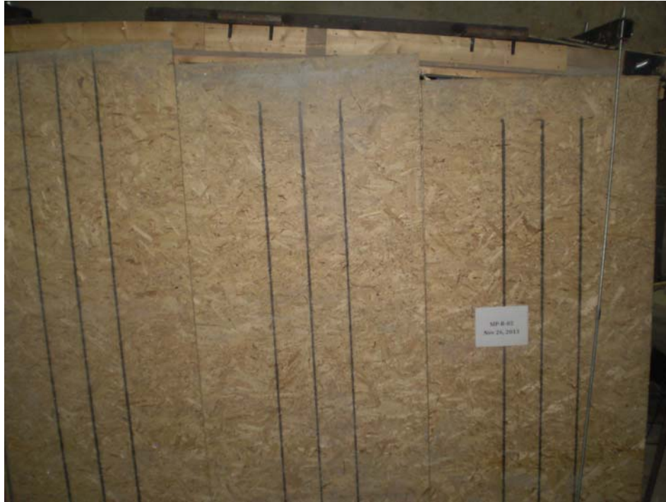
Figure 4.92 – Global failure of specimen SIP-R-4 under racking load showing global shear deformation and relation shear rotation of SIP segments at spline connection
