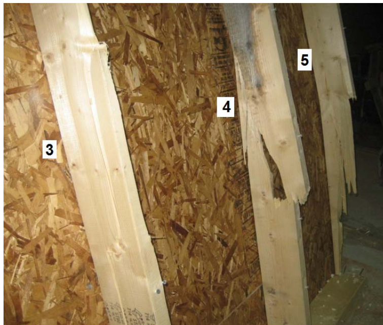
Figure 4.57 - Close-up view of failure of joists No. 3, 4 and 5 of specimen SW-F-2 after failure
