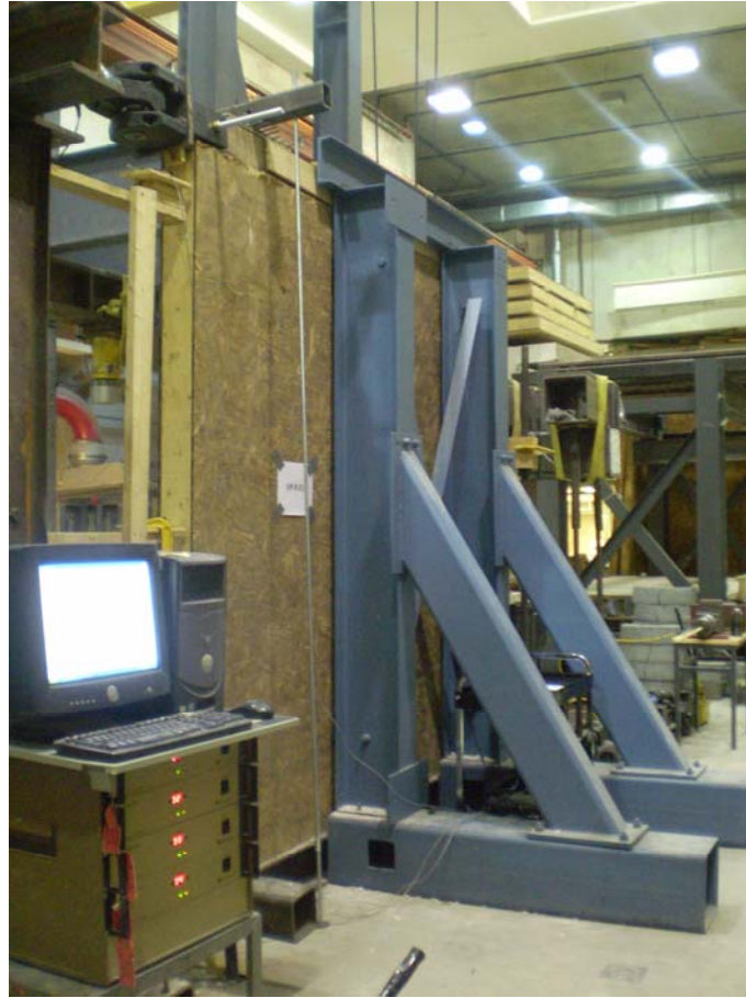
Figure 3.31 – Typical test setup for monotonic and cyclic lateral load testing on the SIP wall
