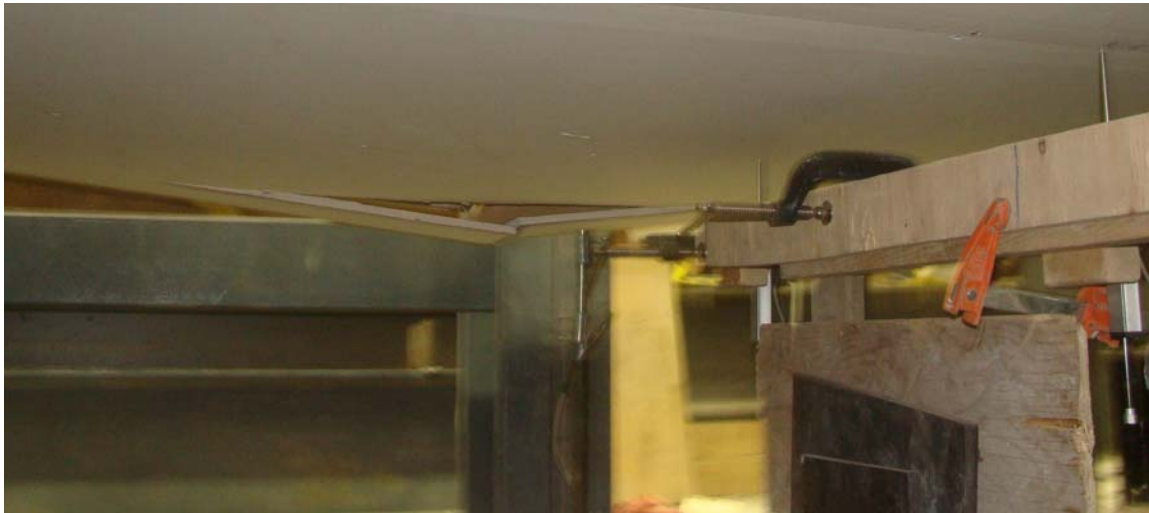
Figure 4.45 - Close-up view from underside of the first joist showing longitudinal and transverse flexural cracks in the drywall of SW-F-1
