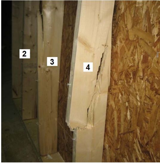
Figure 4.58 - Close-up view of failure in joist failure of No. 3 and 4 of specimen SW-F-2
