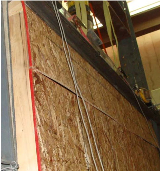
(b) View of the OSB sheet joint widening from left side sheet joint
