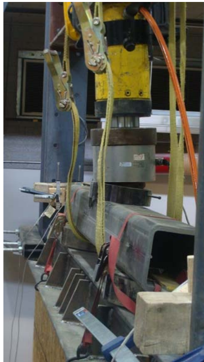
Figure 4.22 - Rotation of the top rail at failure of stud wall specimen SW-A-2
