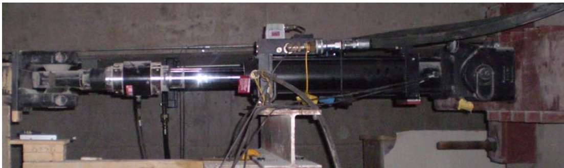
Figure 3.13 – View of hydraulic actuator for racking and cyclic loading
