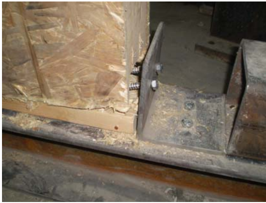
(a) Uplift, tearing and cracking of lumber at the bottom of the panel
