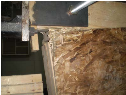
(c) Crushing OSB sheet at top of the panel
