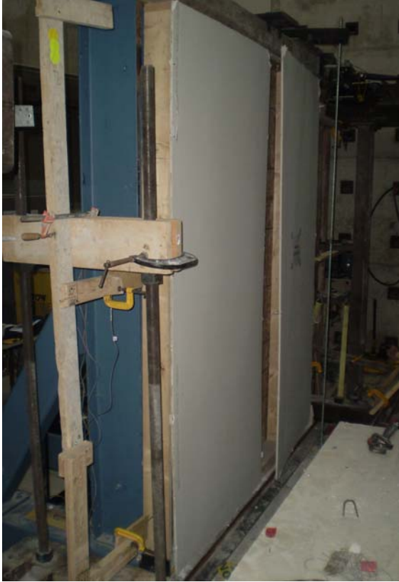
(a) Separation of dry wall
