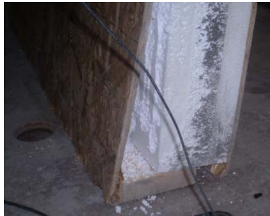
(b) Foam-OSB debonding and OSB crushing
