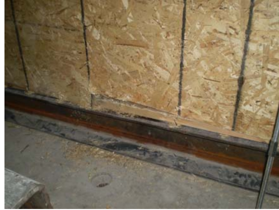
(b) Bending of nail and crushing of OSB sheet in nail location
