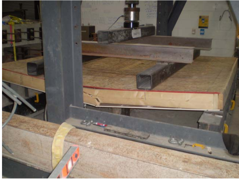
(b) Deformation and failure of specimen SW-F-1
