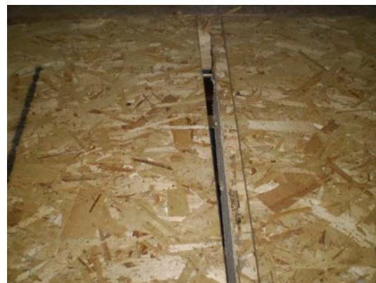
(b) OSB and spline separation at the middle of the panel
