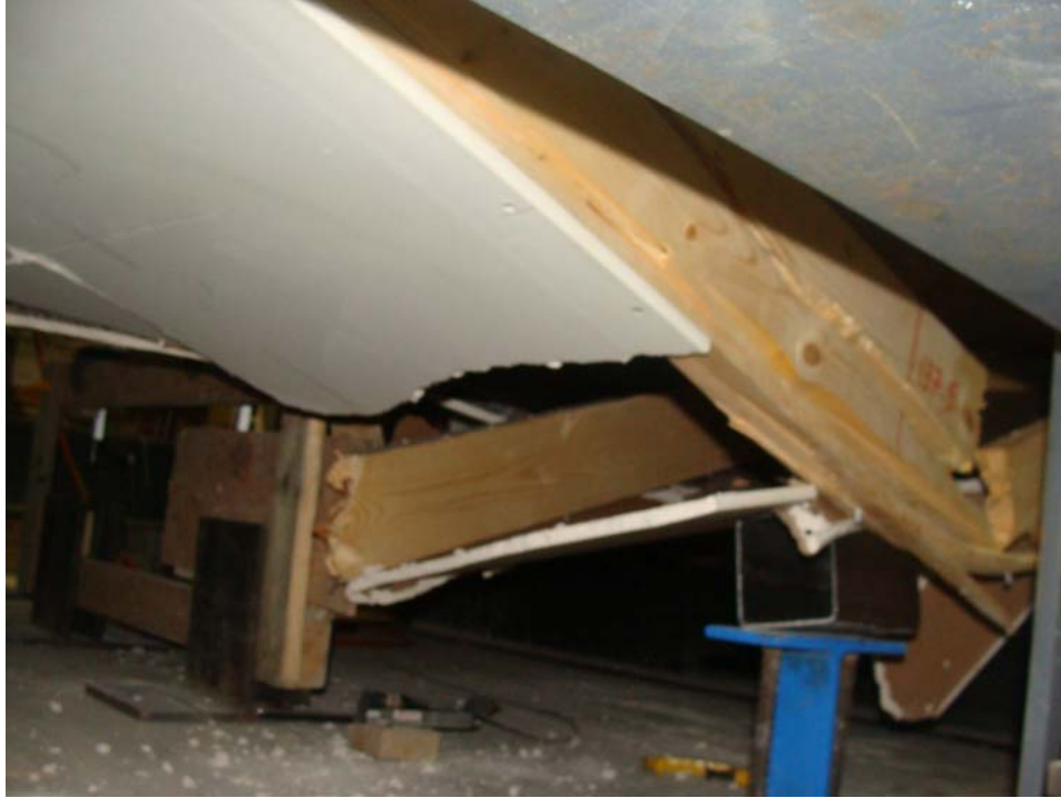
Figure 4.68 - Close-up view of the flexural failure of joists No. 4 and 5 and well as drywall break in specimen SW-F-3
