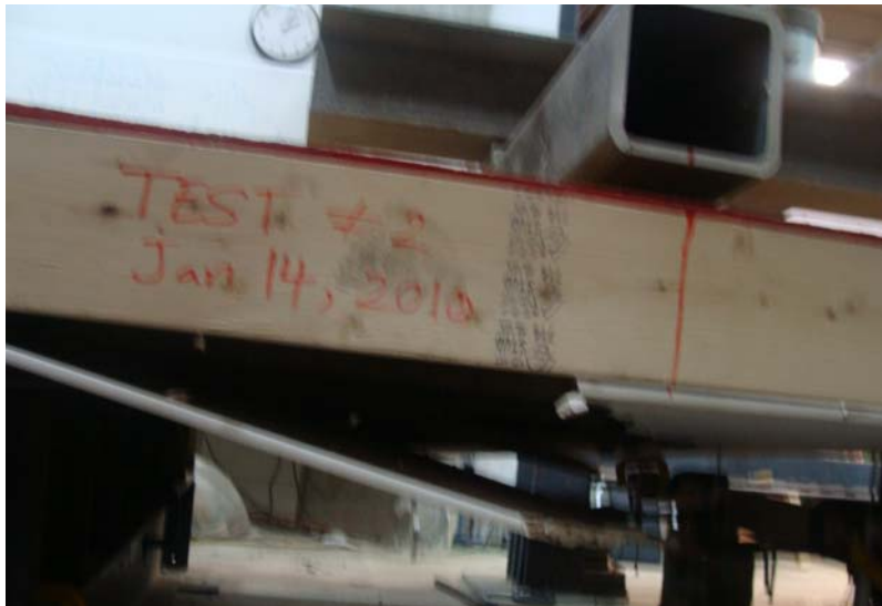
Figure 4.55 - View of drywall break at the quarter point of joist No. 1 of specimen SW-F-2
