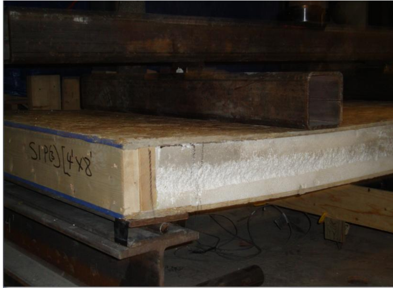
Figure 4.38 - View of the deflected shape of specimen SIP-F-3 after failure
