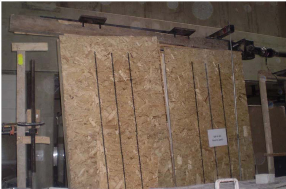
(c) Deformation at failure of specimen SIP-C-1
