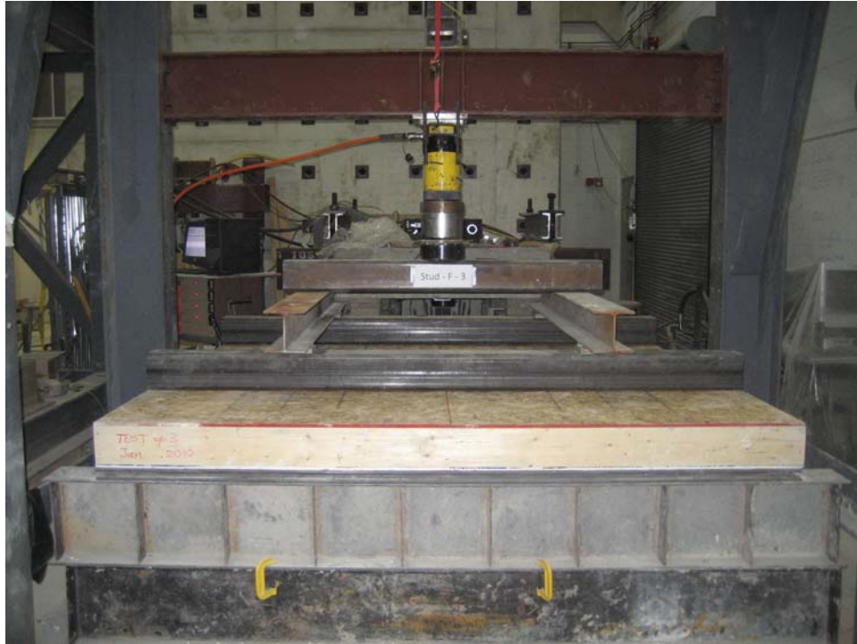
Figure 3.36 – Typical test setup of flexure for stud panel specimen
