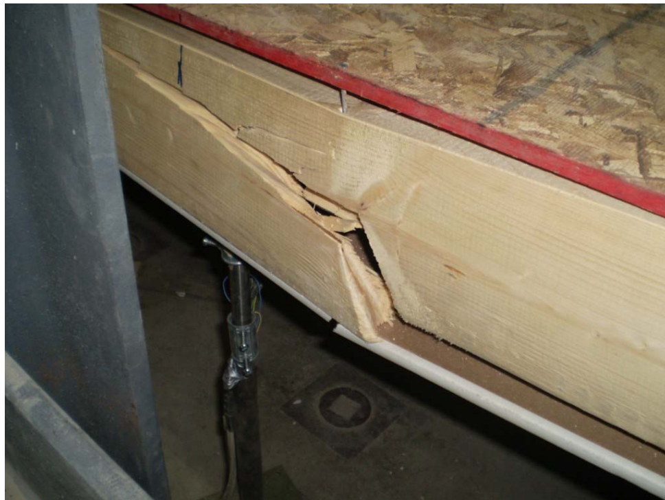
Figure 4.43 - Close-up view of the flexural failure pattern in the first joist at end of specimen SW-F-1
