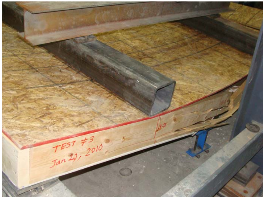
Figure 4.65 - View of the flexural failure and deformation of joist No. 5 of specimen SW-F-3 after failure
