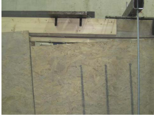
(c) Separation top plate from OSB
