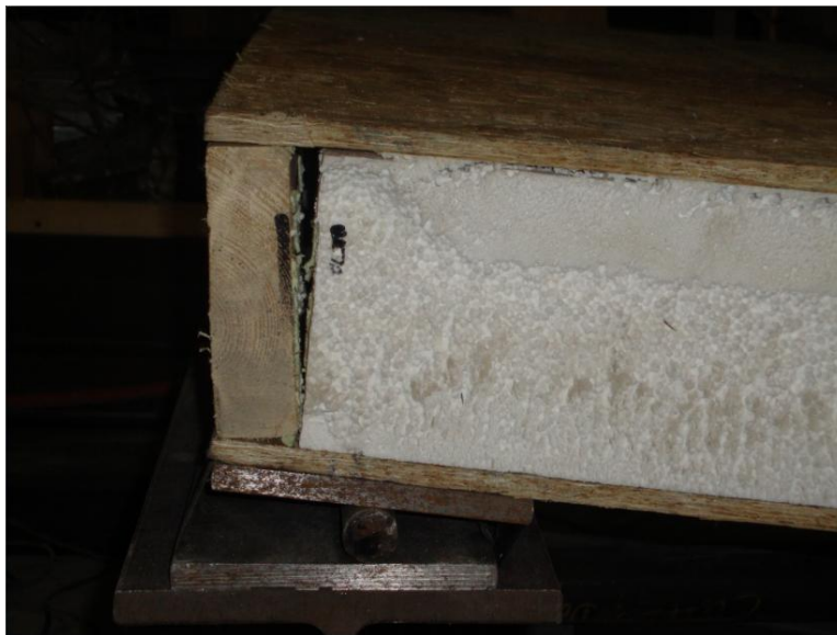
Figure 4.30 - View of the deflected shape of specimen SIP-F-1 at support after failure
