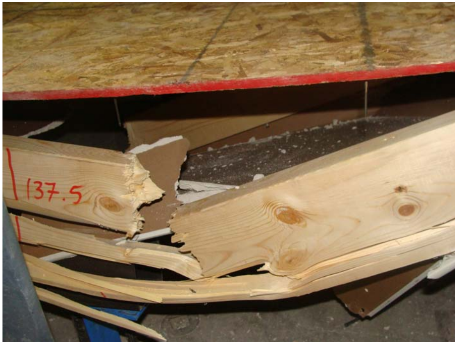
Figure 4.67 - Front view of the flexural failure of joist No. 5 in specimen SW-F-3
