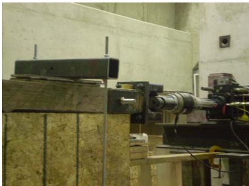
(a) Boundary condition on top of wall
