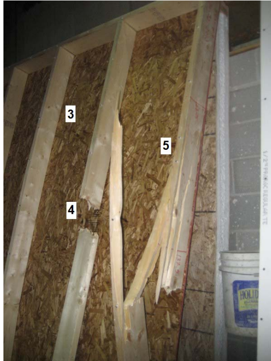
Figure 4.72 - Close-up view of the failure in joists No. 4 and 5 in specimen SW-F-3 after removing the drywall
