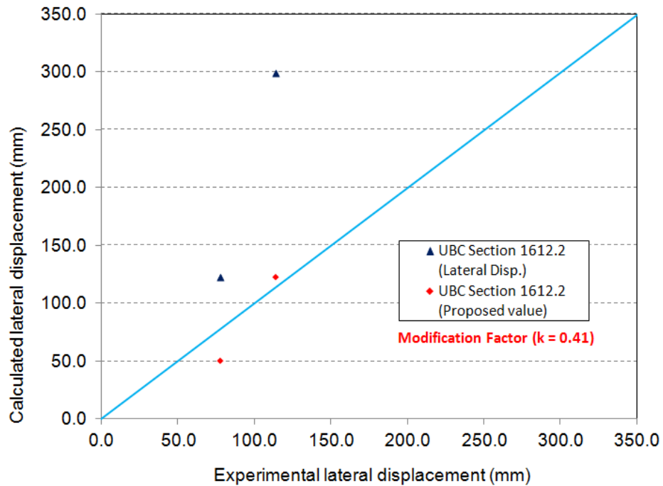
Figure 6.17 – Correlation between the monotonic lateral displacement obtained experimentally and that obtained using UBC Section 1612.2 along with the values using the proposed modification factor for racking loading on SIP walls
