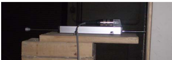
Figure 3.17 – View of potentiometer used in this study
