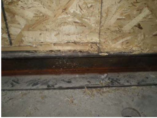
(c) Rotation of OSB sheet, nail bending and OSB crushing at nail location (d) Separation of lumbers at connection at top of the panel
