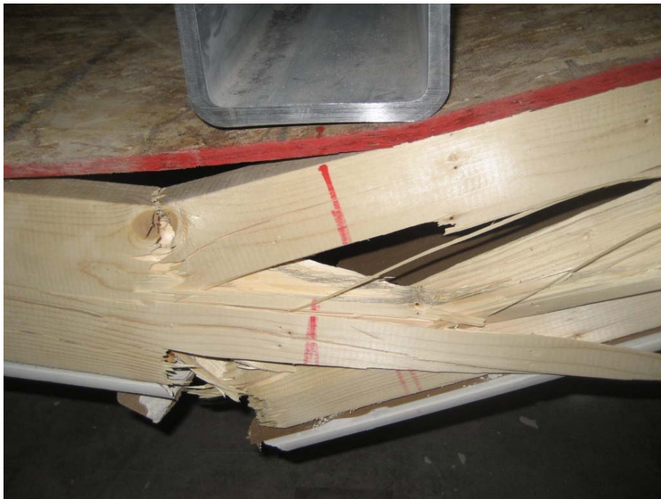
Figure 4.53 - Close-up view of the flexural failure at the quarter point of joist No. 5 of specimen SW-F-2
