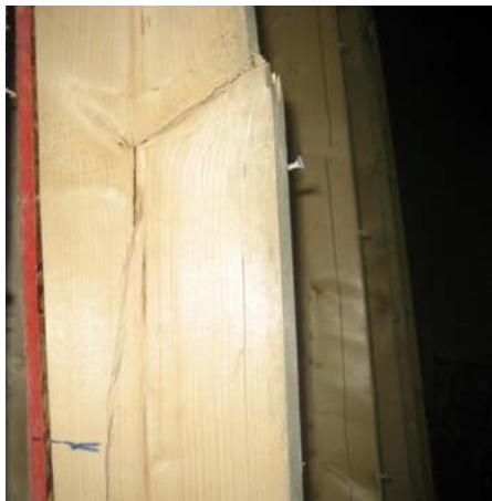
Figure 4.47 - Close-up view of the flexural failure longitudinal in joist No. 1 of specimen SW-F-1
