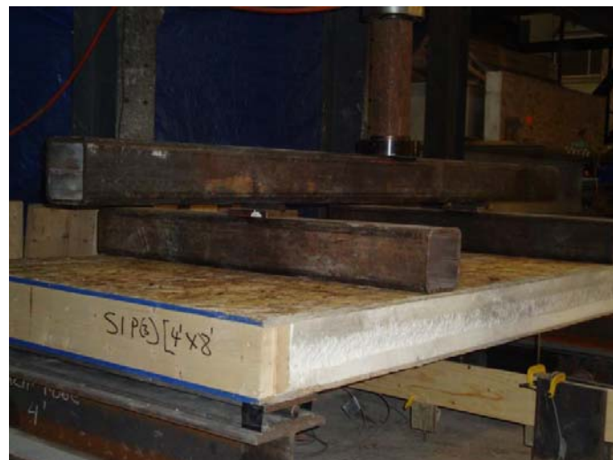
Figure 3.21 – Typical test setup for flexure of the SIP floor
