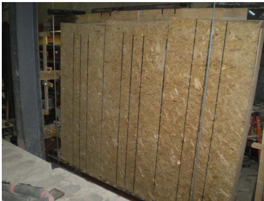
Figure 4.110 – Global failure of specimen SIP-C-4 under cyclic loading showing global shear deformation and relation shear rotation of SIP segments at spline connection
