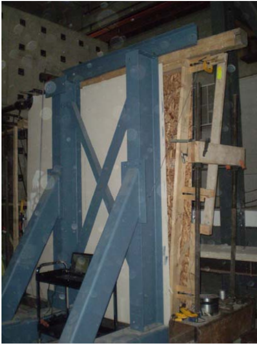
(a) Large shear deformation on the right side of the wall
