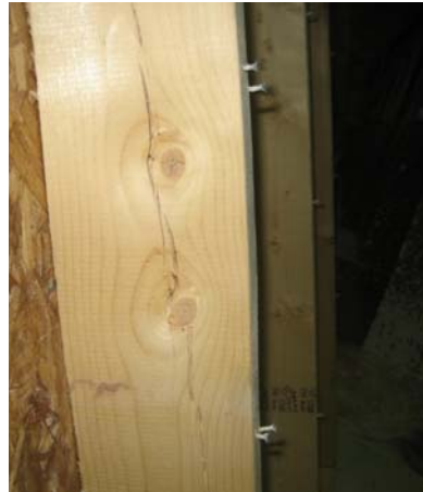
Figure 4.48 - Close-up view of crack in joist No. 2 of specimen SW-F-1
