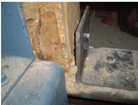
(a) Uplift at the bottom and lumber cracking at nail location
