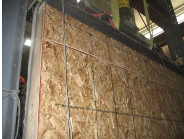
(b) View of deformation and failure of specimen SW-A-1
