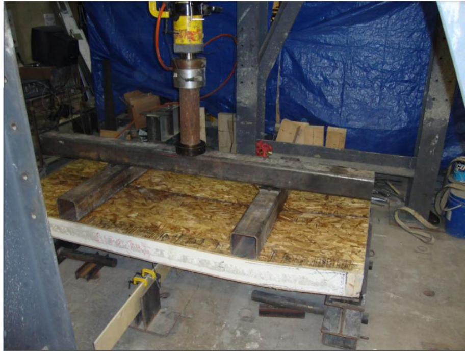
(b) Deformation and failure in specimen SIP-F-1
