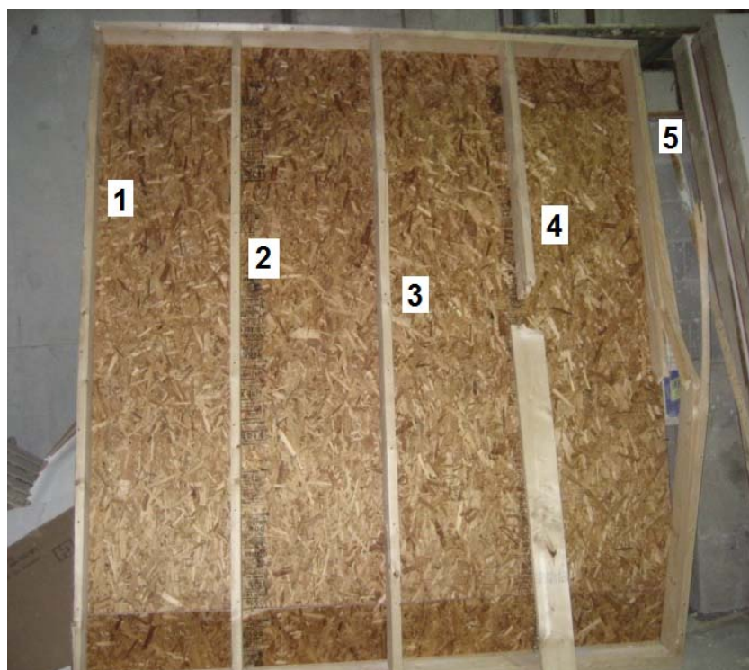
Figure 4.71 - View of the joists after removing the drywall of specimen SW-F-3
