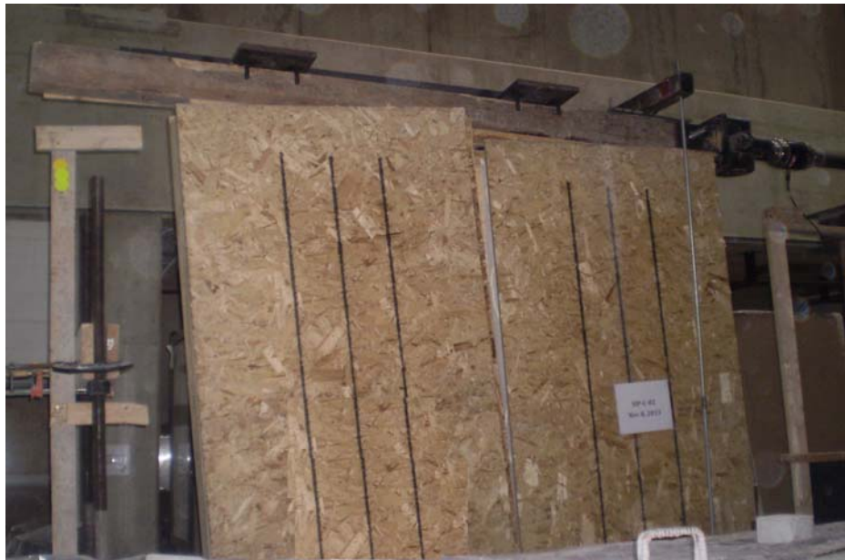
Figure 4.107 – Global failure of specimen SIP-C-1 under cyclic loading showing global shear deformation and relation shear rotation of SIP segments at spline connection
