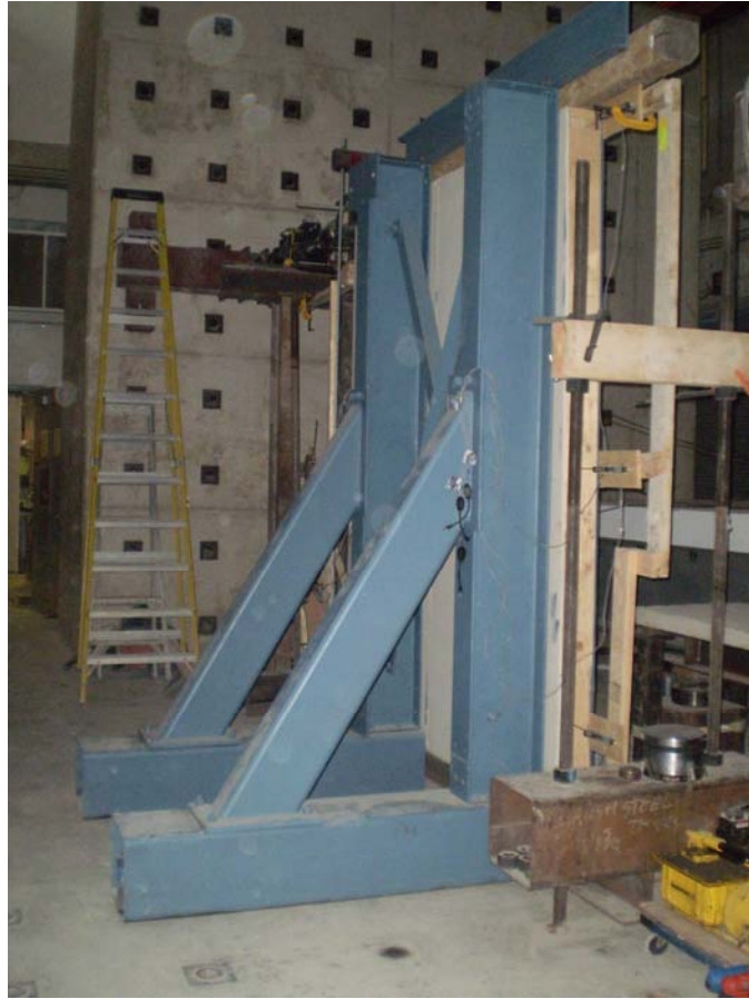
Figure 3.44 – Typical test setup of monotonic and cyclic lateral load for the stud wall
