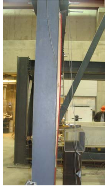
(b) Lateral deflection shape of the OSB sheet side of the wall
