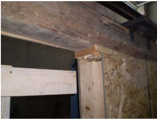
(c) Separation of the end plate and OSB
