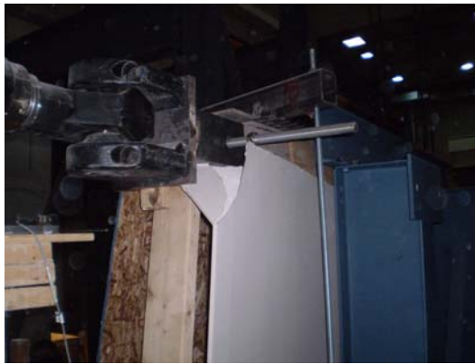
(a) Failure of gypsum board on top
