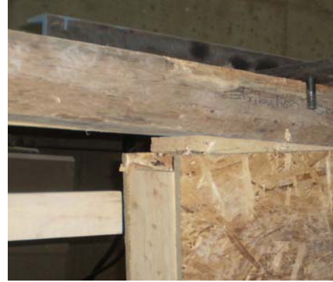
(c) Rotation of OSB sheet, nail bending and OSB crushing at nail location (d) Separation of lumbers at connection at top of the panel
