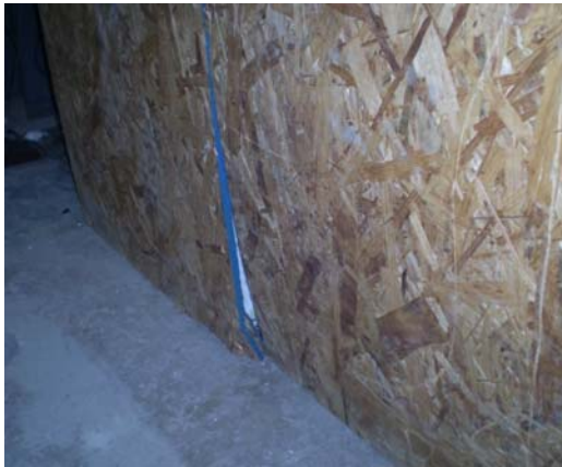
(a)Crushing of OSB at bottom of wall
