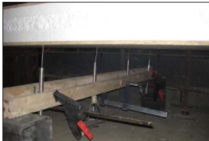
Figure 3.23 - View of LVDTs at mid-span location of SIP floor
