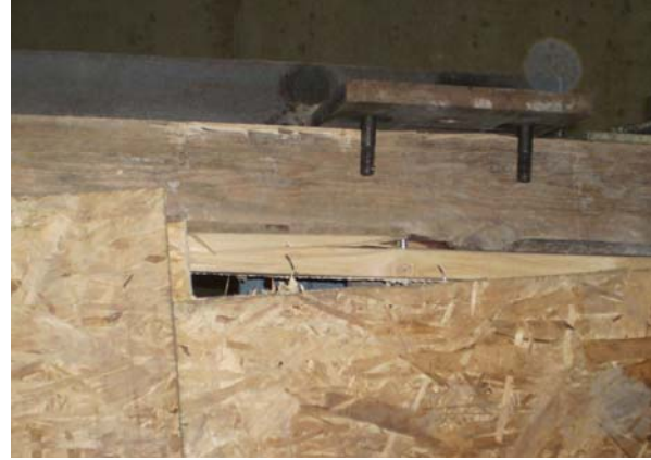
(b) Nail bending and OSB crushing
