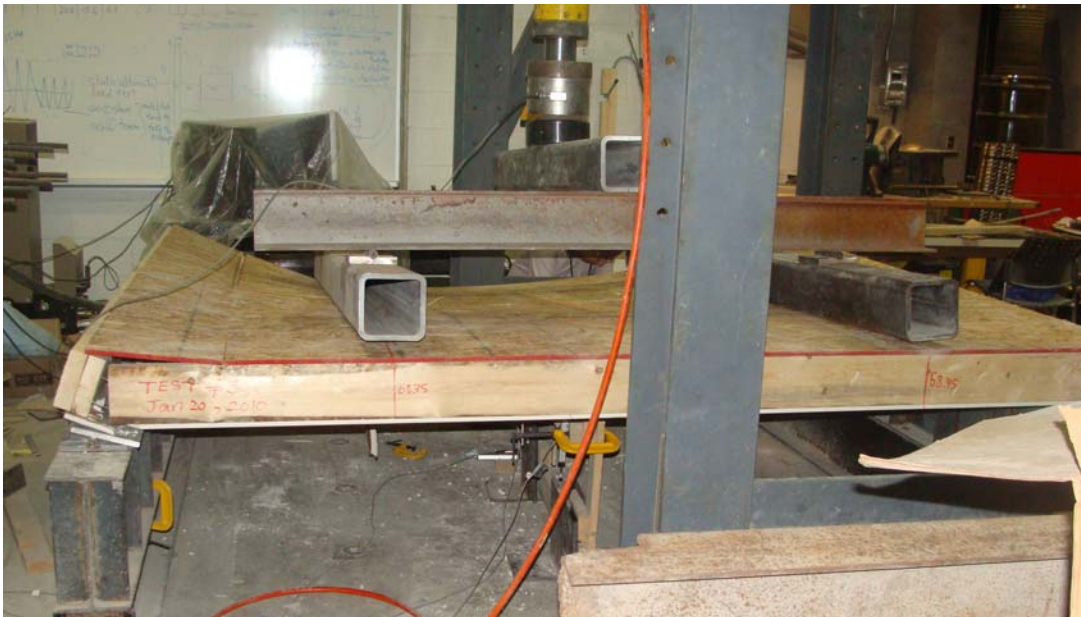
Figure 4.69 - View of the deflected shape of specimen SW-F-3 showing the bearing rotation as well as end stud and OSB sheet separation from joist No. 1
