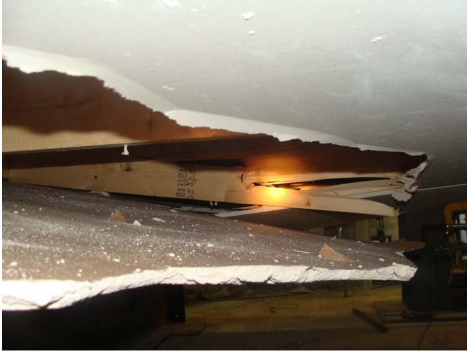
Figure 4.54 - Close-up view of the failure around the quarter point of joist No. 3 of specimen SW-F-2
