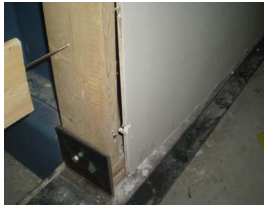
(b) Crushing of gypsum board in nail location
