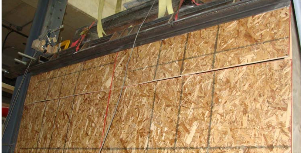
(a) View of the panel after failure showing OSB sheet joint widening near the top of wall
