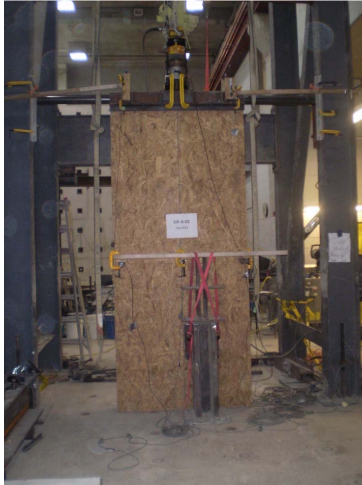
Figure 3.26 – Typical test setup for flexure eccentric compressive load of the SIP wall
