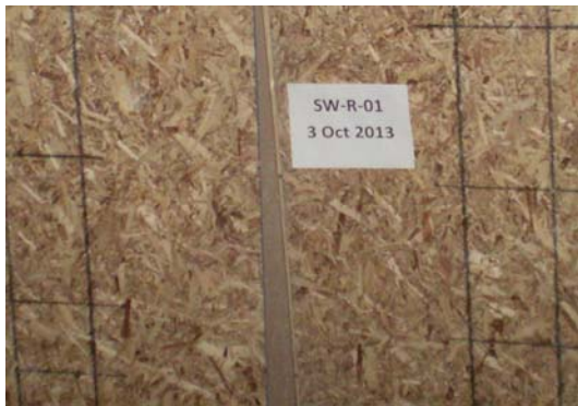
(c) Separation and crushing of OSB sheet at spline connection
