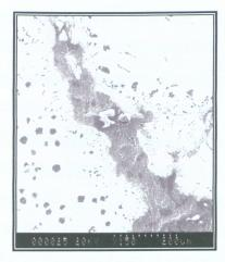
**Figure 4.17:** SEM micrograph of dross below the skin in a 14mm thick specimen cast at 1400°C. 150X.
