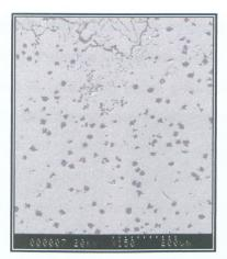
Figure 4.15: SEM micrograph of slag in a 4mm thick specimen cast at 1400°C. 100X.
