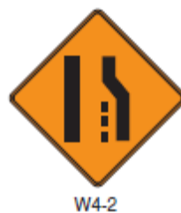
Figure 2.6: Sign for Lanes Involved in Merging Maneuvers (MUTCD, 2009)
