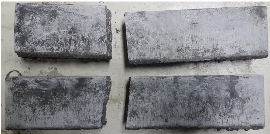
Figure 4.13: Flexural Crack due to Maximum Load for 0.5% Crumb Rubber Specimens
