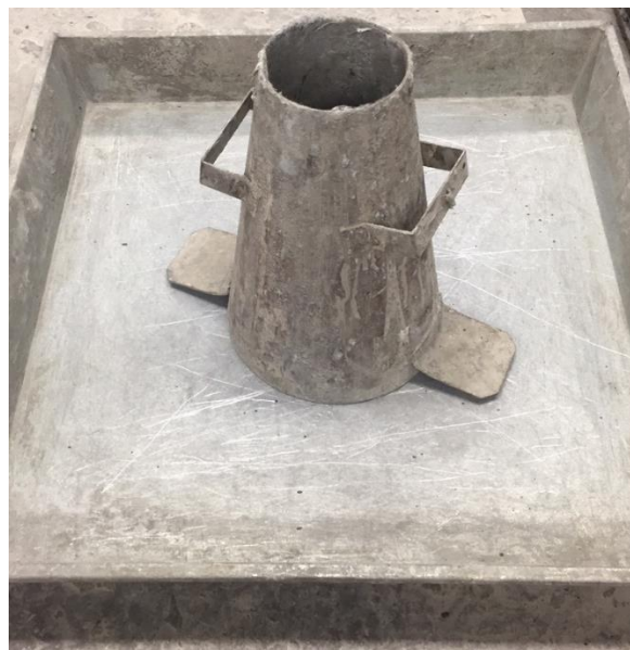
Figure 3.4: Slump Flow Test Setup
