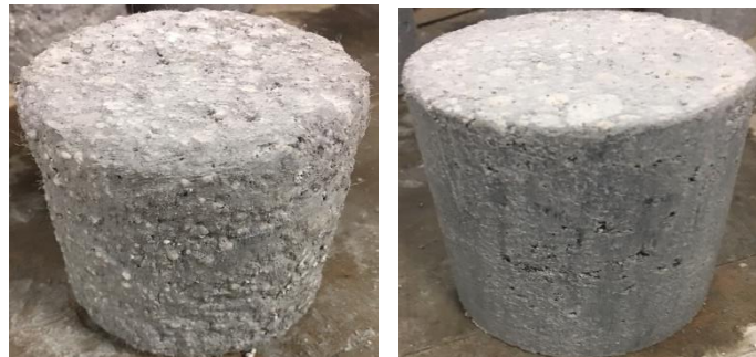
Figure 4.21: Deterioration of 0.25% PVA (Left) and 0.125% PVA (Right) after 56 Days in 5% H_2SO_4
