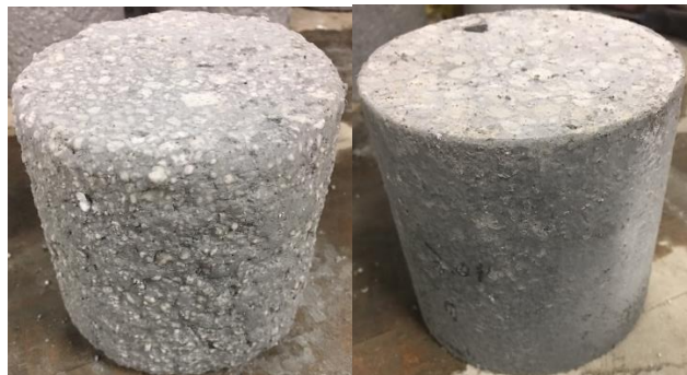
Figure 4.20: Deterioration of 1.0% Crumb Rubber (Left) and 0.5% Crumb Rubber (Right) after 56 Days in 5% H_2SO_4
