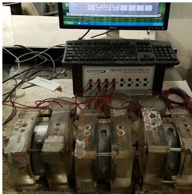
Figure 3.8: Rapid Chloride Penetration Test Setup
