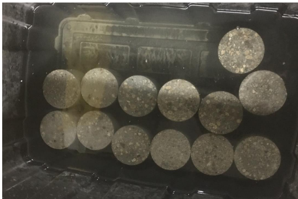
Figure 3.9: Acid Attack Test Setup
