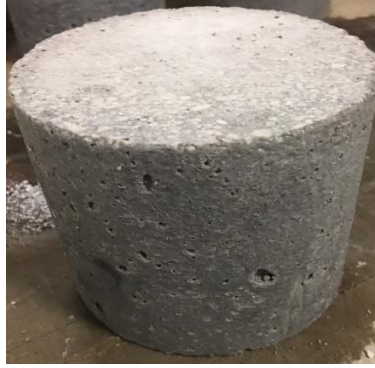
Figure 4.22: Deterioration of Control Specimen after 56 Days in H_2SO_4
