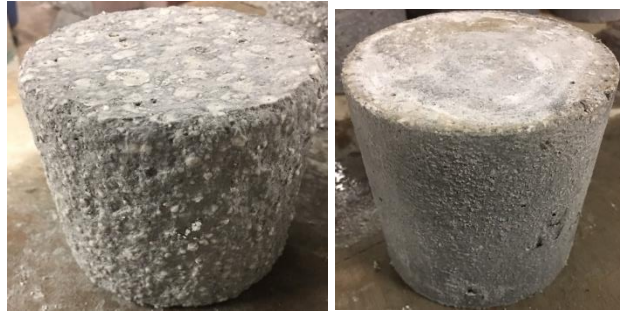
Figure 4.19: Deterioration of 1.0% HDPE (Left) and 0.5% HDPE (Right) after 56 Days in 5% H_2SO_4
