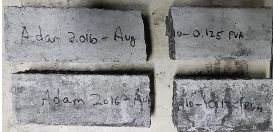
Figure 4.15: Flexural Crack due to Maximum Load for 0.125% PVA Specimens
