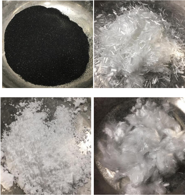
Figure 3.2: Top Left: Crumb Rubber. Top Right: PVA. Bottom Left: HDPE. Bottom Right: PE
