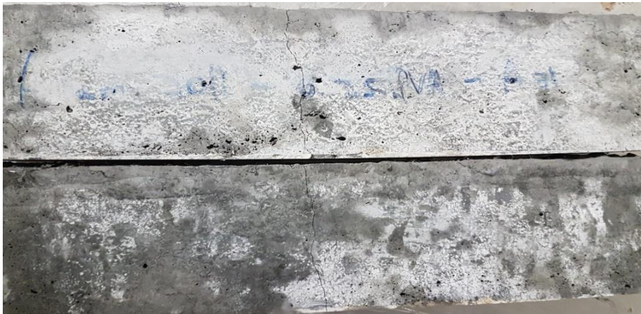
Figure 4.16: Flexural Crack due to Maximum Load for 0.25% PVA Specimens
