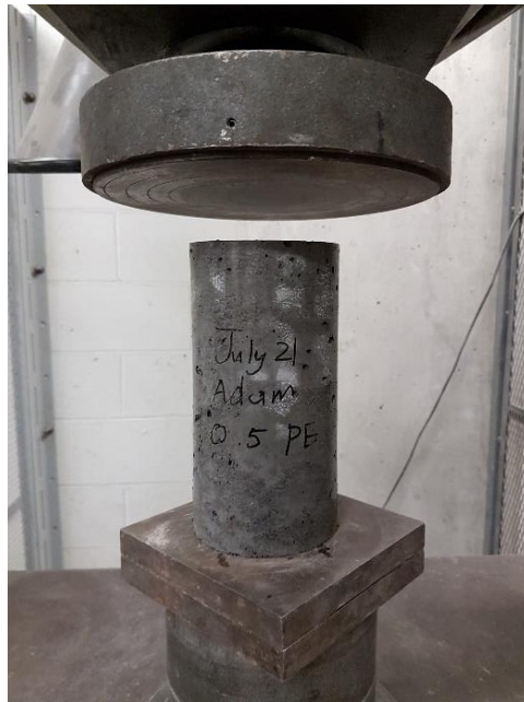
Figure 3.5: Compressive Strength Test Setup
