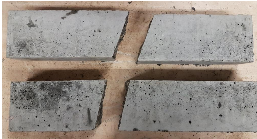
Figure 4.10: Flexural Crack Due to Maximum Load for Control Specimens
