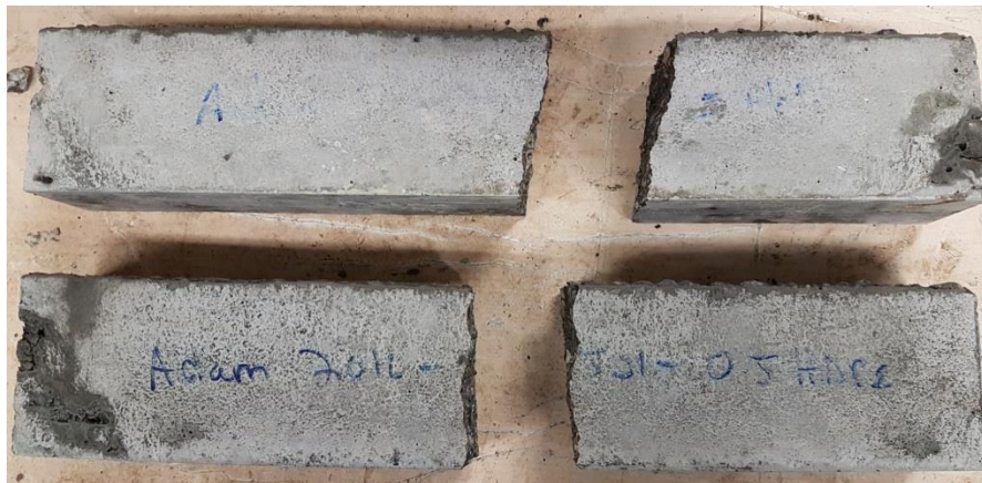
Figure 4.11: Flexural Crack Due to Maximum Load for 0.5% HDPE Specimens
