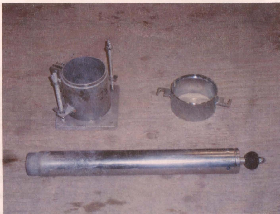
Figure 3.6. Proctor Mould, Filling Collar and Compaction Hammer.
