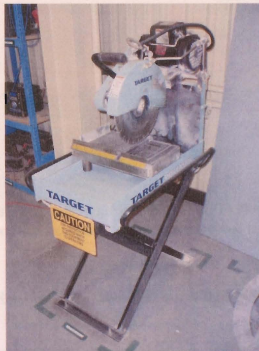
Figure 3.5. Target concrete saw used for preparing cylinders for RCPT.
