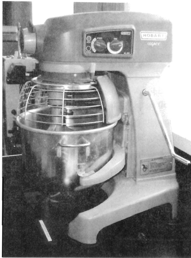
Figure 3.1. The Hobart HL200 Paddle Mixer used for all ready mix preliminary batching.
