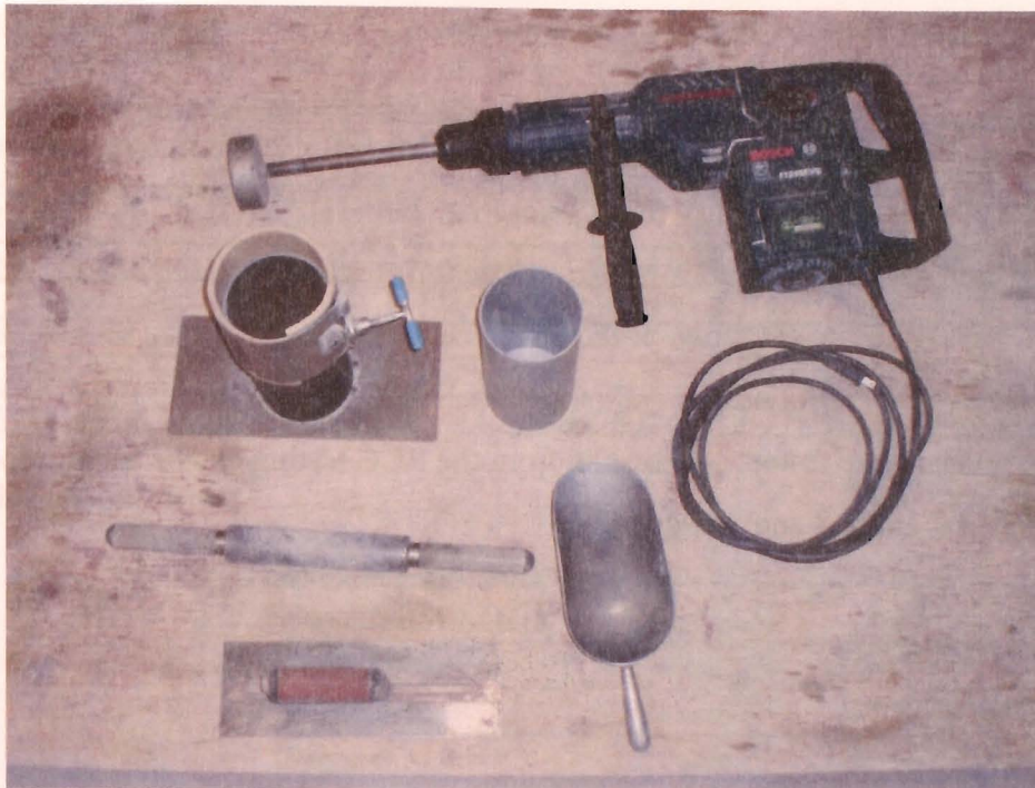
Figure 3.11. Impact hammer, tamping plate, mould sleeve with filling collar and finishing tools.
