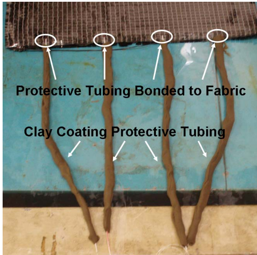
Figure 22 - Bottom Fabric Layer with Fiber Optics in Place
