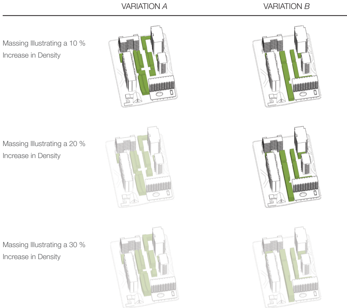
Figure 30 Massing Variations Exploring the Effect of an Increased Physical Density on the Mid-block Experience (Sauder, 2015).
