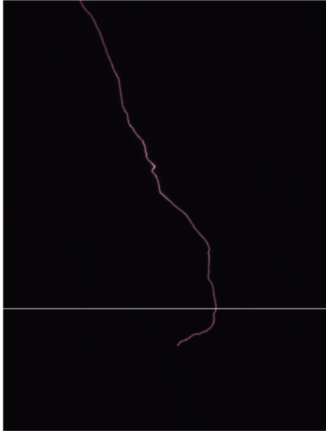
Figure 4.16 – Channel trajectory image of the third flash recorded on July 8, 2013.
