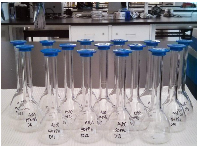
Figure 13: Production of standard solutions for each of the chosen arsenic concentrations.
