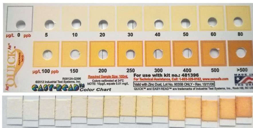
Figure 36: Aged samples, faded but still may be quantified six months after production.
