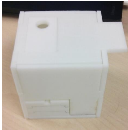
Figure 24: The first attempt at a 3D-printed imaging apparatus for in field use.
