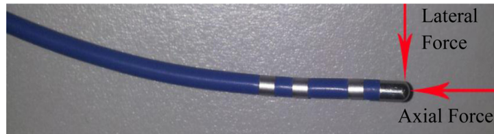
Figure 1.10: Axial and lateral forces applied to the tip of an ablation catheter
