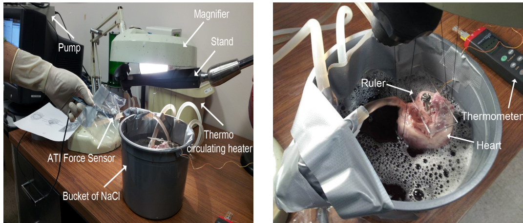
Figure 2.10: Experimental setup for measurement of applied force to MA from CS
