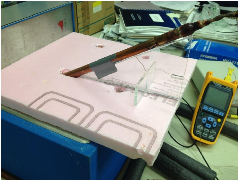
Figure 5-12: The setup of thermosyphon at 30 degrees
