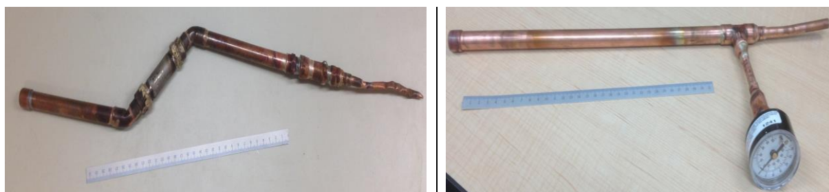
Figure 5-3: The manufactured thermosyphon, S (left) and I (right) shape
