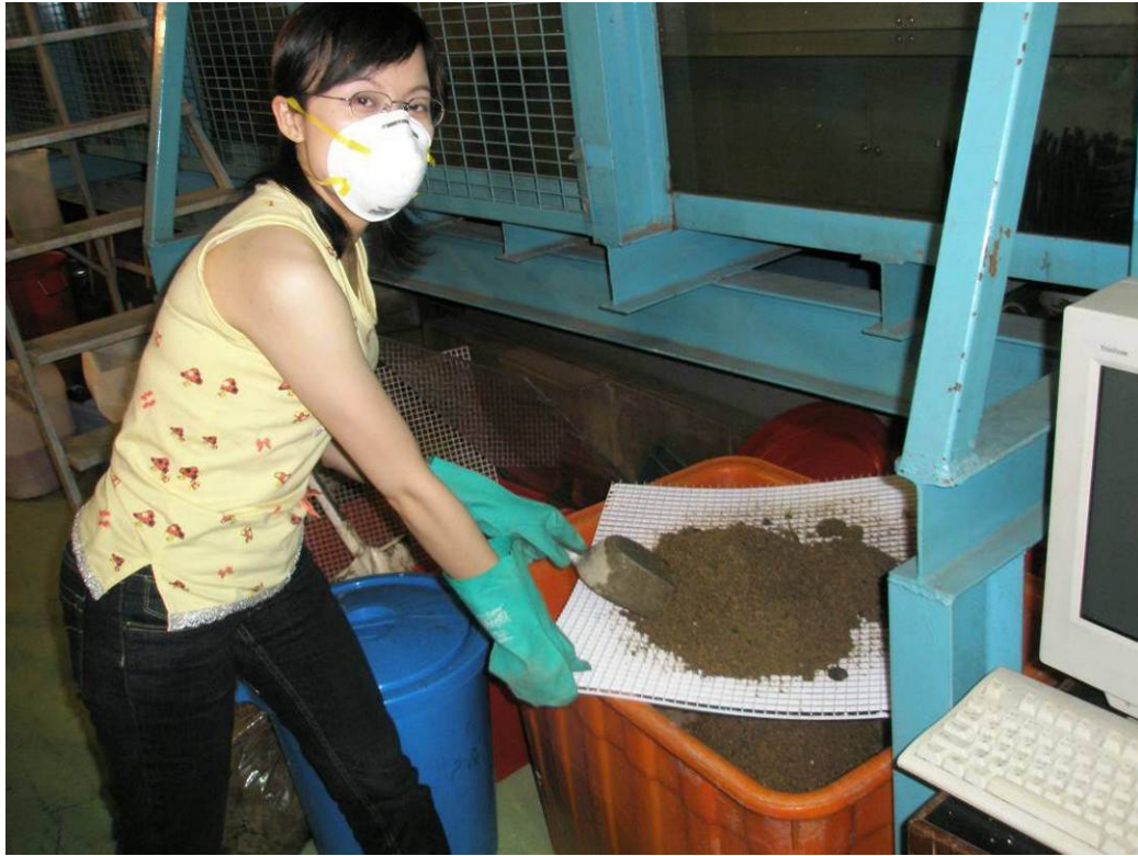
Figure 64: Preliminary screening of the sediment.
