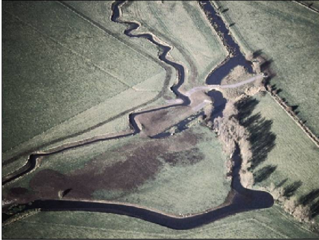
Figure 6: The new meandering river course and the restored meander in the mill leat (Burns, 2002).
