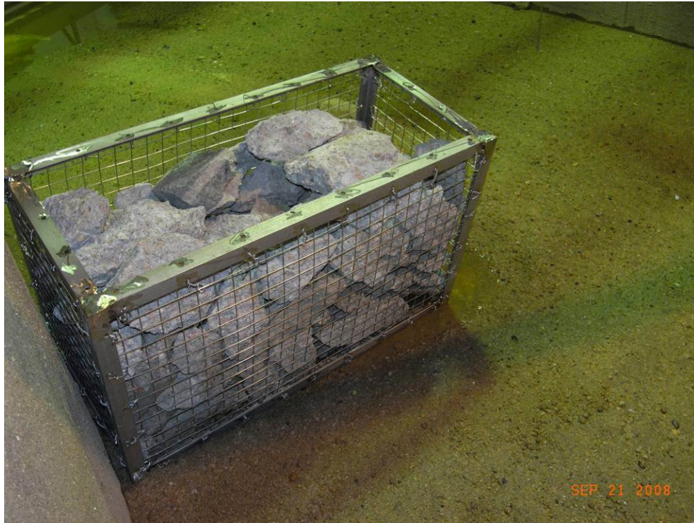
Figure 50: Deflector of the physical experiments.
