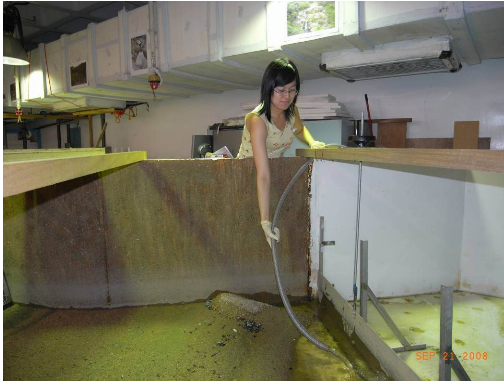
Figure 71: Filling water to the physical model from the outlet drop.
