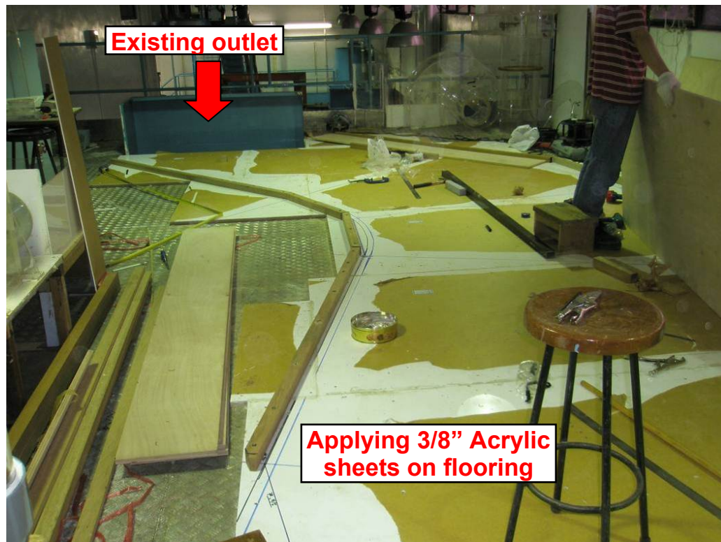
Figure 43: Flooring of the physical model.
