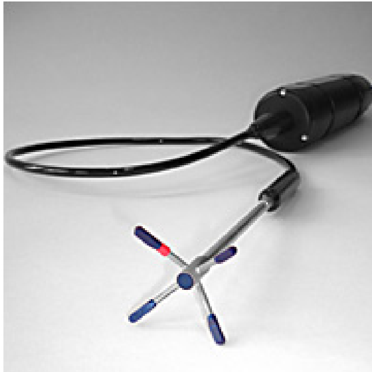
Figure 69: Four-port ADV used for the velocity profile measurement.
