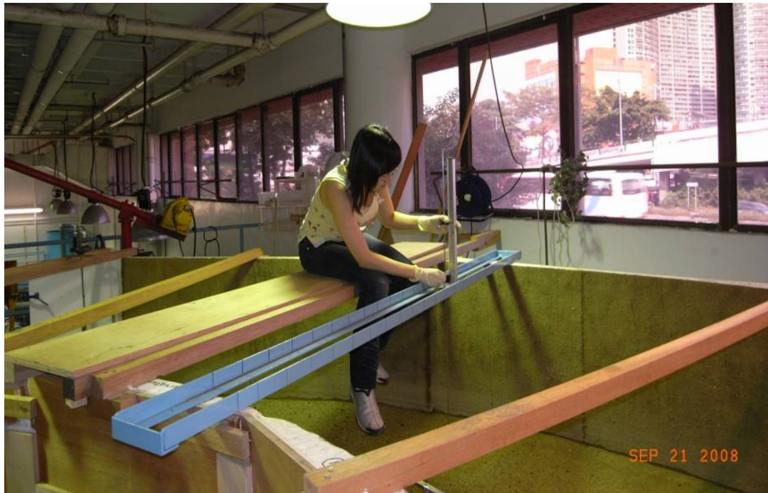
Figure 70: Sediment profile measurement using a height gauge.
