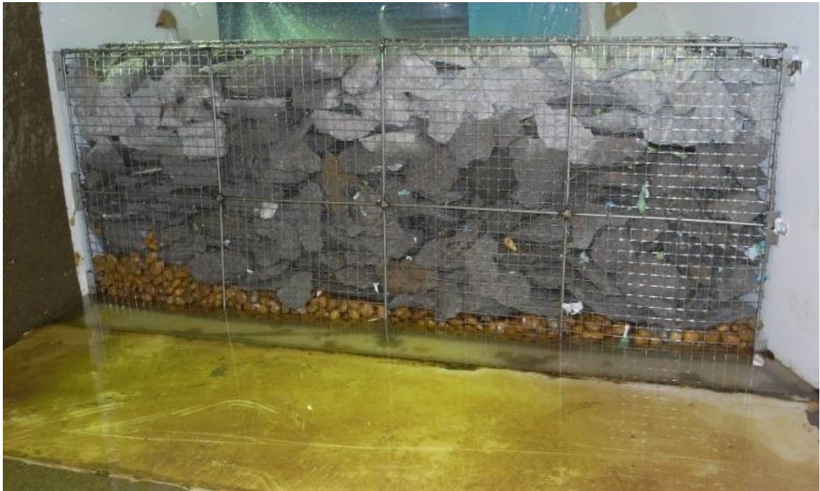
Figure 56: Baffle wall with crushed concrete.
