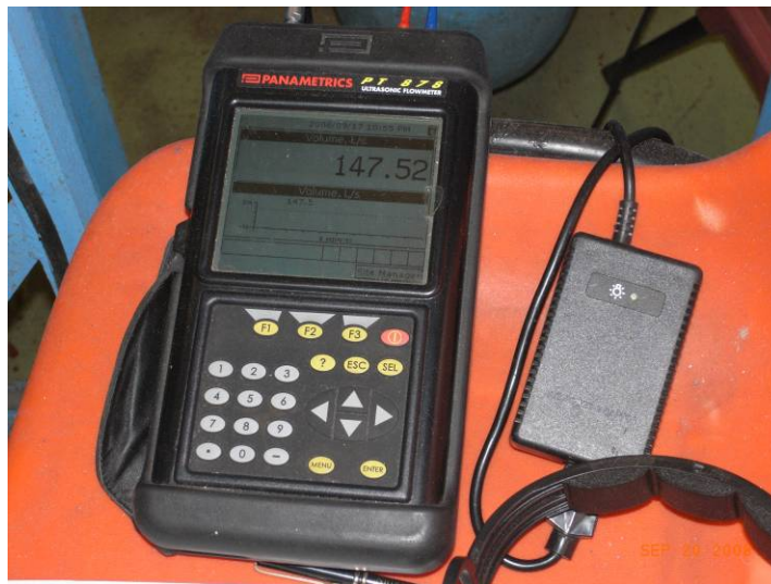
Figure 67: Flow meter with sensor connected to the inlet pipe of the holding tank.
