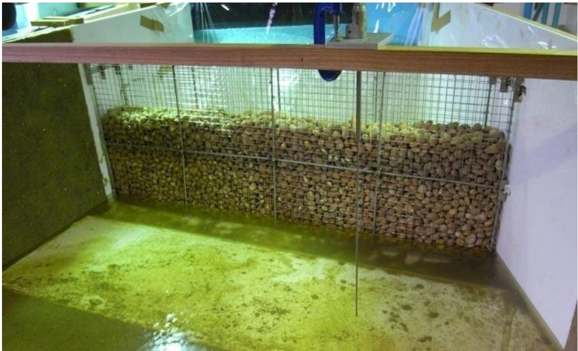
Figure 57: Baffle wall with rounded pebble stones.
