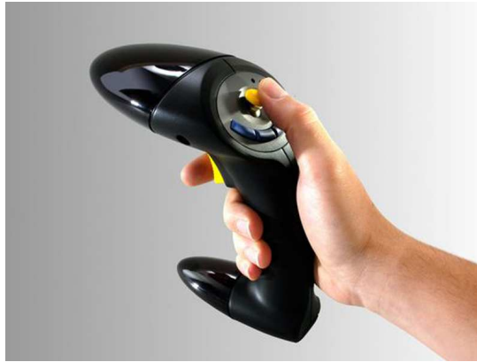
Figure 3.2: A wand input device (Flystick).
