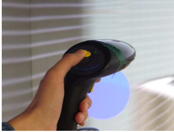
Figure 3.10: Demonstration of joystick navigation: the right hand is used to point out a direction and pushing on the joystick activates flying.
