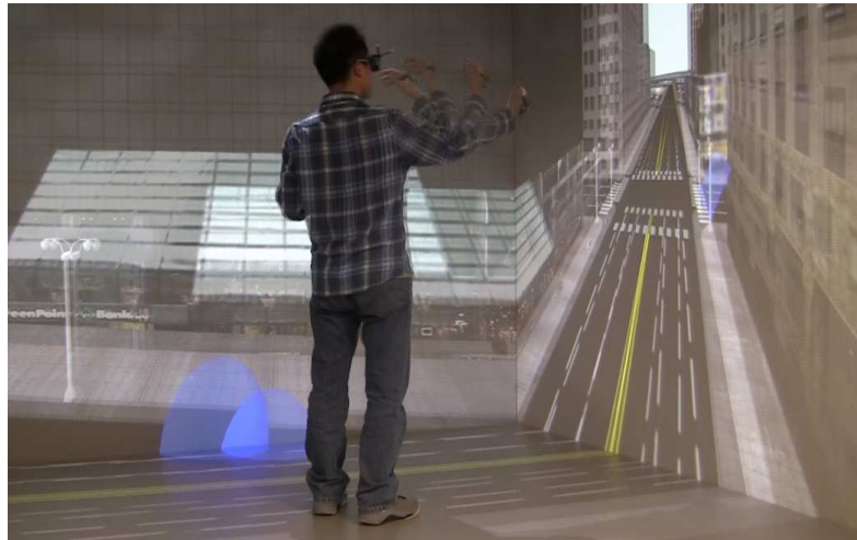
Figure 3.12: Demonstration of waving hand navigation: fly to the direction of hand waving.
