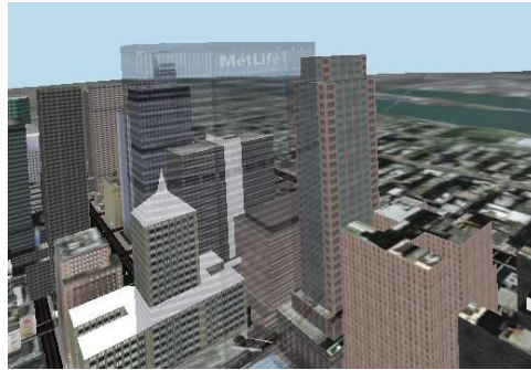
Figure 3.20: View from the same point when occluding building is semi-transparent, with a transparency of 20%.
