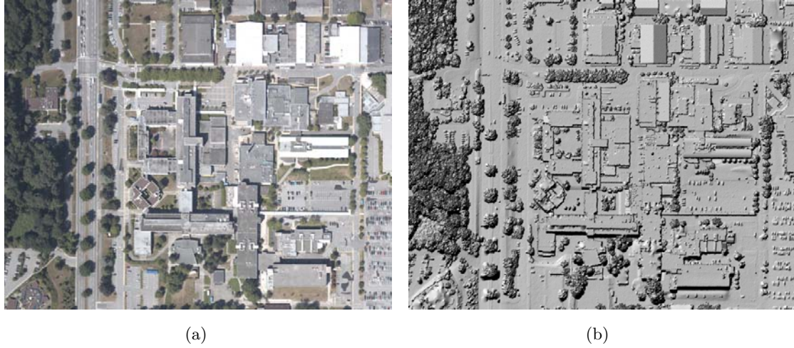
Figure 5.2: (a) Aerial photo and (b) shaded DEM generated from the LiDAR data in the 1 st case
