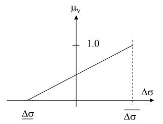
Figure 8 Satisfaction function  $\mu_V$  for the second objective of Voltage Stability Margin Maximization
