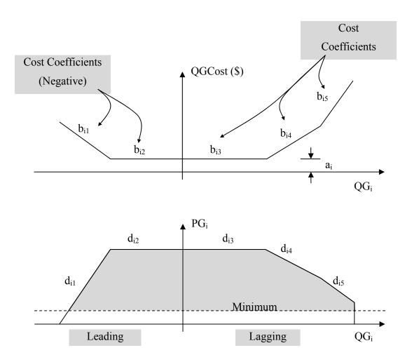
Figure 6 Combined reactive power pricing and capability charts Note: The coefficients d<sub>12</sub> and d<sub>13</sub> are zero. As a convention, QG<sub>i</sub> is taken positive when lagging and negative when leading.
