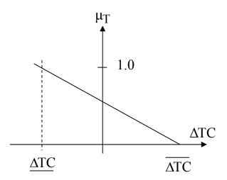
Figure 7 Satisfaction function  $\mu_T$  for the first objective of Total Cost Minimization
