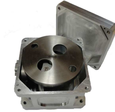
Figure 2.6 Reaction wheel unit developed in the SSDC lab at Ryerson University
