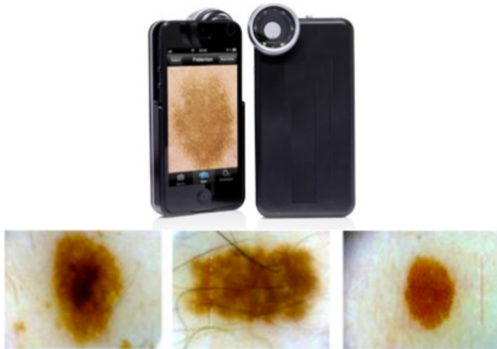
Figure 2.7: The dermatoscope device attached to the iPhone and sample of images captured using the device [22]
