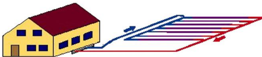
Figure 2.3: Horizontal ground loop configuration (reproduced from [5])
