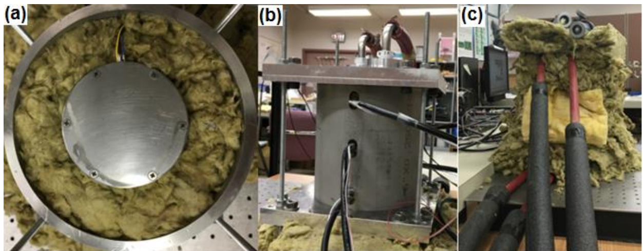
Fig. C.4 From left to right: (a) Top view of modified model #3 soil cell which is surrounded by fiber glass insulation and outer stainless steel tube, (b) Side view of the apparatus without outer insulation layer and (c) Side view of the apparatus with outer insulation layer
