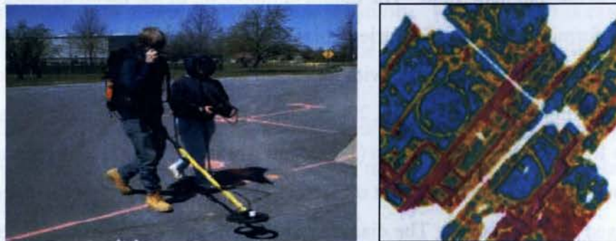
Figure 3.6 Field survey and imagery using a metal detector (www.geomodel.com).
