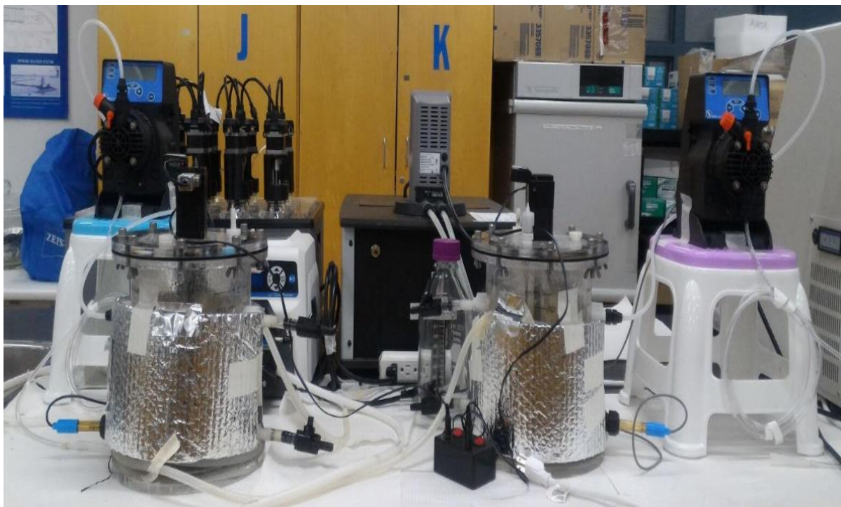
Figure 3 Photograph for bench scale PS anaerobic acid fermentation experimental set up
