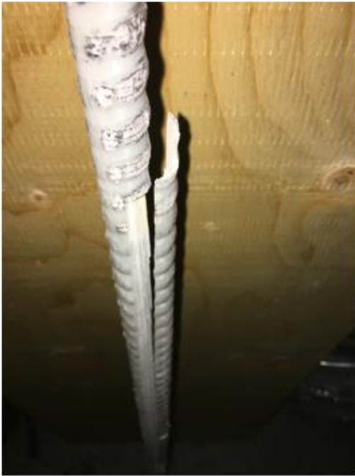
a) Bar A rupture at the anchorage
