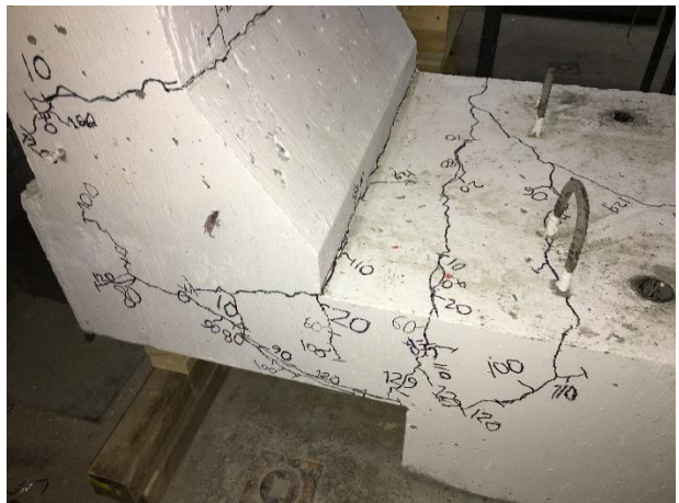
Figure 4.32: Close up view of crack pattern after failure of specimen B-2
