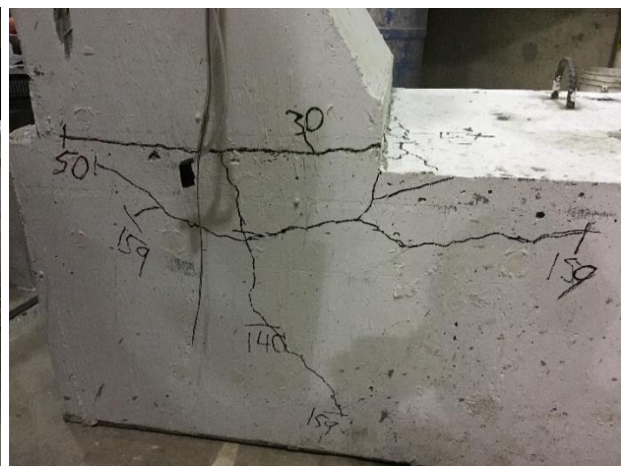
Figure 4.40: Close up view of crack pattern after failure of specimen B-5
