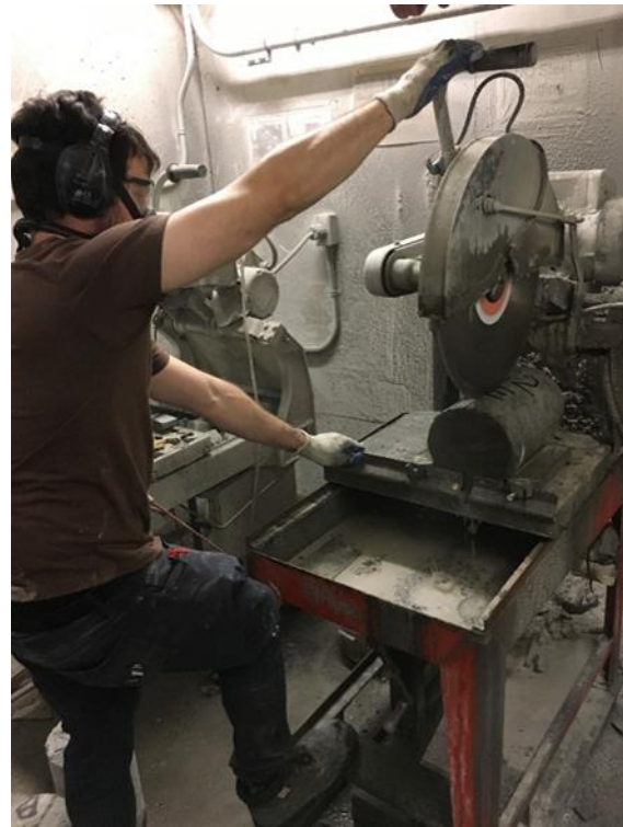
Figure 3.19: Slicing the cored samples in half
