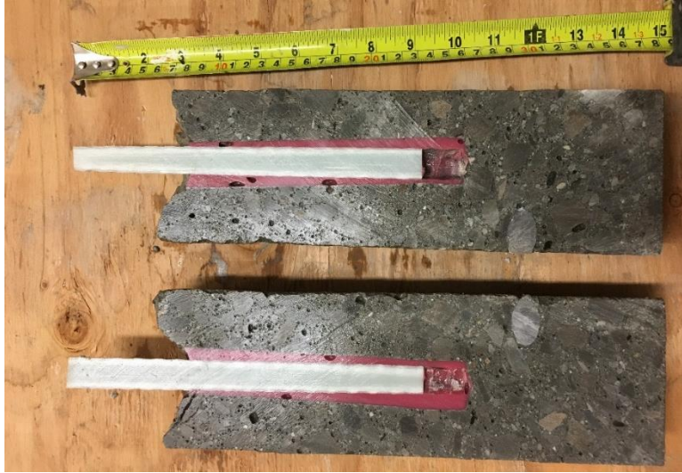
Figure 3.31: Sliced core sample for post-installed bars in group 3 showing bar slip
