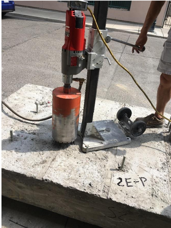
Figure 3.18: Coring of the slab for analysis
