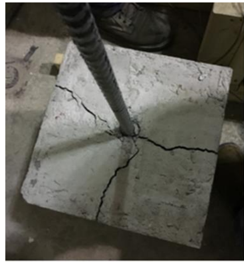
b) View of concrete splitting failure
