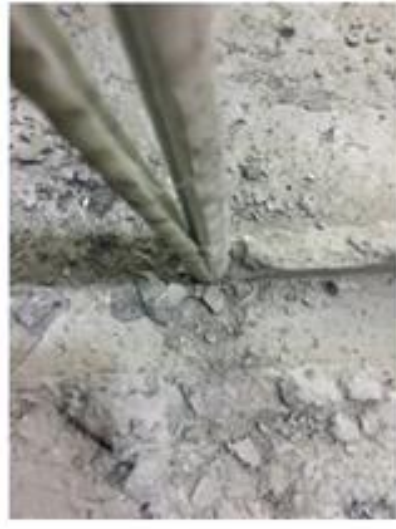
c) Light concrete crushing around the bar
