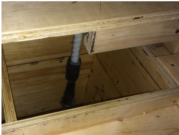
a) View of the timber form and unbonded headed bar
