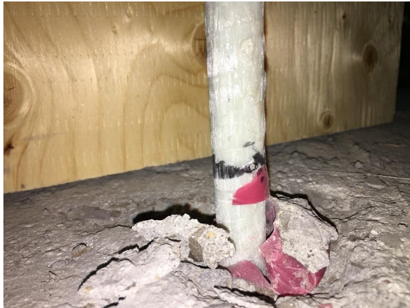
Figure 3.28: Slippage failure mode of post-installed bars in group 2
