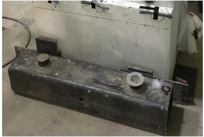
b) Steel HSS attached to barrier front side and tied-down to lab floor to prevent barrier sliding
