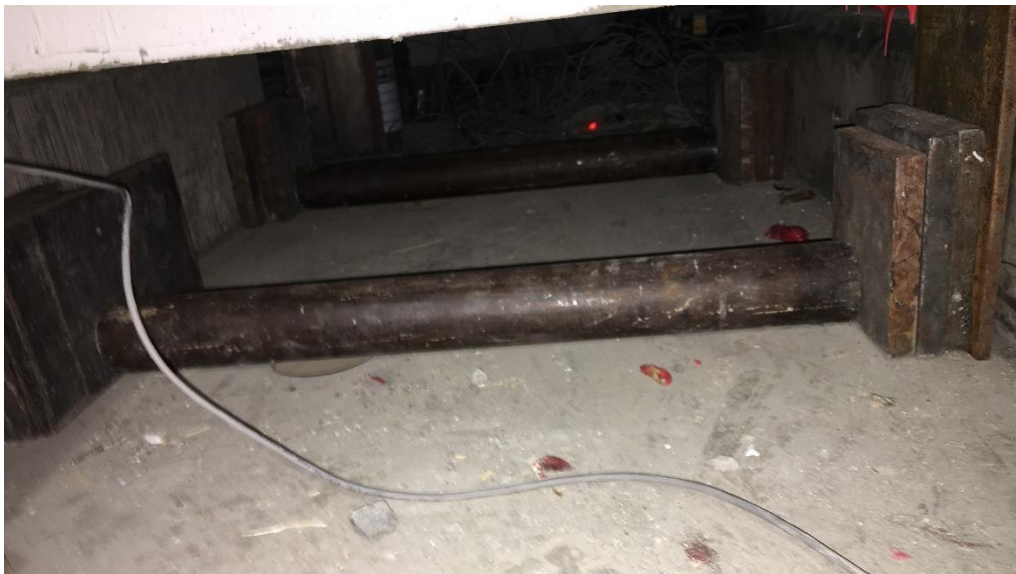
c) Setup underneath deck cantilever to prevent barrier sliding over floor under transverse loading
