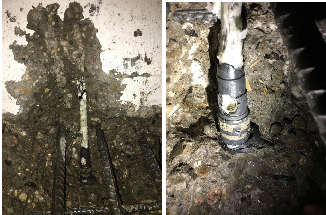
Figure 4.25: Close up of failed headed GFRP bar in specimen B-1 after jack hammering concrete at barrier-deck junction
