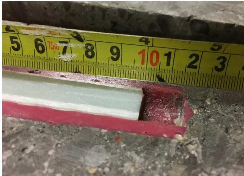
Figure 3.27: Close up view of slip of post-installed bar specimen D in group 1
