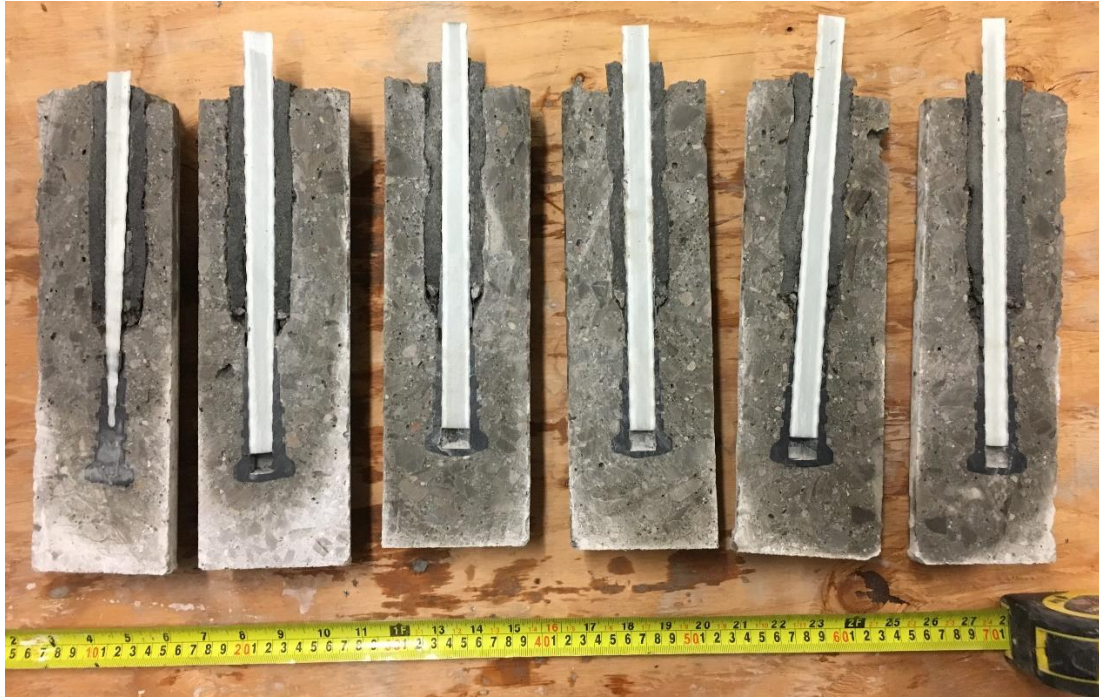
Figure 3.24: View of the sliced core samples for group 3 showing bar slip from head
