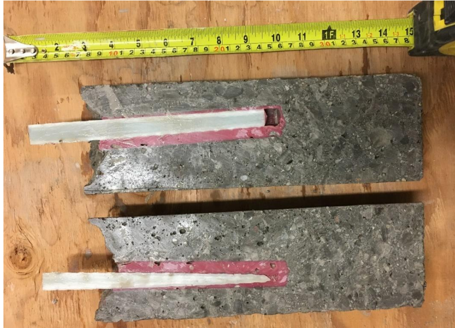
Figure 3.29: Sliced core sample for post-installed bars in group 2 showing bar slip
