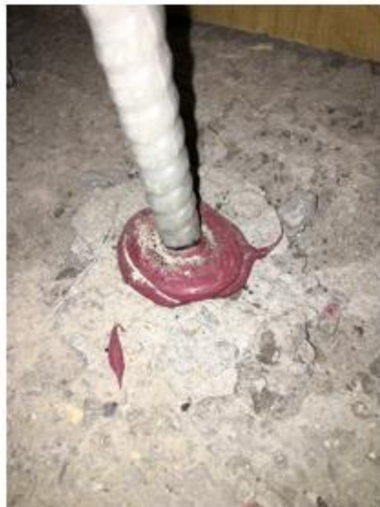
b) Conical concrete failure in 3-A
