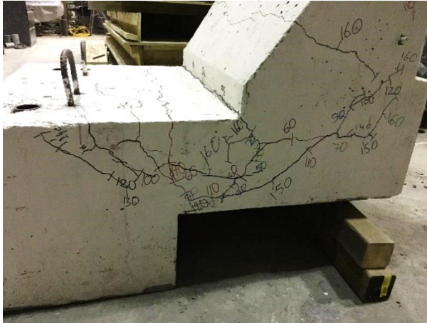
Figure 4.36: Close up view of crack pattern after failure of specimen B-4
