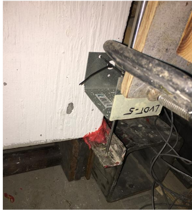
b) Location of Pot on the right side of the slab to measure barrier wall vertical deflection
