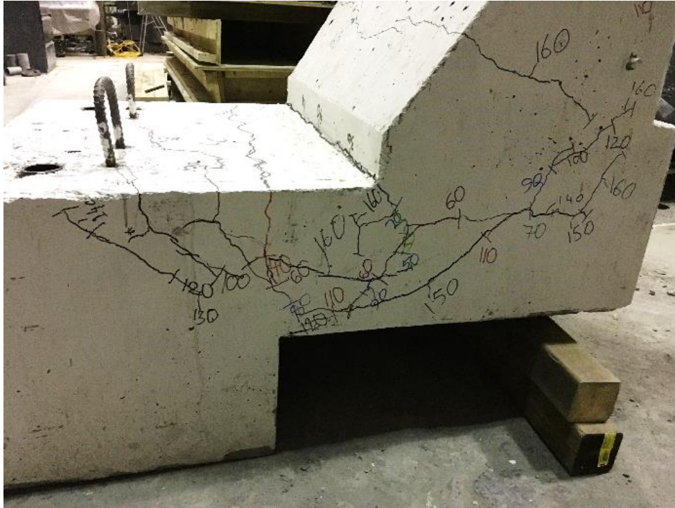
Figure 4.66: Barrier B-4 exterior location; similar diagonal cracking is visible
