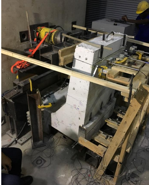
Figure 4.17: Typical test setup for a barrier resting over deck cantilever (test in progress in the photograph)
