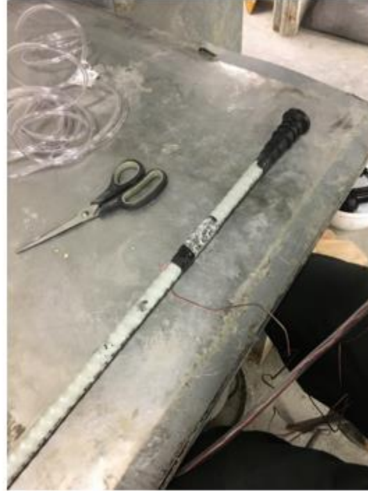
b) strain gauge covered with tape for protection
