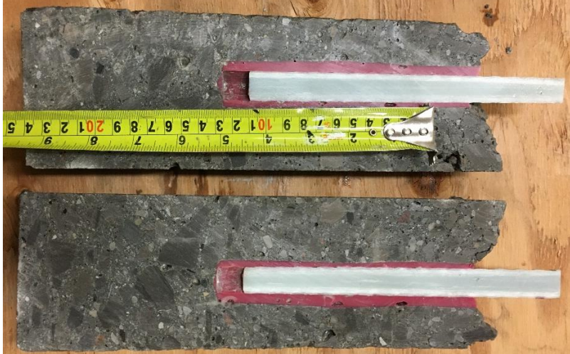
Figure 3.26: Sliced core sample for post-installed bars in group 1 showing bar slip
