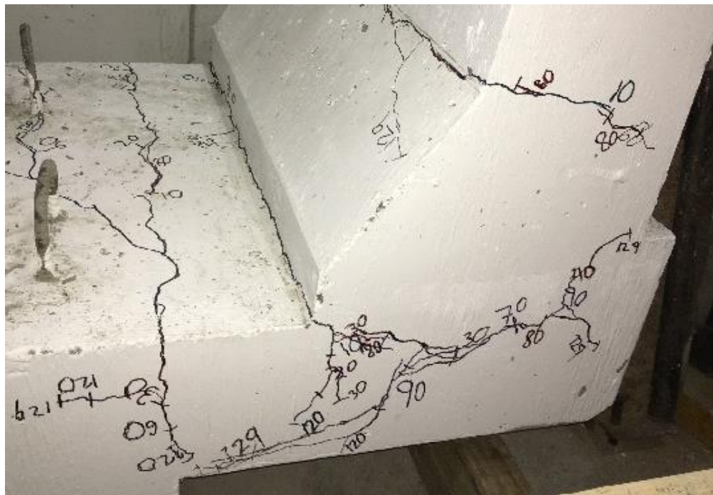
Figure 4.65: Barrier B-3- Interior location cantilever; diagonal cracking is evident in areas and lengths mentioned above
