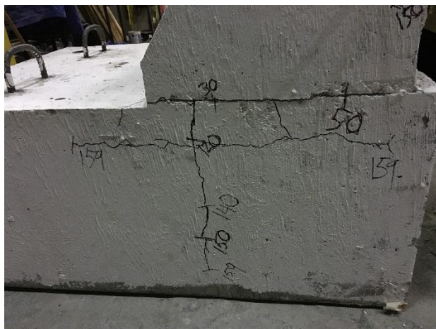
Figure 4.40: Close up view of crack pattern after failure of specimen B-5
