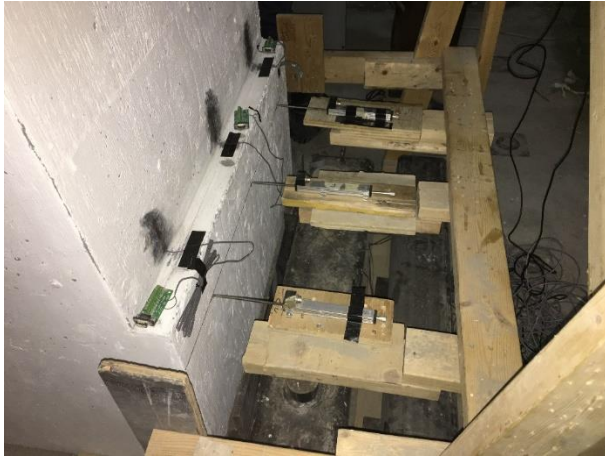
a) Locations of Pots at the level of the deck slab and concrete strain gauges to the side of the wall
