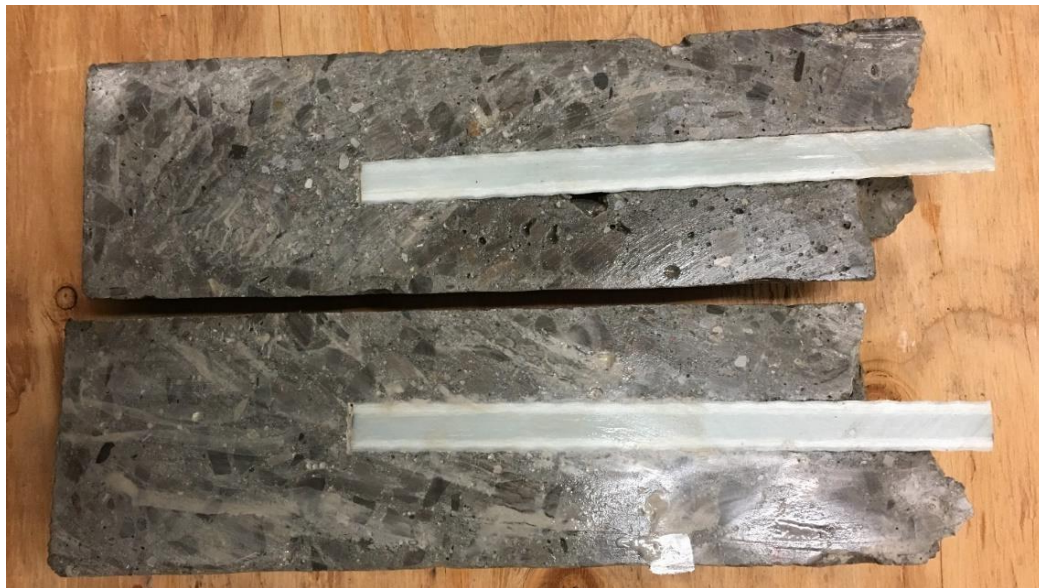
Figure 3.20: Sliced core sample for group 1 showing no bar slip
