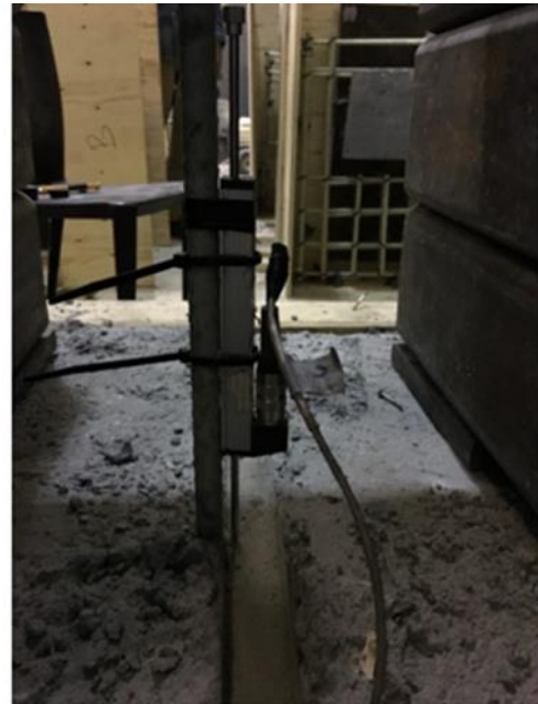
c) Close-up view of the POT to measure bar slip
