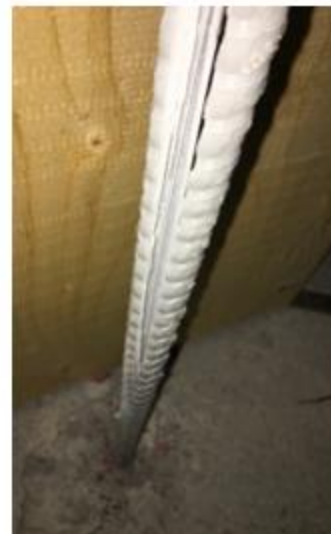
c) Bar rupture in 3-C
