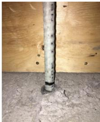
Figure 3.23: View of straight-end GFRP bar slippage from concrete
