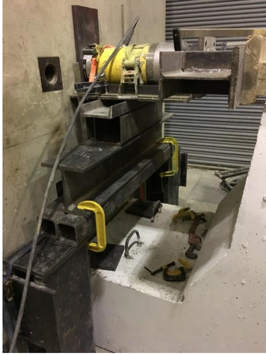
a) Setup for load application and tie-down anchors at back of deck slab
