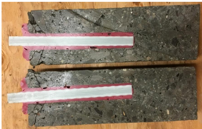
Figure 3.32: Sliced core sample for post-installed bars in group 3 showing conical failure
