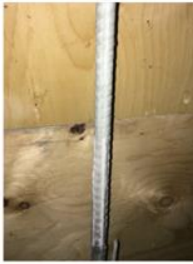
b) bar rupture at grip area
