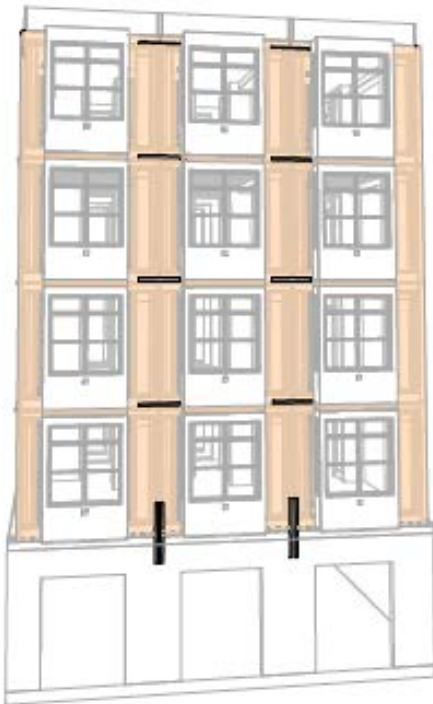
3. Install straps between modules and to the podium
