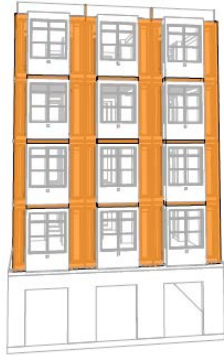
2. Shear plywood installed across horizontal and vertical mate lines
