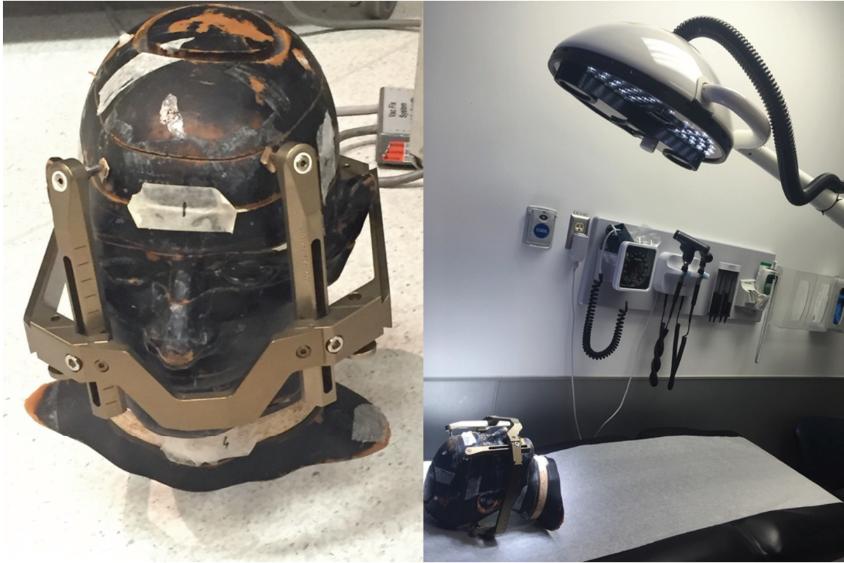
Figure 6.1: Left Panel: “Rando” anthropomorphic head phantom with Leksell stereotactic frame attached. Right Panel: Experimental set-up for acquisition of optical topographical image.
