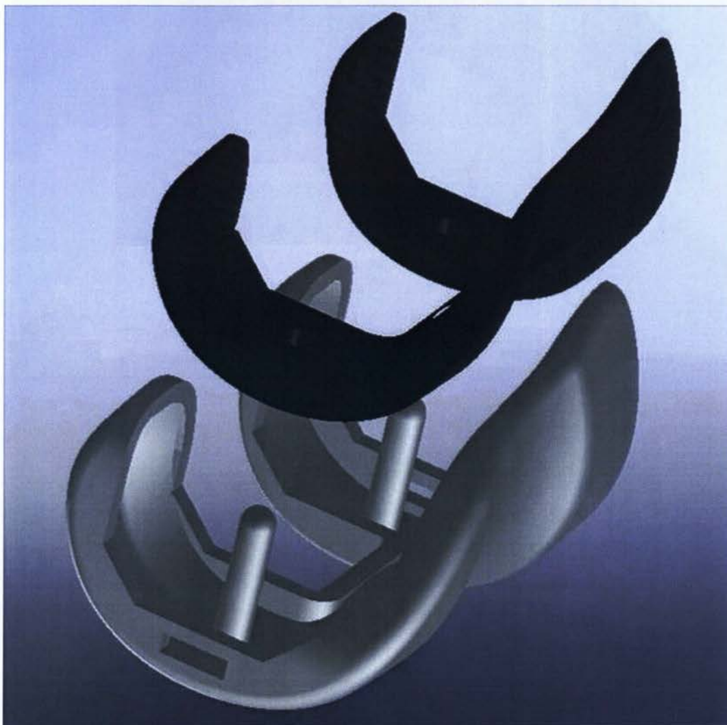
Figure 7.7 Exploded view of the hybrid femoral component, showing the CF/PA12 layer
