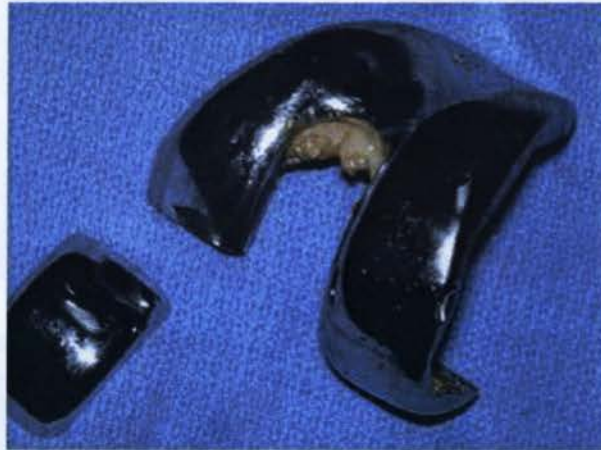
Figure 6.12 Fracture of a PFC femoral component from Duffy et al. [204]
