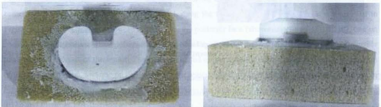
Figure 6.13 Superior (left) and anterior (right) view of the tibial components implanted in a brick of synthetic cancellous bone tissue
