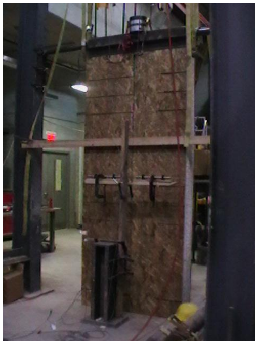
Figure 4.15. View of specimen BW3 after failure due to crushing of OSB face at the top of the wall
