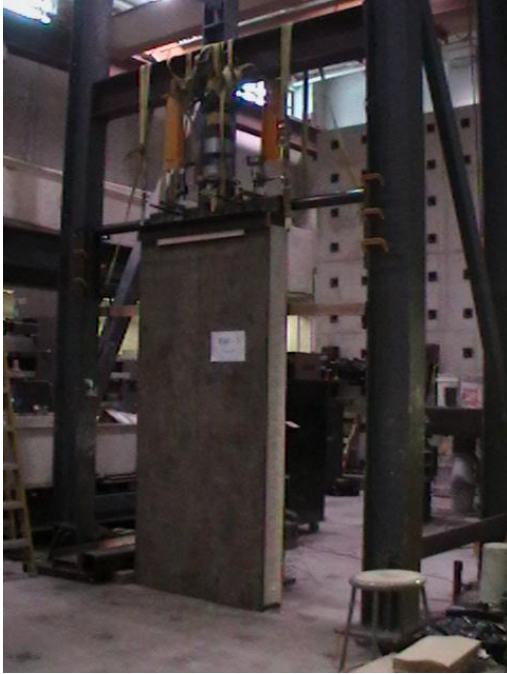
Figure 4.20. Views of the front and back faces of specimen BW5 before axial load testing
