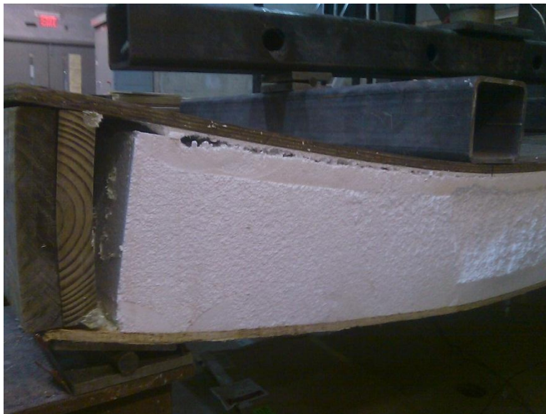
Figure 4.35. View of the east edge of the end of specimen BW3 showing shear failure at the interface between the top plywood face and foam core
