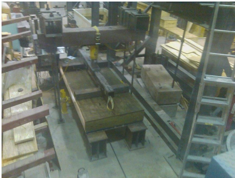
Figure 4.25. View of specimen BW1 before flexural load testing
