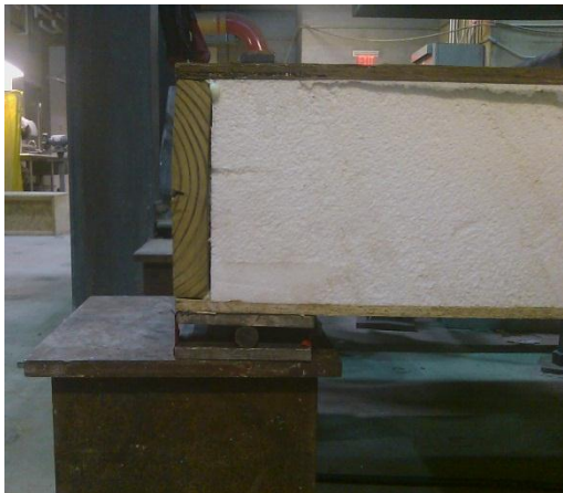
Figure 3.23. Views of the bearing plate assembly used to transfer applied loading to the supports
