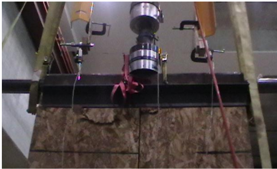
Figure 4.16. Close-up views of specimen BW3 after failure showing crushing of OSB face near the top of the wall
