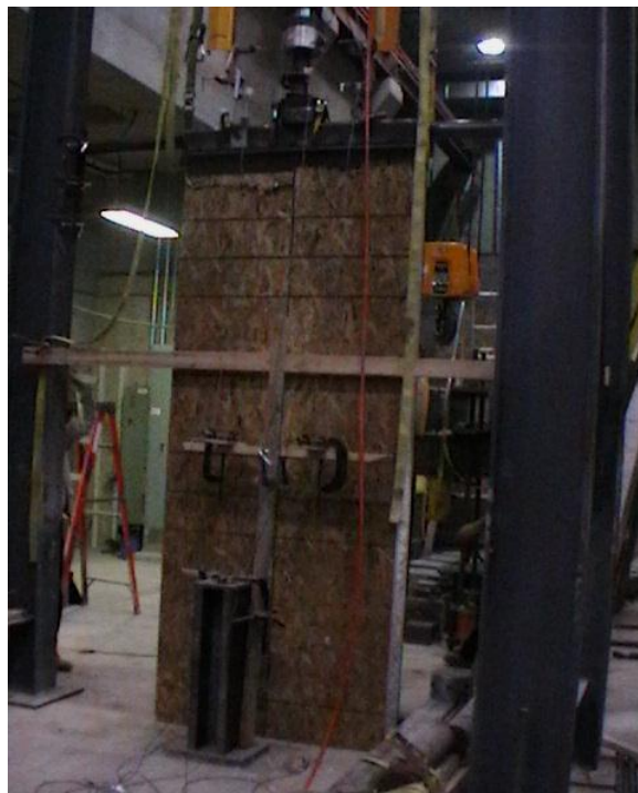
Figure 4.6. View of specimen BW1 after failure showing crushing of OSB face near the top of the wall
