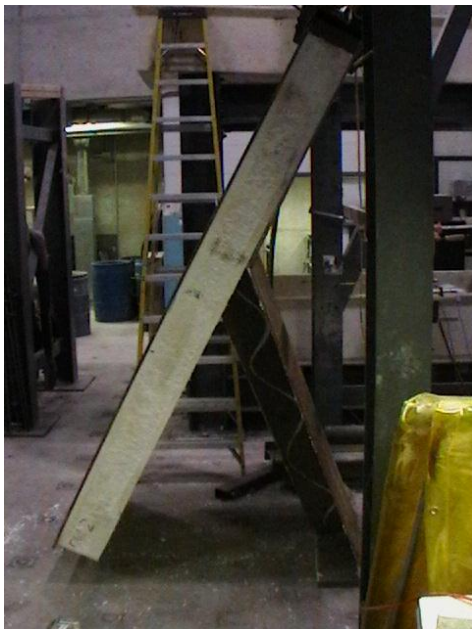
Figure 4.13. Views of fracture of the lumber stud at the connection and diagonal crack of the foam after splitting from the OSB face of specimen BW2
