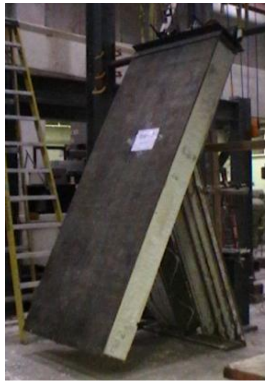
Figure 4.12. Views of back face of of specimen BW2 at the end of axial load testing
