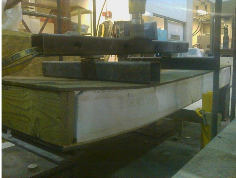
Figure 4.26. View of deformed shape of specimen BW1 after flexural load testing
