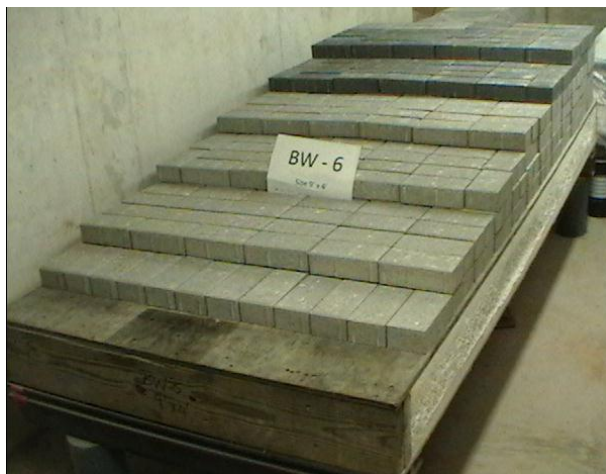
Figure 3.12. View of specimen BW6 during creep testing
