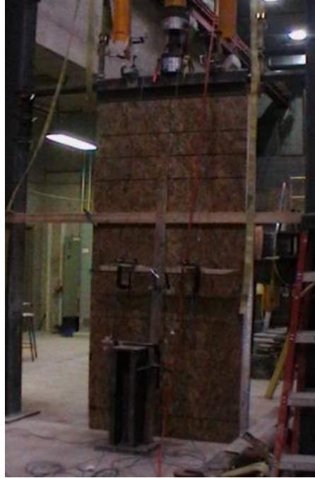
Figure 4.9. Views of front and back faces of specimen BW2 before axial load testing
