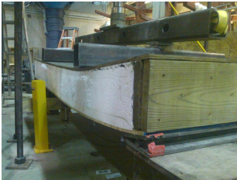
Figure 4.29. View of deformed shape of specimen BW2 after flexural load testing
