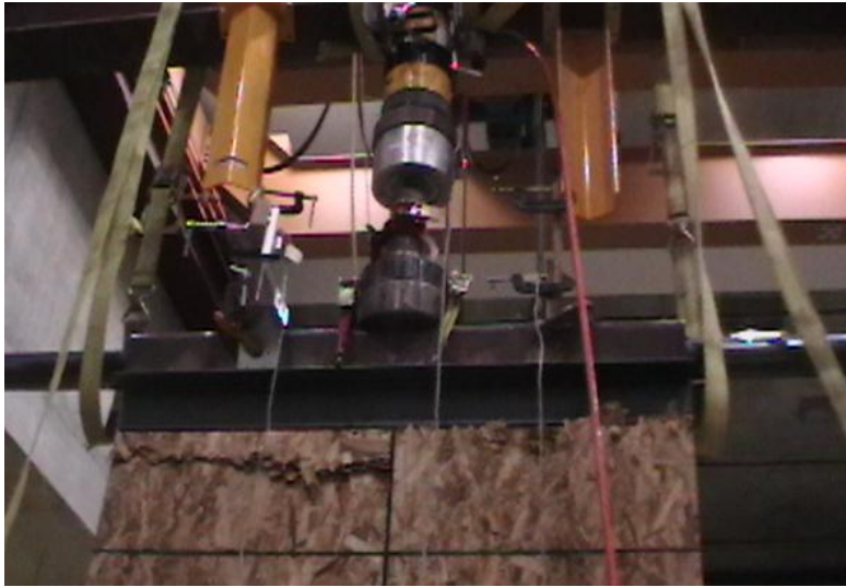
Figure 4.7. Close-up view of specimen BW1 after failure showing crushing of OSB face near the top of the wall
