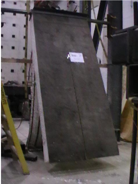
Figure 4.12. Views of back face of of specimen BW2 at the end of axial load testing
