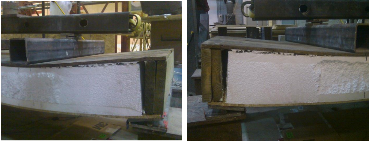
Figure 4.30. Views of shear failure at the interface between the top plywood face and foam core of specimen BW2 after flexural load testing
