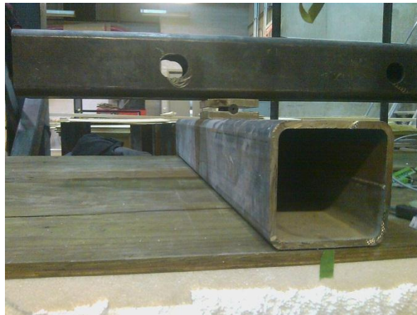
Figure 3.23. Views of the bearing plate assembly used to transfer applied loading to the supports
