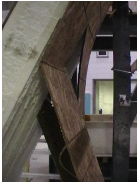
Figure 4.10. Views of crushing failure mode of the OSB face, delamination at OSB-foam interface and fracture of the lumber stud at the connection of specimen BW2 at the end of axial load testing
