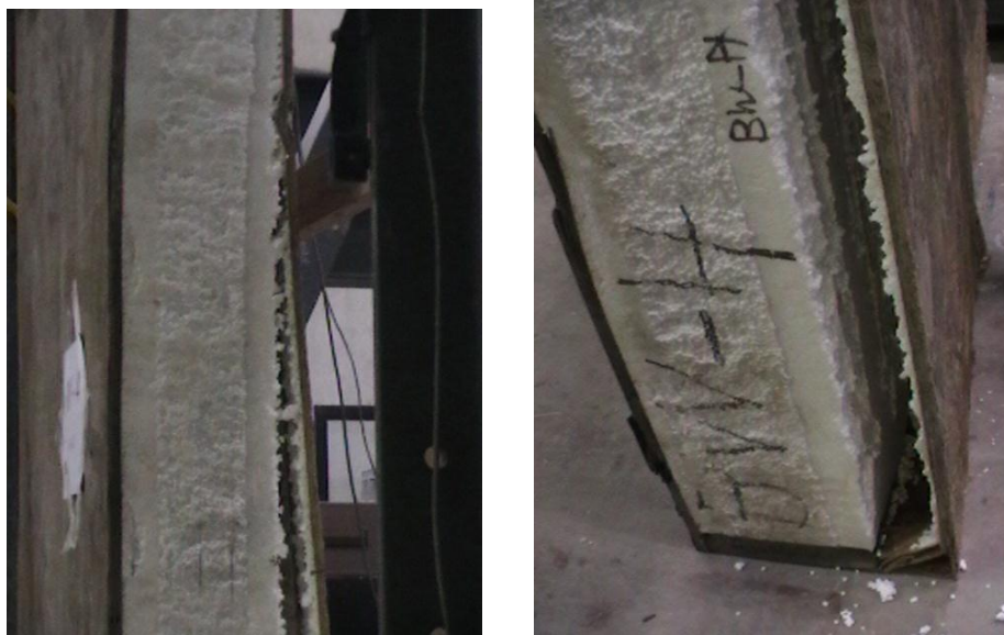
Figure 4.19. a) Close-up view of OSB-foam delamination near the top of the wall, b) Close-up view of the OSB-foam delamination and OSB crushing at the bottom of specimen BW4
