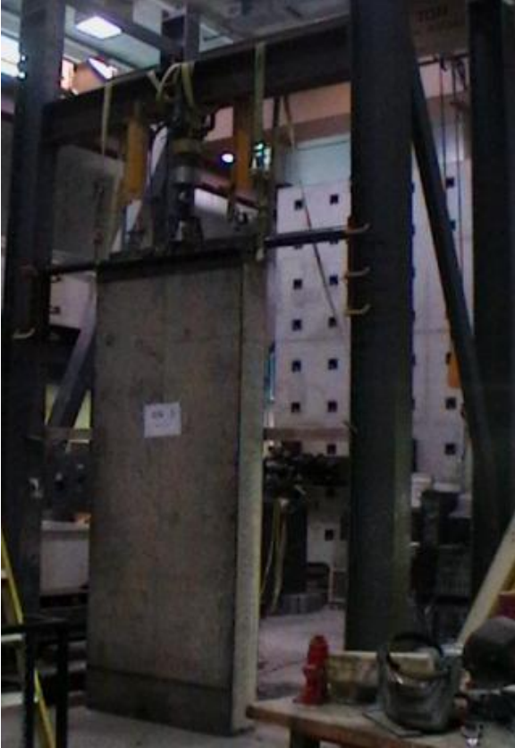
Figure 3.18. Views of the test setup for Axial load Testing
