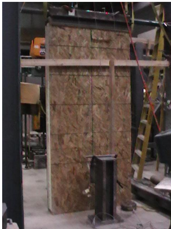
Figure 4.23. View of specimen BW6 after failure due to crushing of OSB face at the top of the wall
