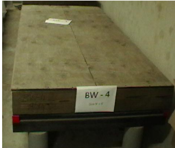
Figure 3.6. View if the SIP panel before applying sustained loading
