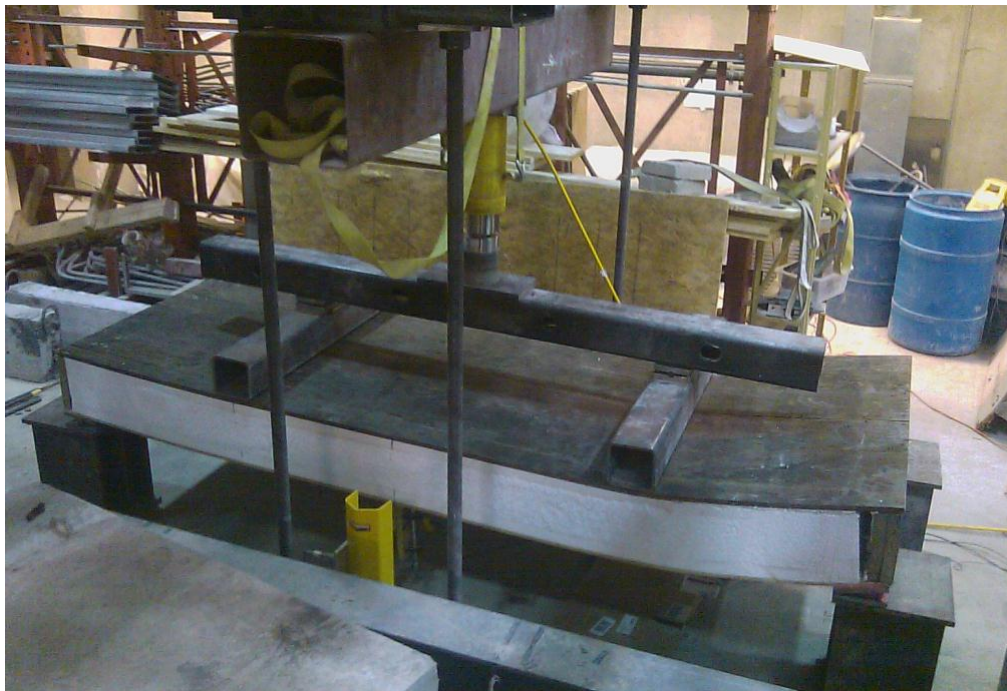
Figure 4.33. View of deformed shape of specimen BW3 after flexural load testing
