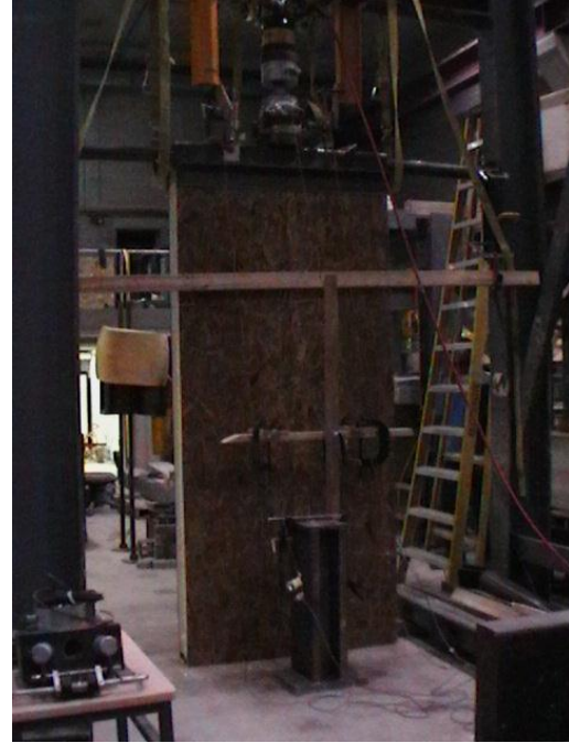
Figure 4.20. Views of the front and back faces of specimen BW5 before axial load testing
