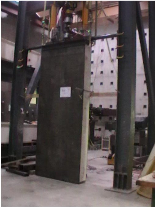
Figure 4.9. Views of front and back faces of specimen BW2 before axial load testing
