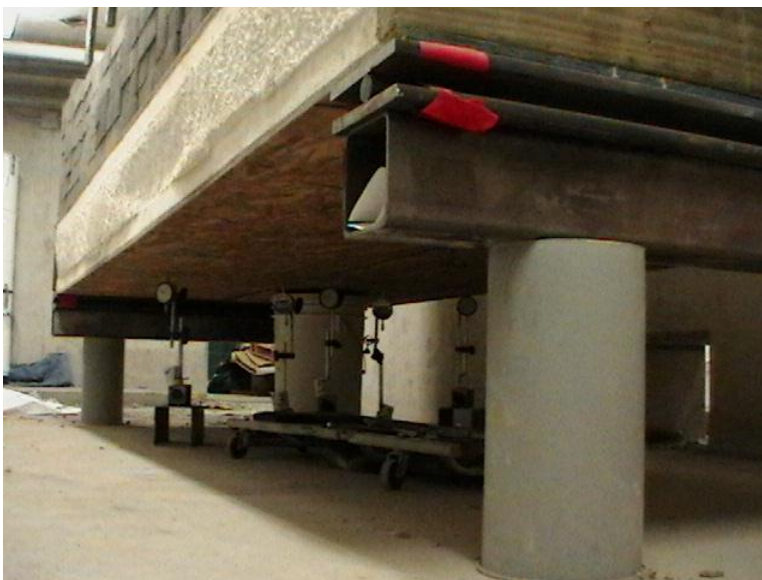
Figure 3.13. View of the dial gauges under the specimen during creep testing
