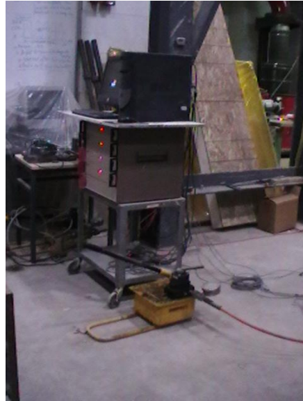
Figure 3.20. View of the data acquisition system and the pump used in the tests
