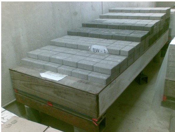
Figure 3.7. Views of specimen BW1 during creep testing
