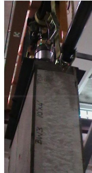
Figure 4.16. Close-up views of specimen BW3 after failure showing crushing of OSB face near the top of the wall
