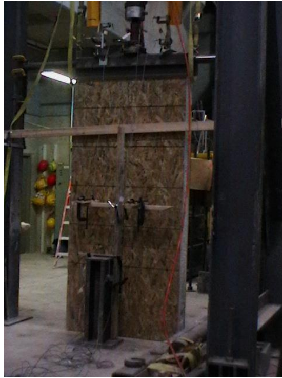
Figure 4.22. View of specimen BW6 before axial load testing
