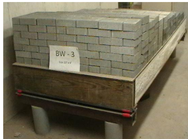
Figure 3.9. Views of specimens BW3 during creep testing
