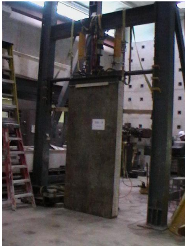
Figure 4.17. View of specimen BW4 before axial load testing
