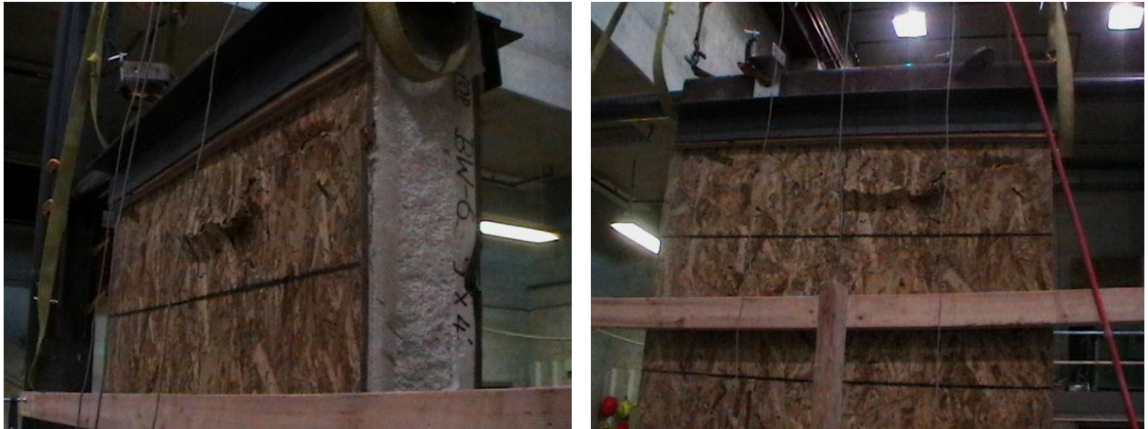
Figure 4.24. Close-up views of specimen BW3 after failure showing crushing of OSB face near the top of the wall
