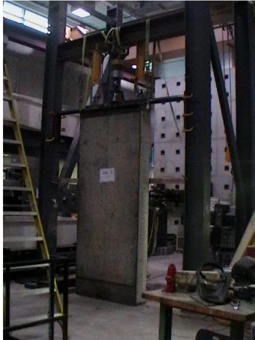
Figure 4.14. View of specimen BW3 before axial load testing
