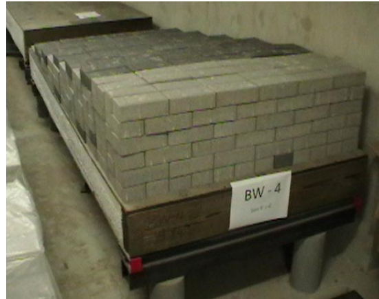
Figure 3.10. Views of specimen BW4 during creep testing
