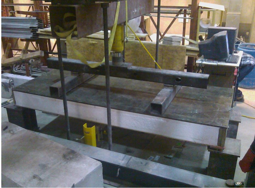
Figure 4.32. View of specimen BW3 before flexural load testing
