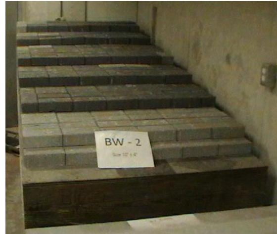
Figure 3.8. Views of specimen BW2 during creep testing
