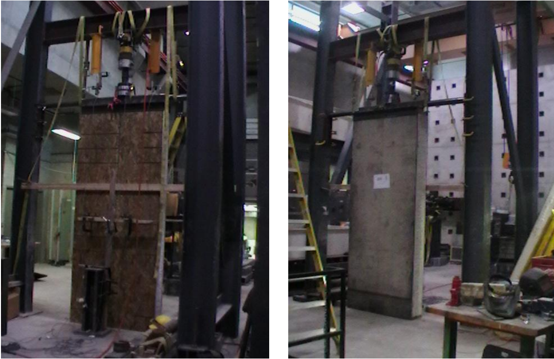
Figure 4.5. View of front and back faces of specimen BW1 before axial load testing
