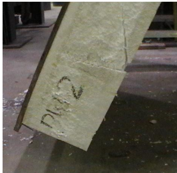
Figure 4.13. Views of fracture of the lumber stud at the connection and diagonal crack of the foam after splitting from the OSB face of specimen BW2
