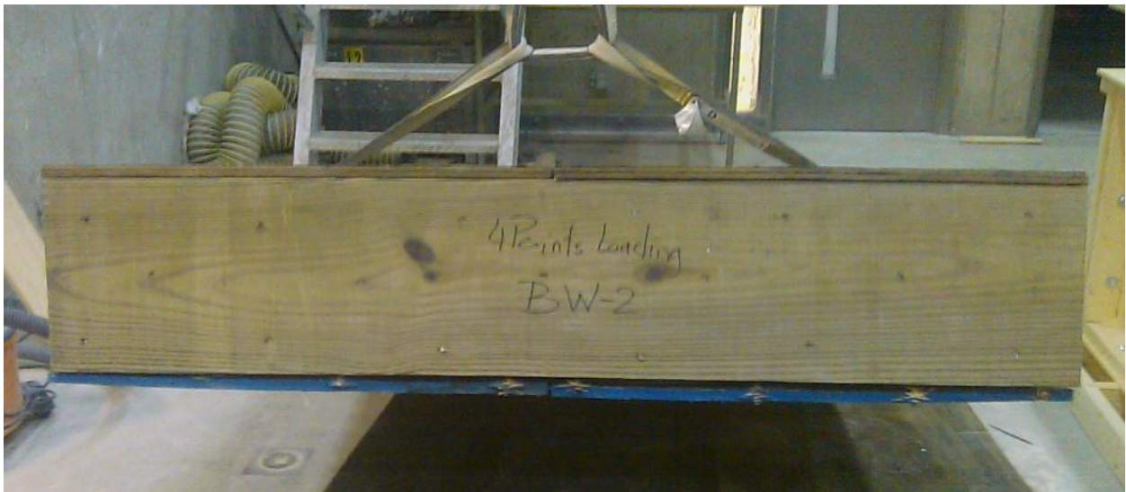
Figure 4.31. View nail tearing failure at the end of OSB face at the support location of specimen BW2 after flexural load testing
