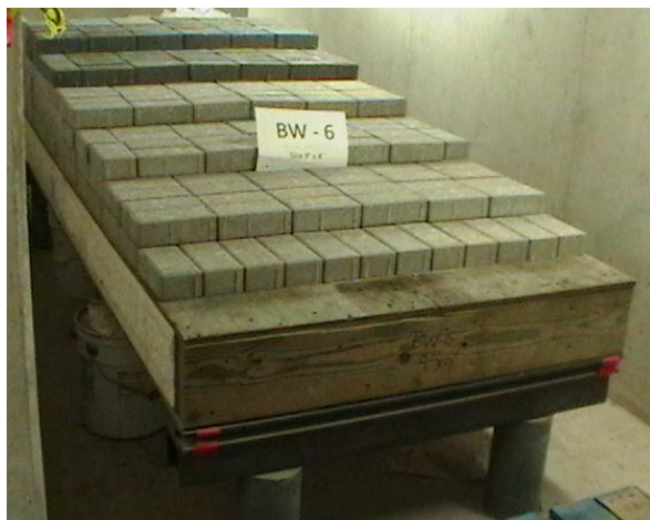
Figure 3.12. View of specimen BW6 during creep testing
