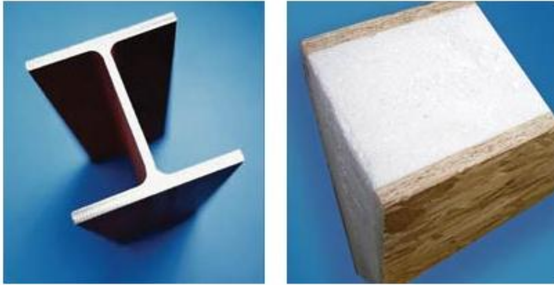
Figure 1.1. Comparison of SIP with I-beam section
