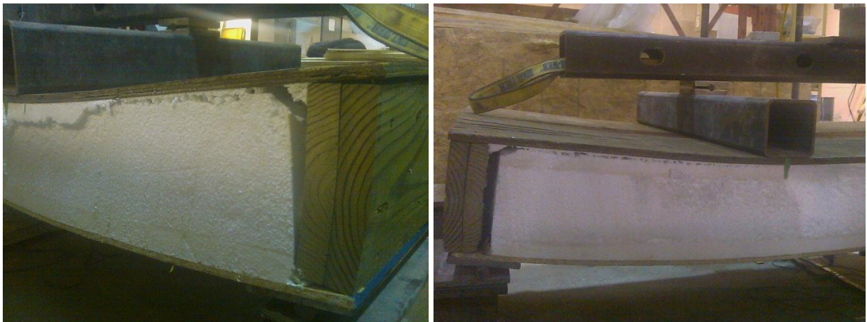
Figure 4.27. Views of shear failure at the interface between the top plywood face and foam core of specimen BW1 after flexural load testing
