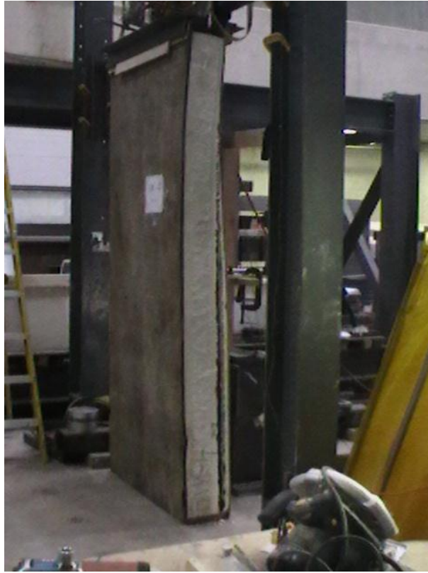
Figure 4.18. View of specimen BW4 after failure showing crushing at the bottom of the OSB face and OSB-foam delamination along the length of the wall
