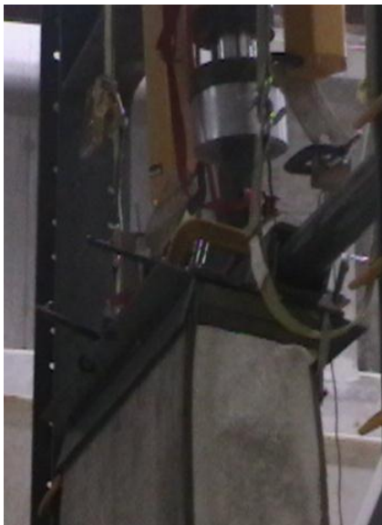
Figure 4.8. Views of top sides of specimen BW1 after failure showing delamination at the OBS-foam interface
