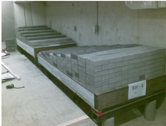
Figure 3.10. Views of specimen BW4 during creep testing
