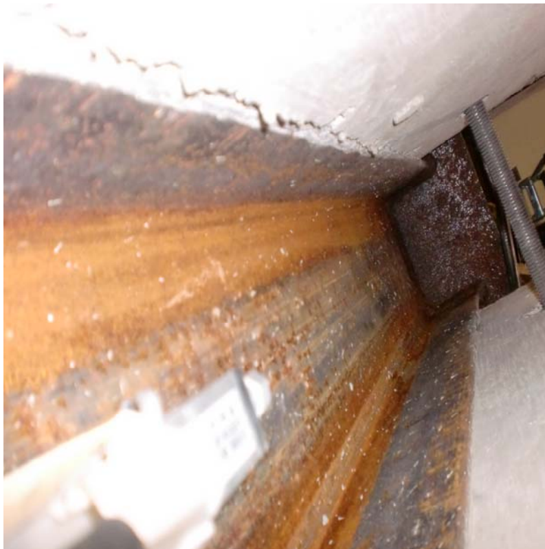
Fig. 4.7 View of the splitting crack at failure along the interface between the concrete slab and the steel flange of specimen PO-2A
