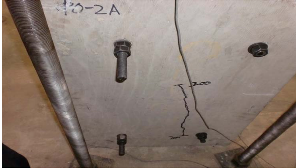
Fig. 4.6 View of the crack pattern at failure on the back side of specimen PO-2A
