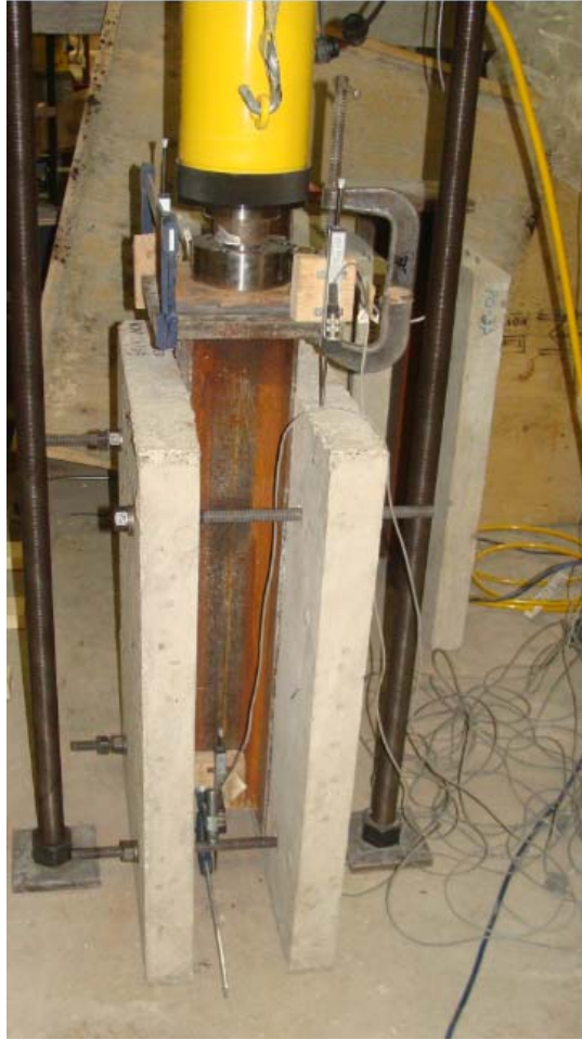
Fig. 3.5 View of LVDT locations in the push-off test
