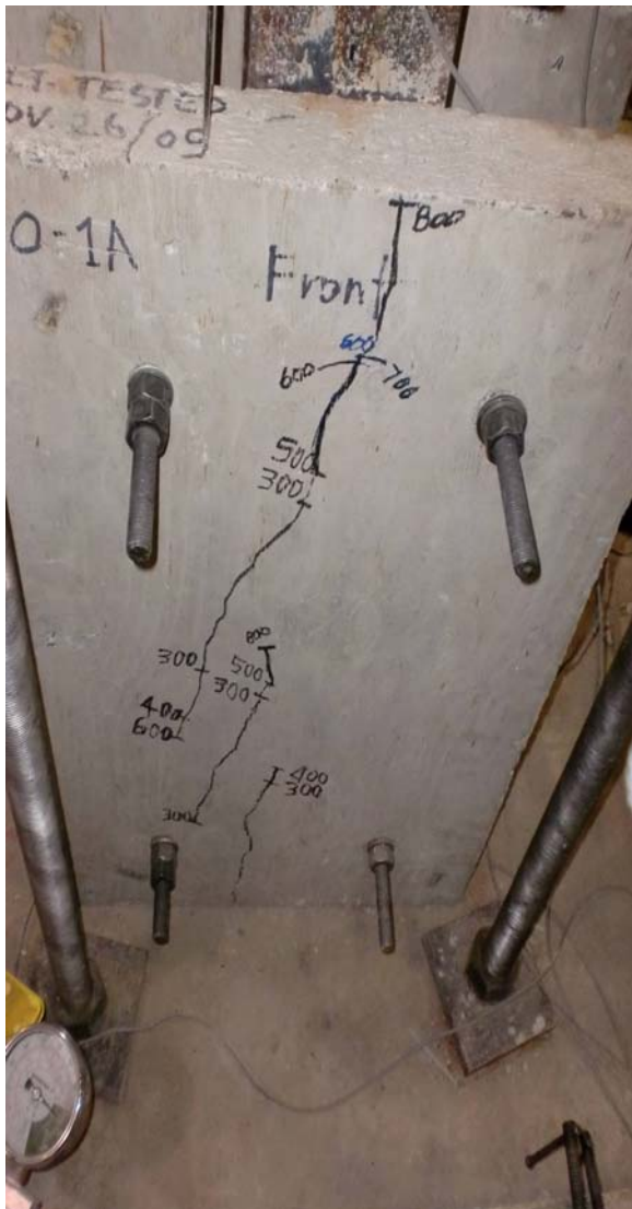
(a) Front side (b) Back side Fig. 4.1 Views of the crack pattern at failure for (a) the front side and (b) the back side of specimen PO-1A
