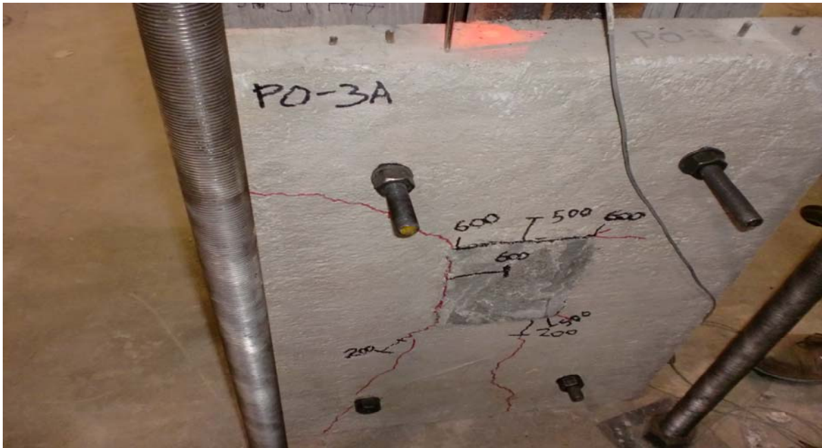
Fig. 4.12 View of the crack pattern at failure on the front side of specimen PO-3A
