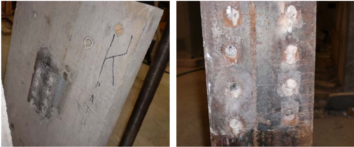
Fig. 4.18 Views of the shear failure of the studs at the slab-shear pocket interface for for specimen PO-3B
