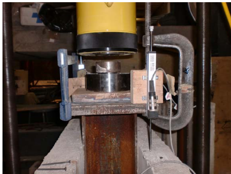
Fig. 3.6 View of LVDT on top of the concrete slab
