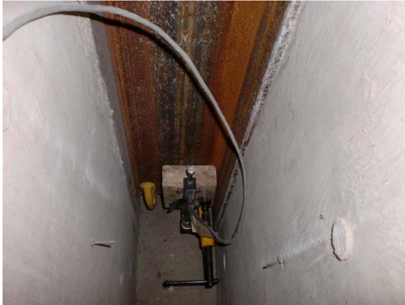
Fig. 3.7 View of LVDT near bottom of steel beam
