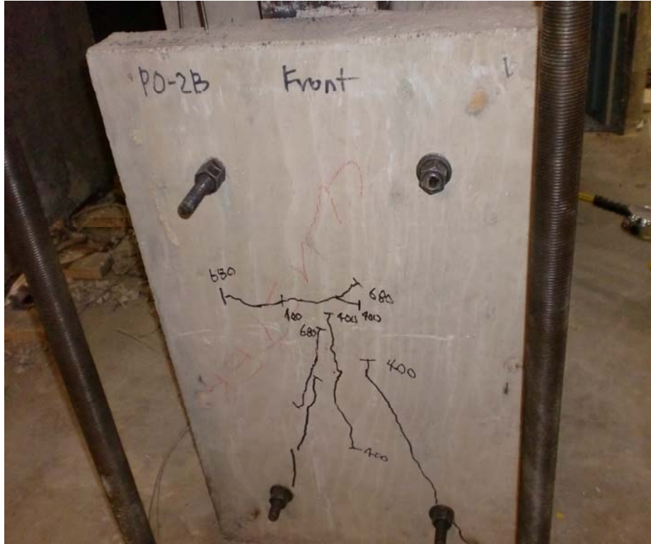
Fig. 4.9 View of the crack pattern at failure on the front side of specimen PO-2B
