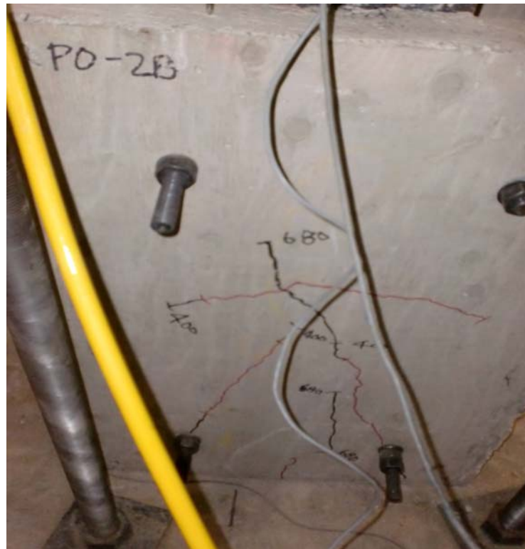
Fig. 4.10 View of the crack pattern at failure on the back side of specimen PO-2B
