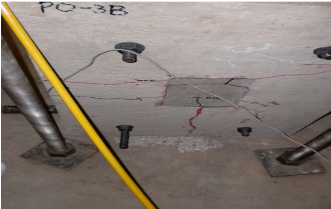
Fig. 4.16 View of the crack pattern at failure on the back side of specimen PO-3B
