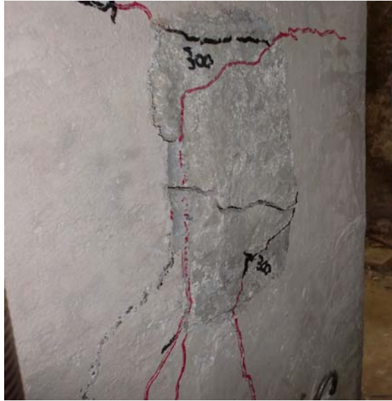
Fig. 4.22 View of the crack pattern at failure on the back side of specimen PO-4B
