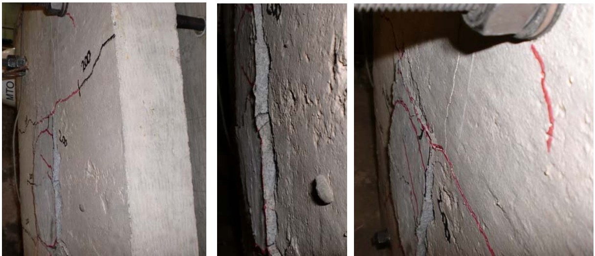
Fig. 4.23 Views of the cracks and pop-out of the shear pocket of specimen PO-4B just before failure
