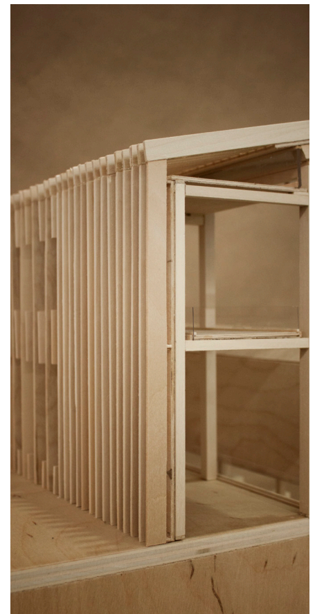
Fig. 49: (bottom right) Detail section model detailing the exterior construction and pattern of the facade
