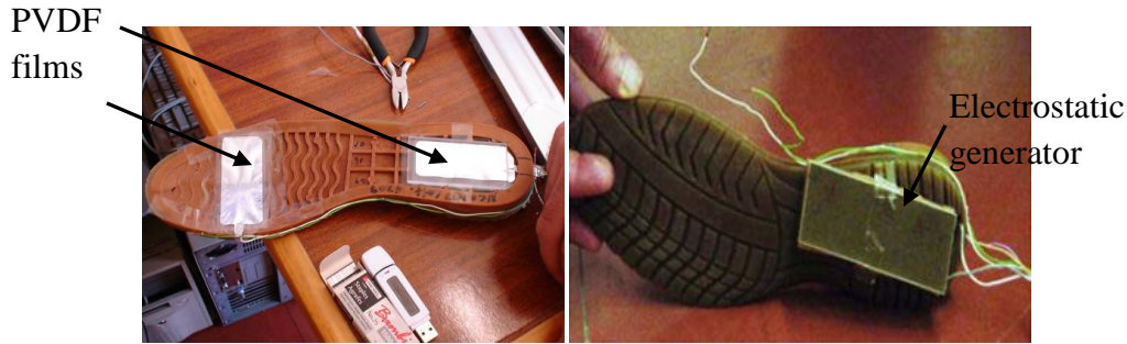
Figure 1.10 Two PVDF films above the shoe sole and an electrostatic generator under the sole [18].
