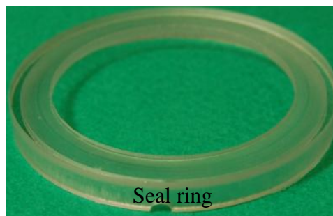
Figure 3.4 The seal ring (Item 6) to keep and seal the rubber bottom surrounding.
