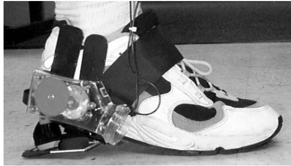
Figure 1.15 A rotary generator system [26].
