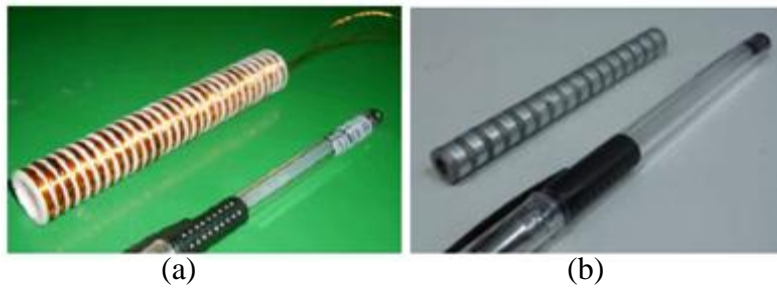
Figure 1.18 Prototype of tubular linear generator. (a) Stator coils, (b) mover magnets [28].
