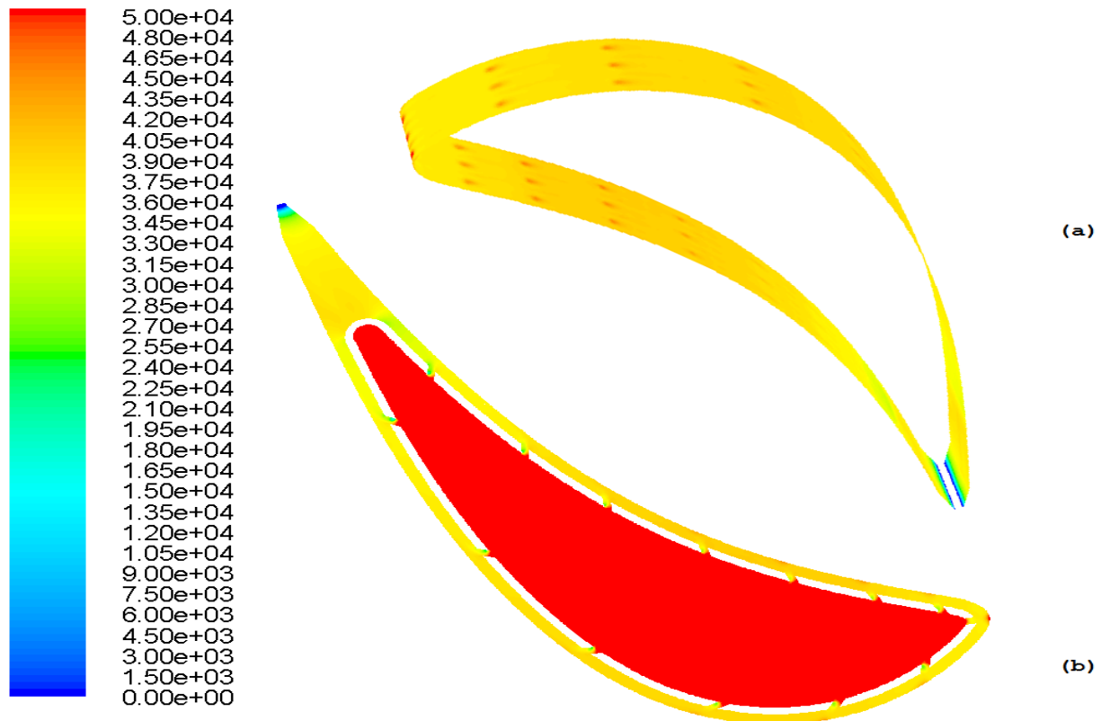
Figure 6-49: Static pressure [Pa] (gauge) for +45° inclination (a) Target surface (b) Column 2
