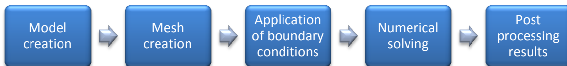
Figure 1-4: Process followed for numerical computation
