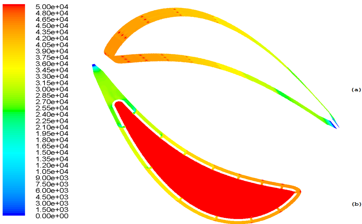
Figure 6-44: Contours of static pressure [Pa] (gauge) for base model (a) Target surface (b) Column 2
