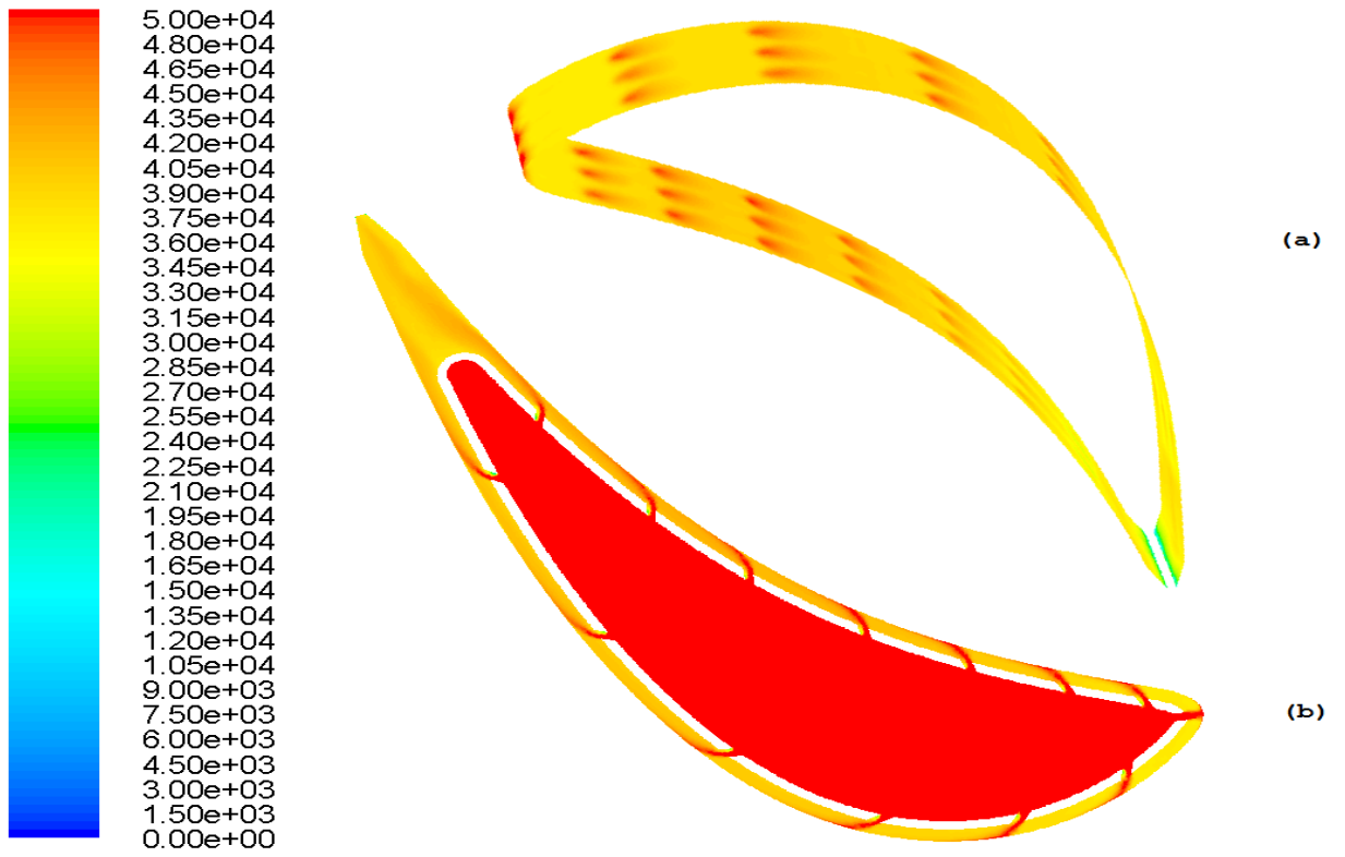
Figure 6-51: Total pressure [Pa] (gauge) for +45° inclination (a) Target surface (b) Column 2
