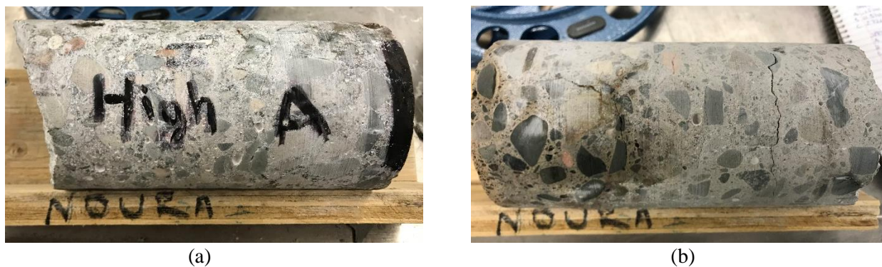
Figure 4.108: (a) High deteriorated and (b) low deteriorated cores after soaking in 0.6 M solution
