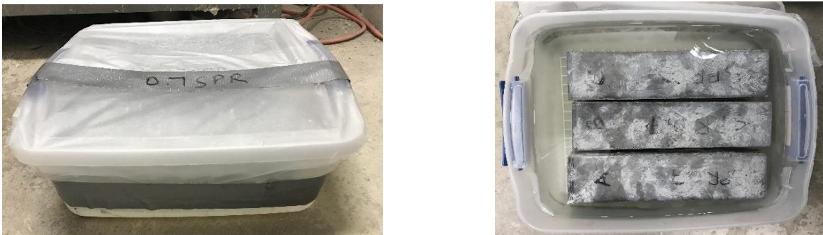
Figure 3.10: Soaking of prisms in plastic containers
