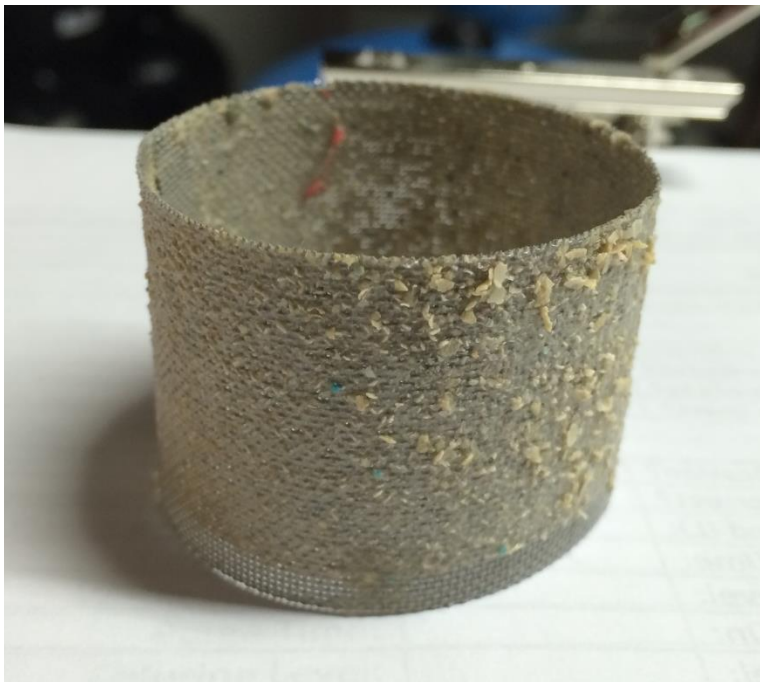
Figure 26: Clogged pump filter from House 22.
