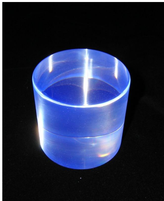
Figure 2.8: Plastic scintillator emitting its characteristic blue light (Eljen Technologies, Sweetwater TX). 49
