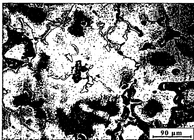
Figure 170: Fully divorced eutectic in the 2.5 cm bar at 5 cm distance from the sprue, 660 °C / 1.3 pcf / with vacuum trial
