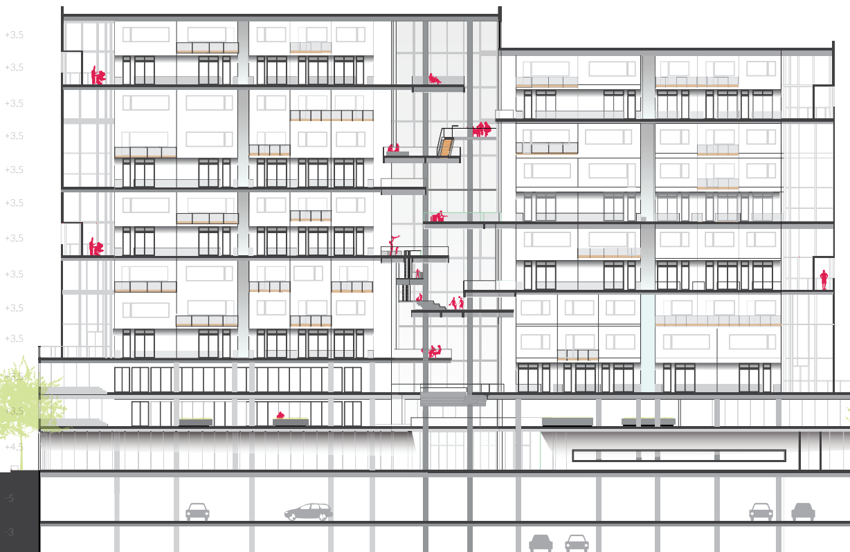
Figure 50: Longitudinal building section illustrating the integration of communal spaces with housing units
