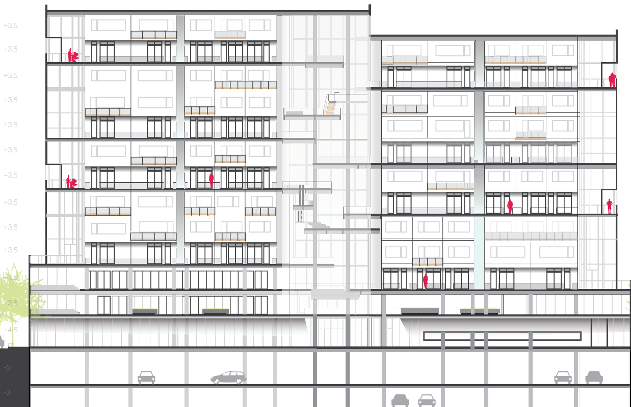
Figure 41: Building section demonstrating that all front doors open on the same level (Scale 1:600) (Below)
