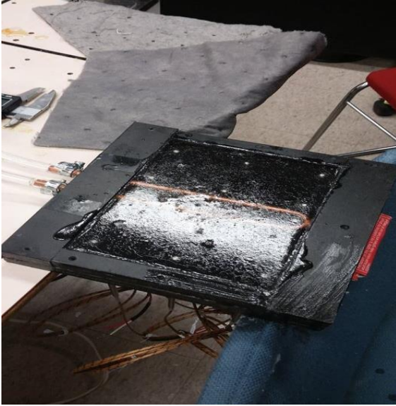
Figure 2.8: Rectangular Cavity with U-shaped tube filled with PCM
