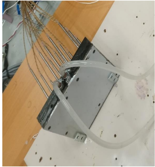
Figure 2.8: Rectangular Cavity with U-shaped tube filled with PCM
